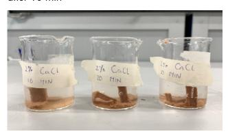
**Figure 103:** 10% CaCL crosslinked AB+SA samples after 10 min
