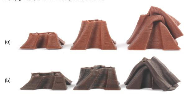
**Figure 96:** Vase shape with converging and diverging overhangs printed with AB, Collapse due to weak spot in the model.
