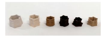
However, it should be noted that these prints did display significant shrinkage, with a 26% reduction in height and a 12% reduction in line width.
