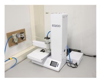
The extrusion pressure was determined seperately for each print since small differences in material and environmental factors were found to influence the necessary pressure for good extrudability. The pressure was adapted until the extruded material showed no signs of under-extrusion or over-extrusion (Figure 35). The extrusion pressure was determined per recipe variation but kept constant during the printing. No fans were used while printing in this phase of the research.
