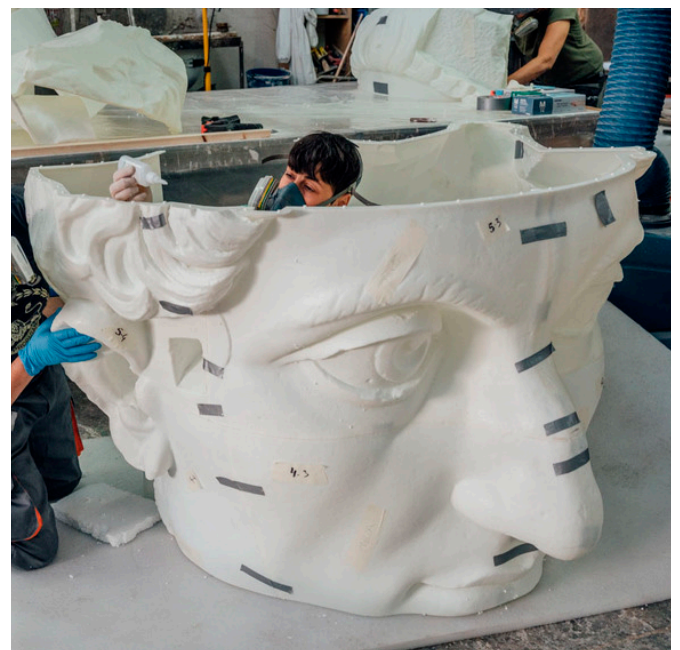
Figure 15. 3D printed moulds being prepared for casting, to recreate the Colossus of Constantine (Factum Foundation, 2024)
