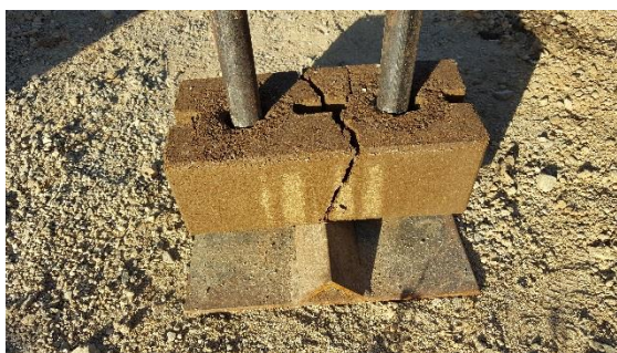
Figure 8: Droptest with a CSEB brick
