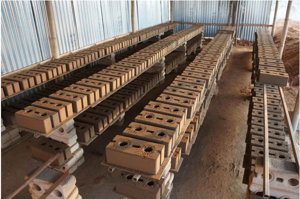
Figure 5: CSEB storage for 24 hours
