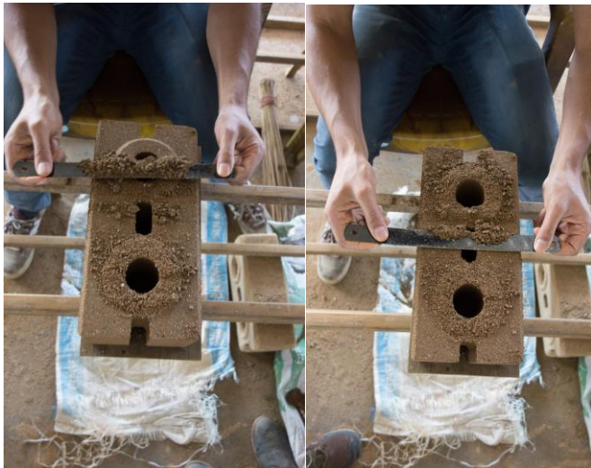
Figure 27: Cutting off the protruding parts
