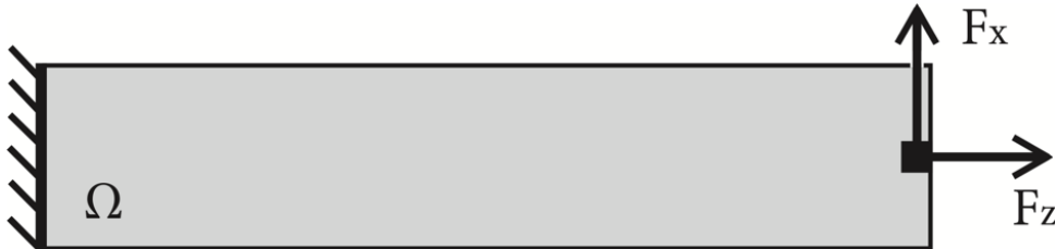
Figure 5.1: Schematic representation of the design domain for a beam
