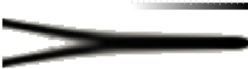
Figure 5.5: Design of beam with objective: maximizing compliance in lateral direction for C_{z \text{ ref}} = 10^{-7} J
