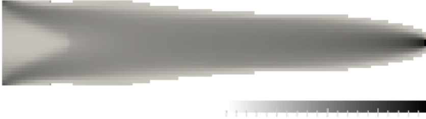
Figure 5.2: Design of beam with objective: maximizing compliance in lateral direction for C_z \text{ ref} = 10^{-6} J
