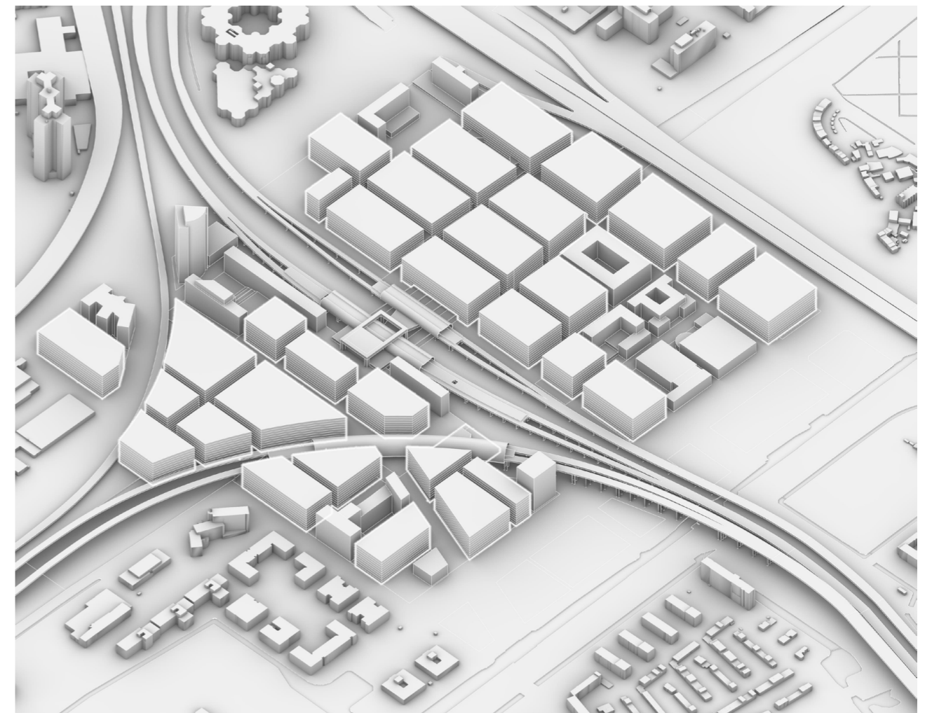
Figure 85. Simplified application of the 50x100m and 100x100m block size combination and the existing fine grain block preservation option that allows for a volumetric visualization of this iteration.
