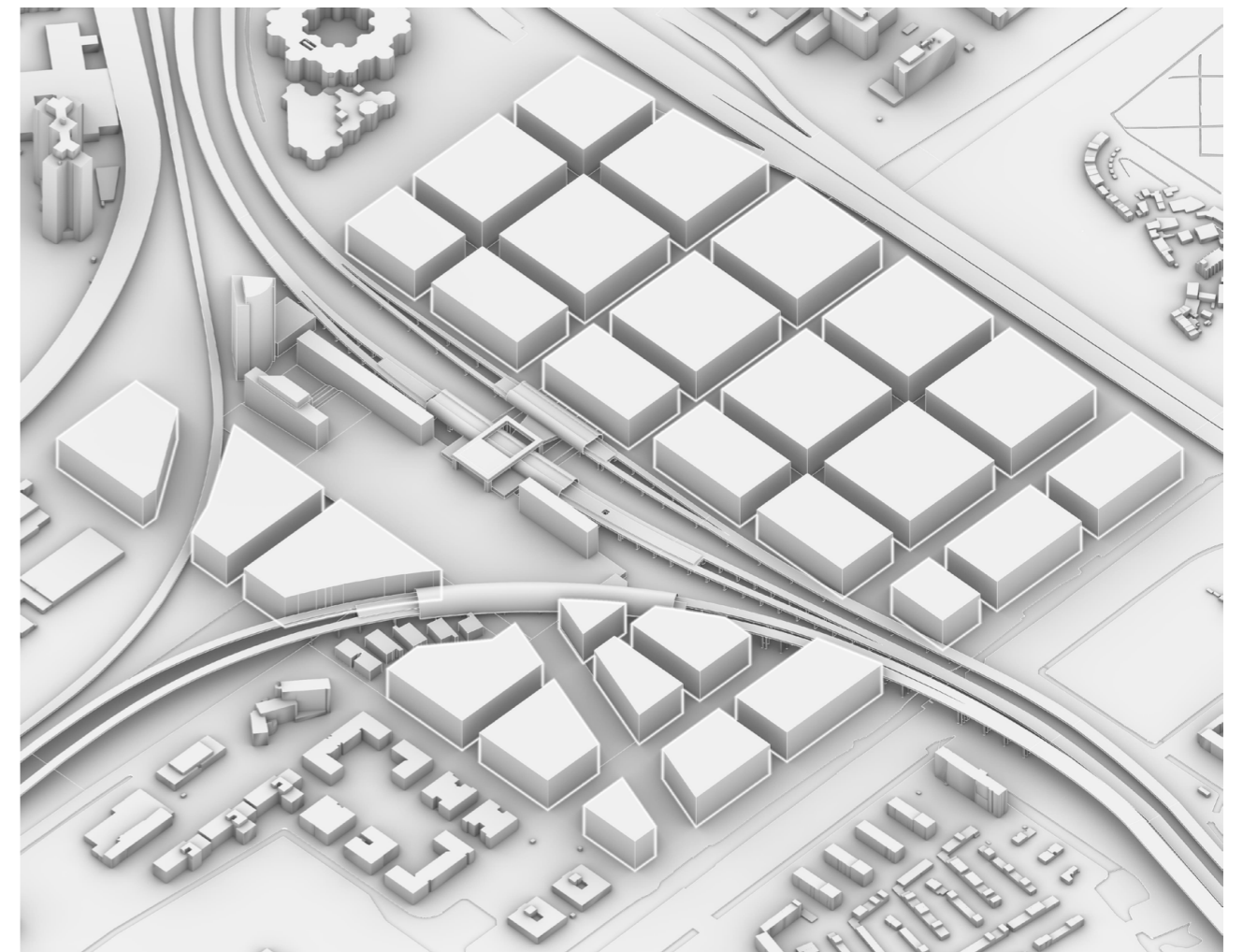
Figure 83. Simplified application of the 100x100m block size that allows for a volumetric visualization of this iteration.
