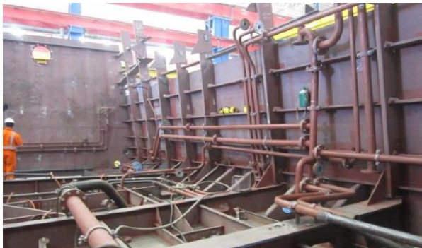
Figure 16: Pre-outfitting work on an open upside down section (Hoekstra, 2014)
