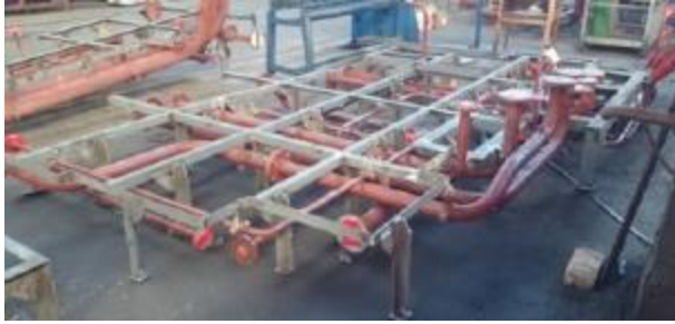
Figure 17: Floor skids after construction in workshop (Reiff, 2016)
