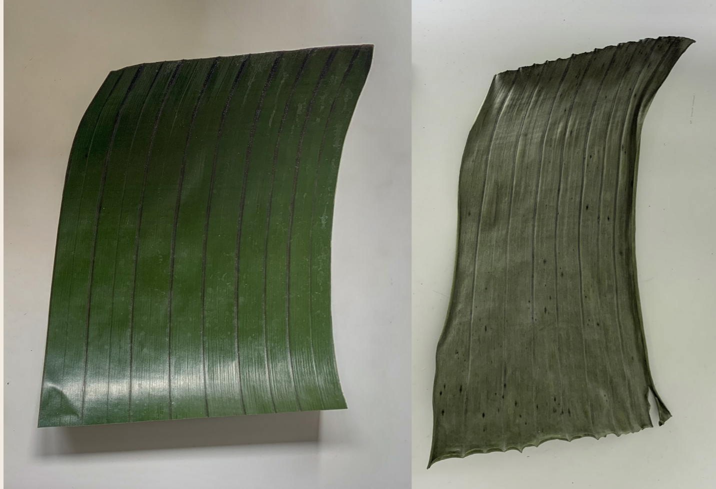
Figure 72 - Shrinkage in leaf after drying
