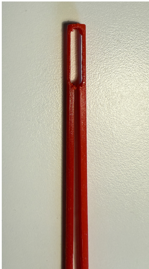
Figure D.1: 3D printed prototype of needle with slot.
