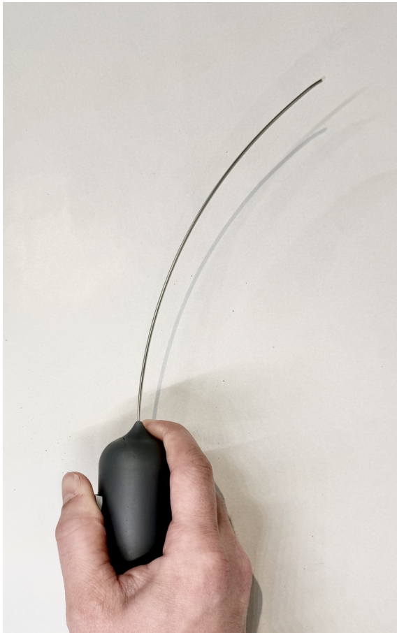
Figure 4.6: Steered configuration of the manually actuated prototype needle housed in a catheter, showing successful lateral deflection upon full actuation during bench testing.
