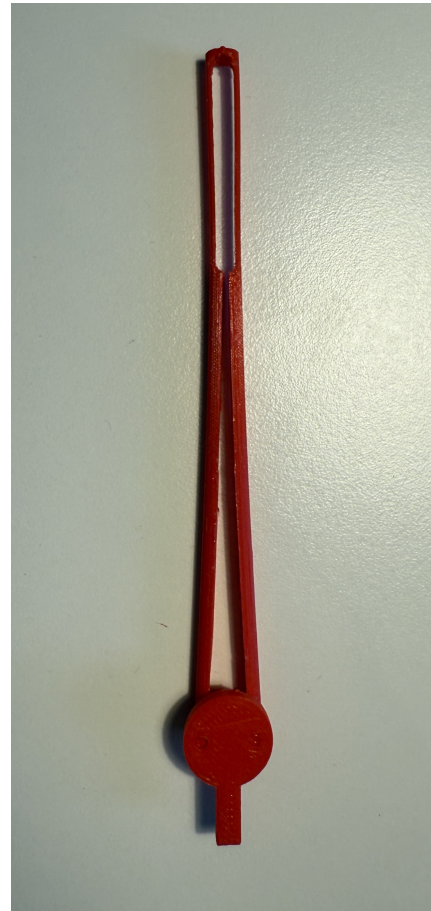
Figure D.4: 3D printed prototype of needle with long sized slot and steering mechanism.
