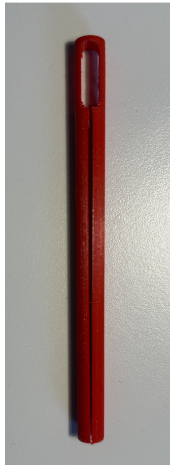
Figure D.2: 3D printed prototype of needle with slot, where the legs are thicker.
