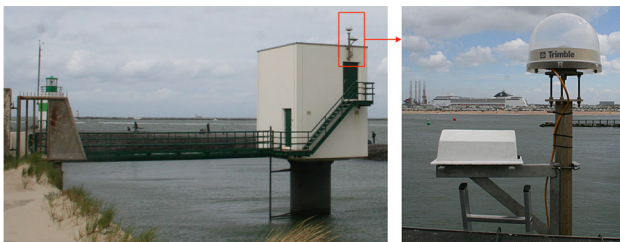
Fig. 1 Example of a collocated transponder-GNSS installation at a tide-gauge in IJmuiden, the Netherlands
