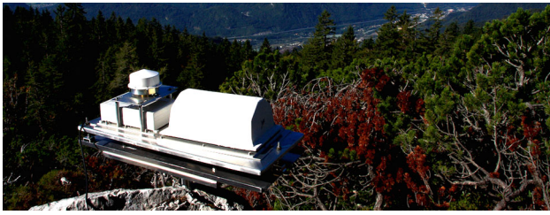
Fig. 13 Example of a collocated transponder-GNSS portable installation [I2GPS (Komac et al. 2012, 2015; Mahapatra 2015)] in the Slovenian Alps
