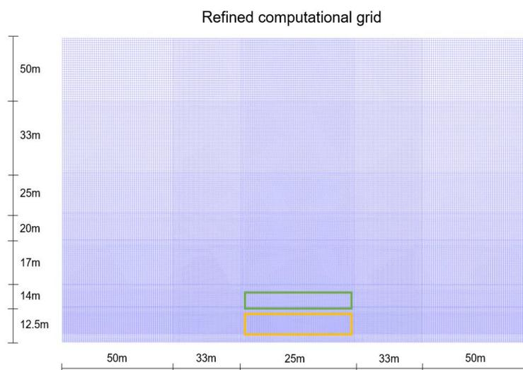
Figure 23: Overview of the computational grid used in XBeach. The grid was built with RGFGRID with a refinement towards the coastline near Domburg. The x – and y-axis represent the dx and dy grid sizes. The yellow and green enclosed zones show the areas where respectively beach and shoreface nourishments are applied.
