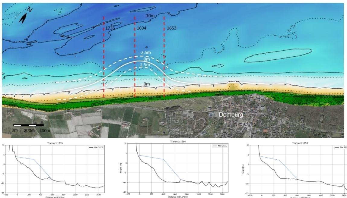
Figure 107: Design of the mega-nourishment, placed to the West of Domburg. The top panel gives a top view of the nourishment with the 2.5m, 0m, and -2.5m contours [white]. The bottom panels provide cross-sections with an indication of the nourished body of sand [dark blue].
