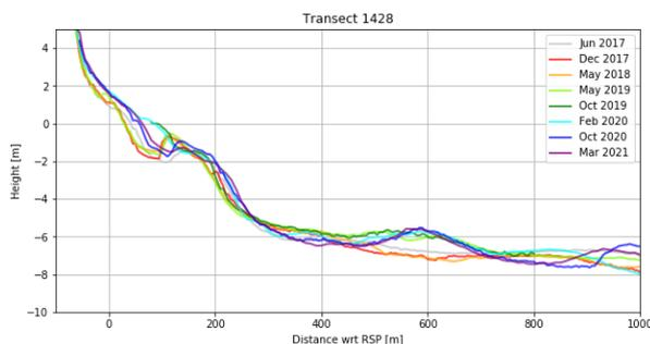
Figure 44: The first transect downstream of the nourished zone shows an emerging shoreface bar after a year.
