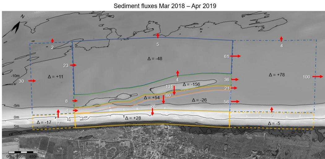
Figure 65: Sediment fluxes and volume changes near Domburg in Mar 2018 – Apr 2019 in  $10^3 \text{ m}^3$  estimated from measurement data. A shoreface nourishment was completed in Dec 2017 in the solid green polygon.
