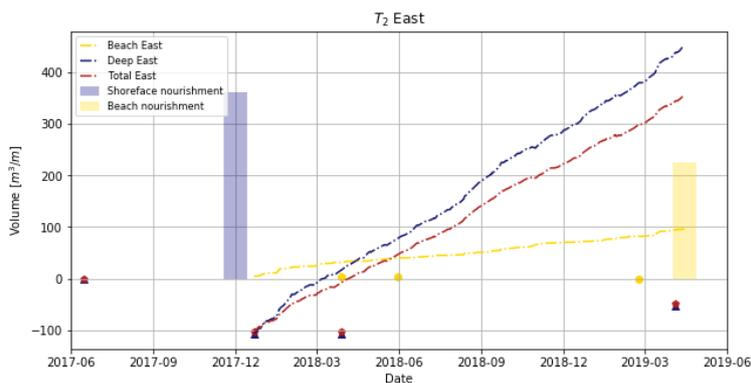
Figure 101: Comparison observed [points] and modelled [dash-dotted lines] volume development of the east coastal zones for  $T_2$ .
