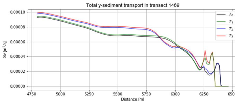
Figure 21: Computed alongshore annual sediment transport from a numerical model. The subtidal zones range between 5400m < x < 6250m, where the sediment transport remains almost constant and starts to decrease at 5800m. The legend portrays the different nourishment scenarios, described in section 3.3.3.
