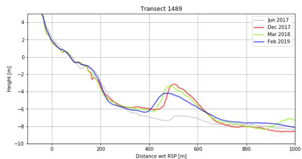
Figure 35: Cross-shore profiles of transect 1489, including the 2017 shoreface nourishment between 400-700m.
