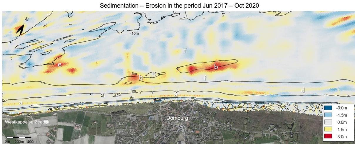
Figure 56: Sedimentation-erosion map between Jun 2017-Oct 2020, showing the morphological changes after a shoreface and beach nourishment. The contour lines are based on the Mar 2018 survey.
