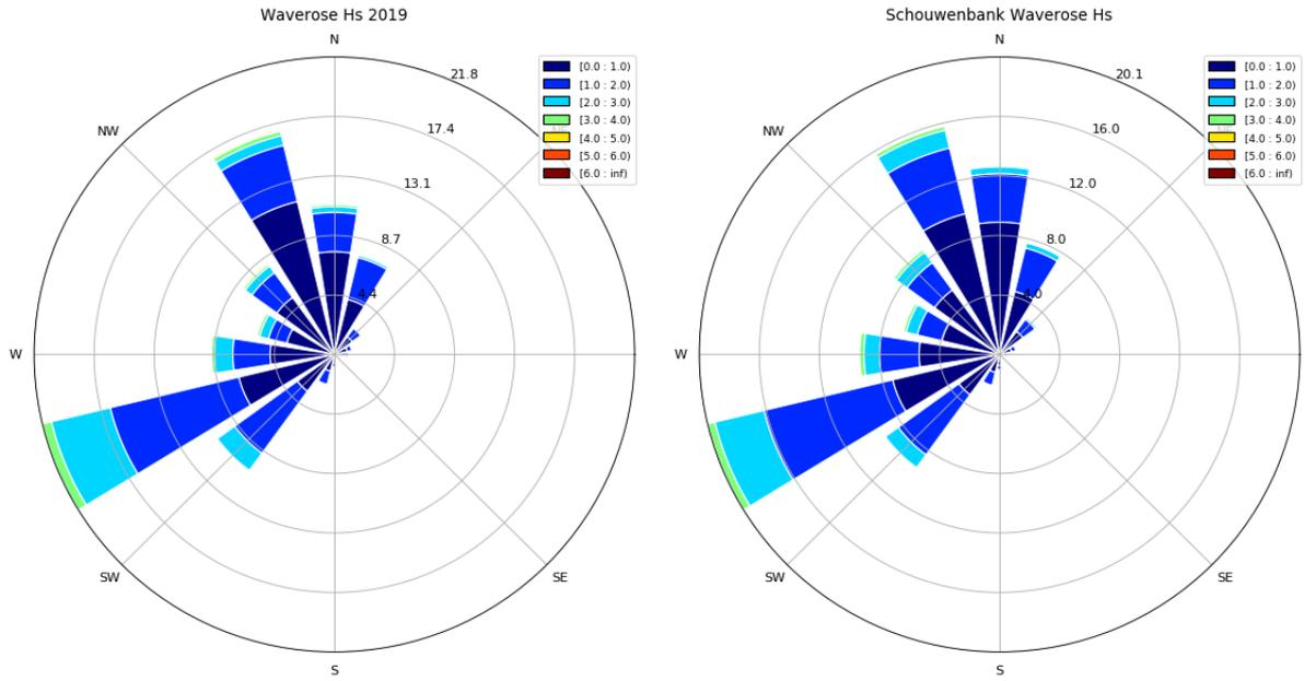
Figure 116: Wave roses after the 2008, 2012, 2014, 2017, 2019 nourishments and the wave rose over the period Jan 2008-Jan 2021. Based on wave data from the Schouwenbank wave buoy [m].
