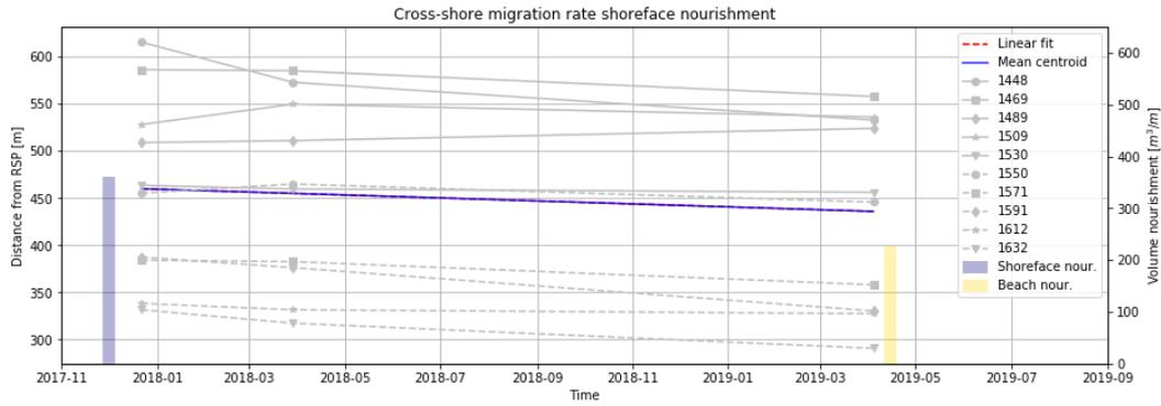
Figure 46: Cross-shore migration of the shoreface nourishment near Domburg based on the position of the centroid of the shoreface bar. The mean migration rate is 18.8 m/year in landward direction. The nourishment volumes are depicted on the secondary y-axis.
