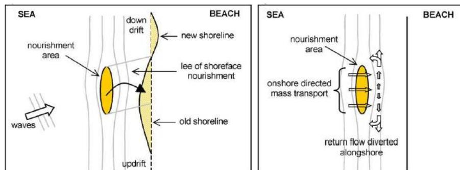
Figure 8: Left panel: Salient effect affecting the alongshore transport rate. Right panel: Feeder-bar affected by both cross- and alongshore processes. (From: van Duin et al., 2004)
