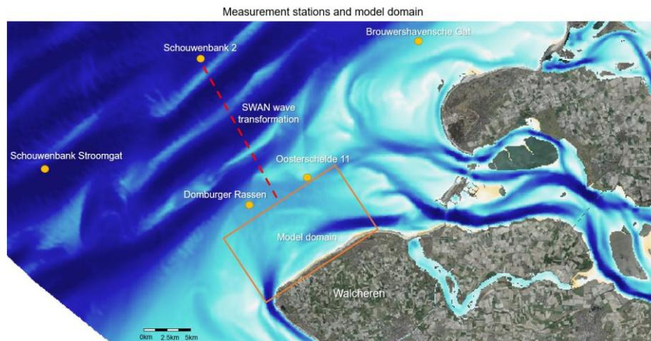
Figure 15: Overview of the measurement stations [yellow], XBeach model domain [orange] and the transect used for wave transformations in SWAN [red dashed].
