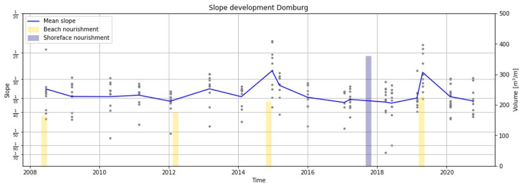
Figure 52: Slope of the coastal profile between NAP+3m and NAP-3m of transects 1448-1632. The nourishment volumes are depicted on the secondary y-axis.
