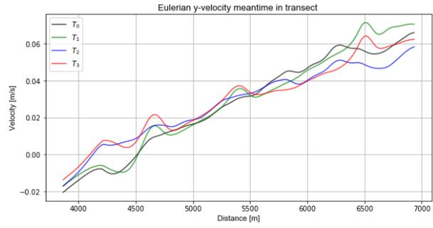
Figure 88: Mean alongshore current for wave condition c2:  $H_s=0.64m$ ,  $\Theta=342^\circ$ ,  $T_p=5.8s$  in the zone from the dune foot to 1000m offshore.
