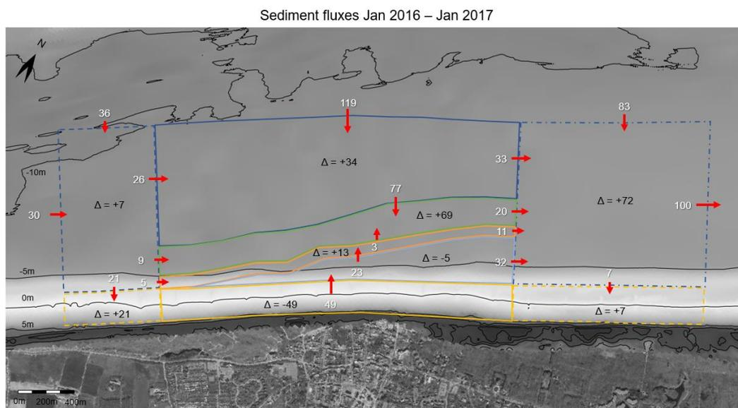
Figure 63: Sediment fluxes and volume changes near Domburg in Jan 2016 - Jan 2017 in 10<sup>3</sup> m<sup>3</sup> estimated from measurement data. The sediment fluxes are represented by red arrows and the volume change for the individual polygons are given by the black deltas. A beach nourishment was completed in Dec 2014 in the yellow solid polygon.
