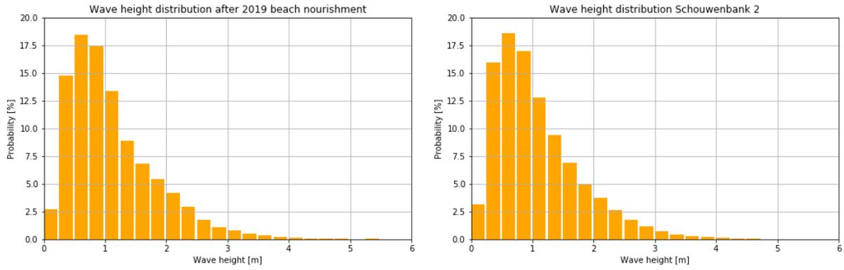
Figure 117: Wave height distribution between the 2008, 2012, 2014, 2017, 2019 nourishments and the general wave height distribution over the period Jan 2008-Jan 2021. Based on wave data from the Schouwenbank wave buoy.
