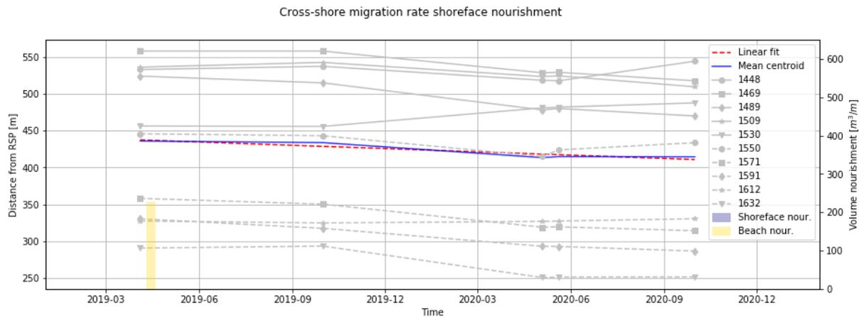
Figure 49: Cross-shore migration of the shoreface nourishment near Domburg posterior to the 2019 beach nourishment, based on the position of the centroid of the sandbar. The mean migration rate is 17.8 m/year in landward direction. The nourishment volumes are depicted on the secondary y-axis.
