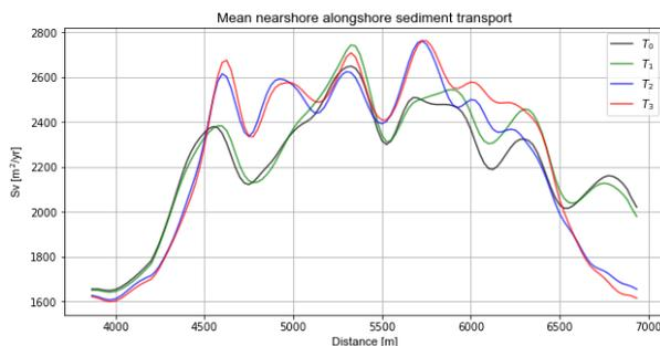
Figure 93: Mean alongshore sediment transport for wave condition c1:  $H_s=0.62\text{m}$ ,  $\Theta=267^\circ$ ,  $T_p=4.7\text{s}$  in the zone from the dune foot to 1000m offshore.
