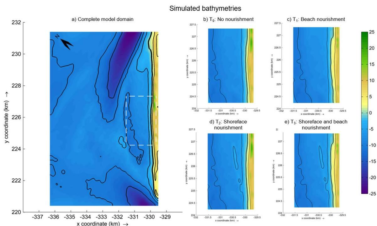
Figure 24: Overview of the simulated bathymetries with 5m contours and the thick solid line represents the 0m line. a) Complete bathymetry of the model domain. The white dashed line represents the area of interest near Domburg where nourishments are applied. b)  $T_0$ : No nourishment. c)  $T_1$ : Beach nourishment. d)  $T_2$ : Shoreface nourishment. e)  $T_3$ : Shoreface and beach nourishment.
