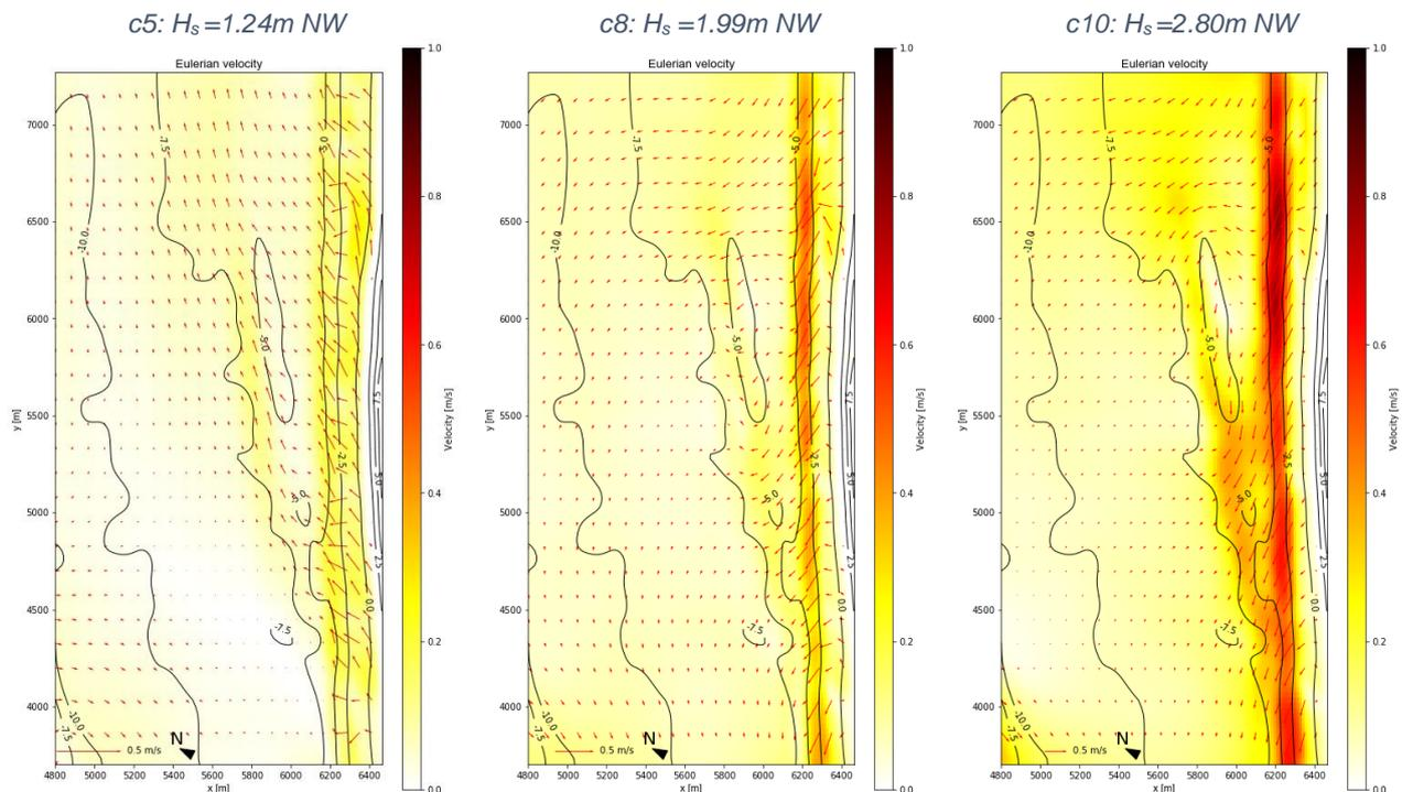
Figure 80: Currents under normally incident ( $328-335^\circ$ ) wave conditions around a shoreface nourishment (T2).
