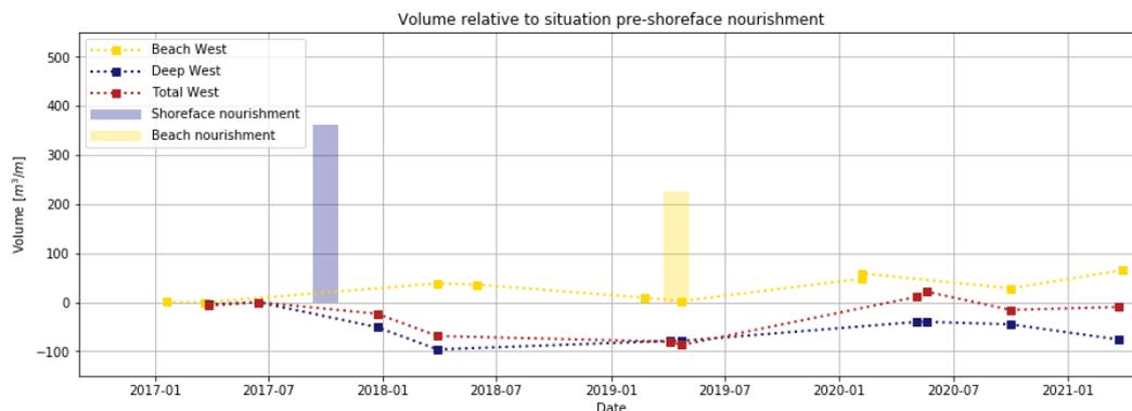
Figure 60: The volume change of coastal zones in transects 1694-1653, to the west of Domburg. No nourishment was placed on these transects, but upstream and downstream a shoreface nourishment and beach nourishment were constructed simultaneously.
