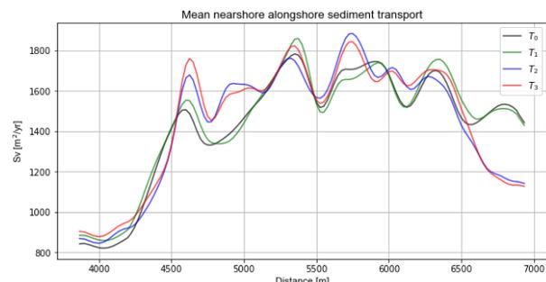
Figure 94: Mean alongshore sediment transport for wave condition c2:  $H_s=0.64\text{m}$ ,  $\Theta=342^\circ$ ,  $T_p=5.8\text{s}$  in the zone from the dune foot to 1000m offshore.
