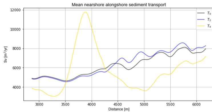
Figure 114: Mean alongshore sediment transport for wave condition c7:  $H_s=1.76m$ ,  $\Theta=272^\circ$ ,  $T_p=6.5s$  in the zone from the dune foot to 1000m offshore. The coast without nourishment ( $T_0$ ), with a shoreface nourishment ( $T_2$ ) and a mega-nourishment ( $T_4$ ) are displayed.
