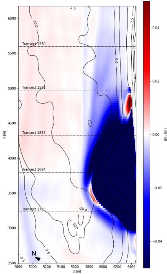
Figure 108: Difference in wave height between  $T_0$  and  $T_4$
