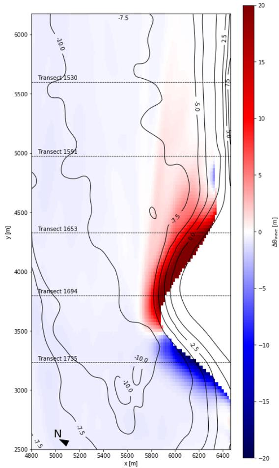
Figure 110: Difference in wave direction between  $T_0$  and  $T_4$
