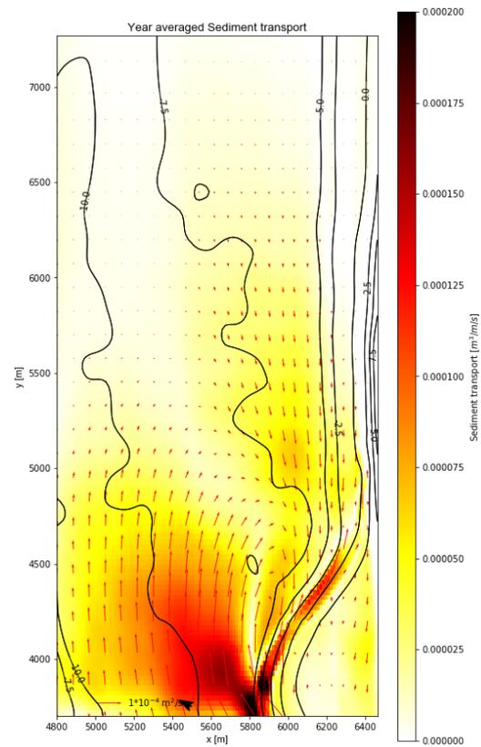
Figure 127: Year-averaged sediment transport for  $T_4 - T_0$
