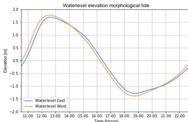
Figure 28: The water level elevations at the west and east model boundaries that represent best the bed level development during a complete tidal cycle. The signal's tidal range is a factor 1.2 larger than the mean tidal range at Walcheren.
