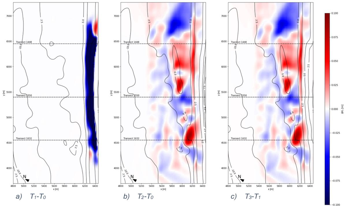
Figure 77: Annual significant wave height changes for the presence of a nourishment. The effect on the wave height due to a) beach nourishment:  $T_1 - T_0$ . b) shoreface nourishment:  $T_2 - T_0$ . c) combined beach and shoreface nourishment to only a beach nourishment:  $T_3 - T_1$ .
