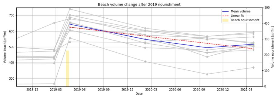
Figure 68: Beach volume change after the combined 2017 shoreface and 2019 beach nourishment. An average erosion rate of  $-70.8\text{m}^3/\text{m}/\text{yr}$  and a lifetime of 3.2 years is estimated based on four surveys in the two years post-construction.
