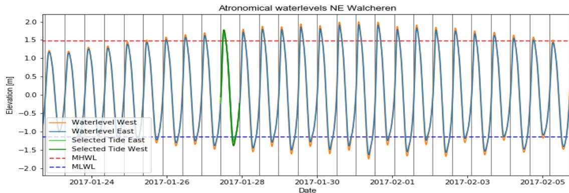
Figure 27: Spring-neap tidal cycle at the west and east model boundaries the mean low and high-water levels indicated.
