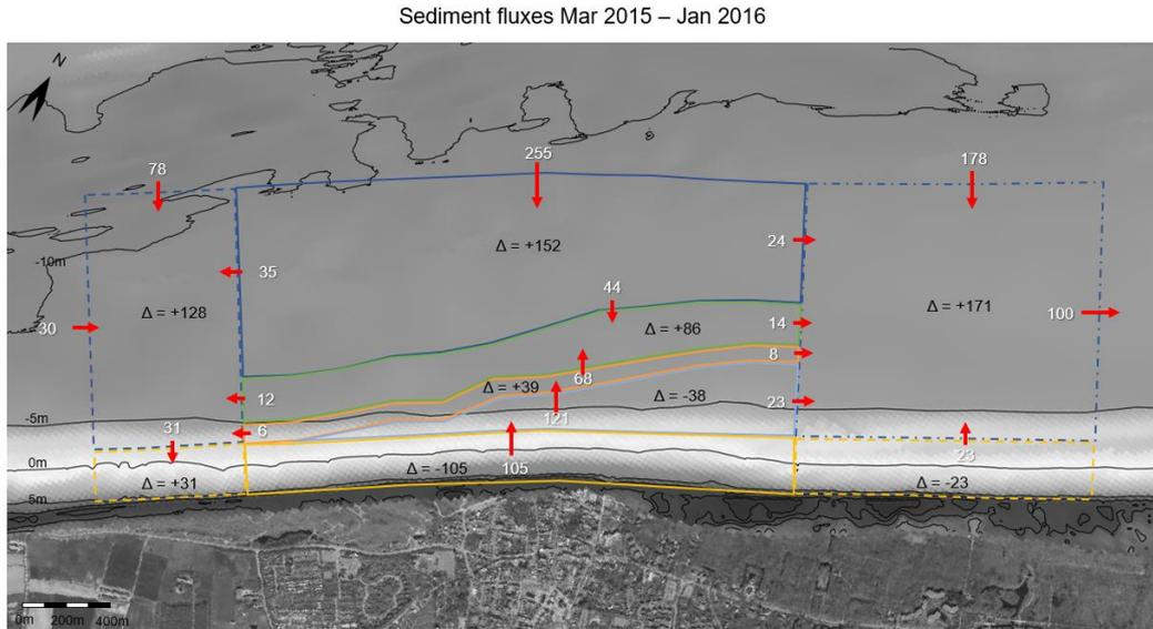
Figure 64: Sediment fluxes and volume changes near Domburg in Mar 2015 - Jan 2016 in  $10^3 \text{ m}^3$  estimated from measurement data. A beach nourishment was completed in Dec 2014 in the yellow solid polygon.
