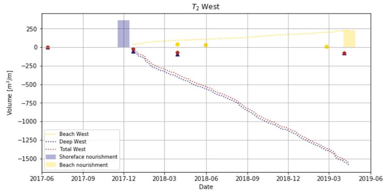
Figure 99: Comparison observed [points] and modelled [dotted lines] volume development west coastal zones for  $T_2$ .
