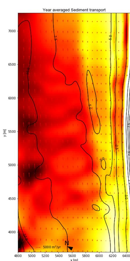
Figure 97: The year averaged sediment transport with a shoreface nourishment,  $T_2$ .
