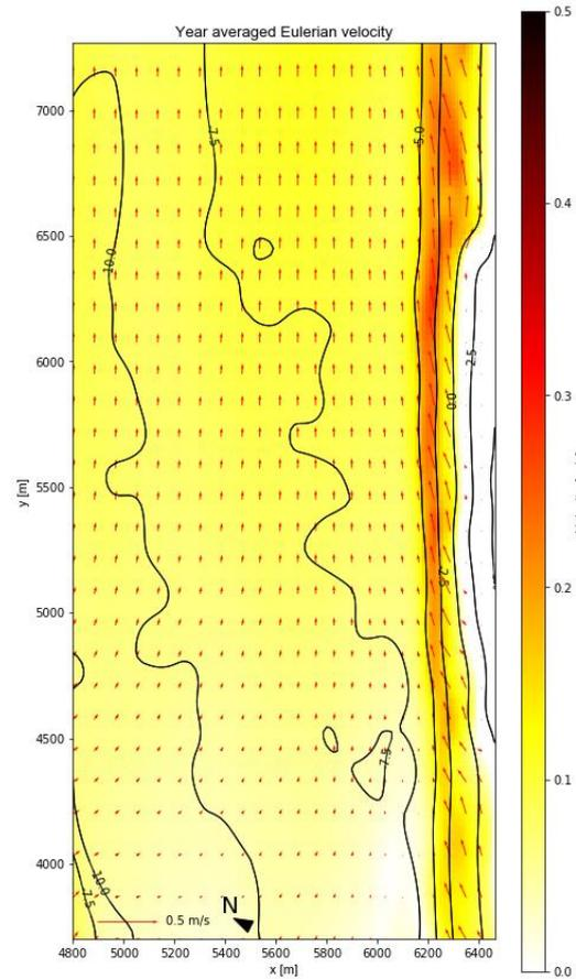
Figure 82: The year averaged Eulerian velocity for  $T_1$ , with a beach nourishment.
