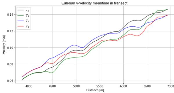
Figure 87: Mean alongshore current for wave condition c1:  $H_s=0.62m$ ,  $\Theta=267^\circ$ ,  $T_p=4.7s$  in the zone from the dune foot to 1000m offshore.
