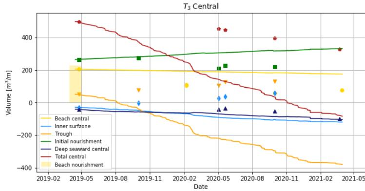
Figure 103: Comparison observed and modelled volume development central coastal zones for  $T_3$ .
