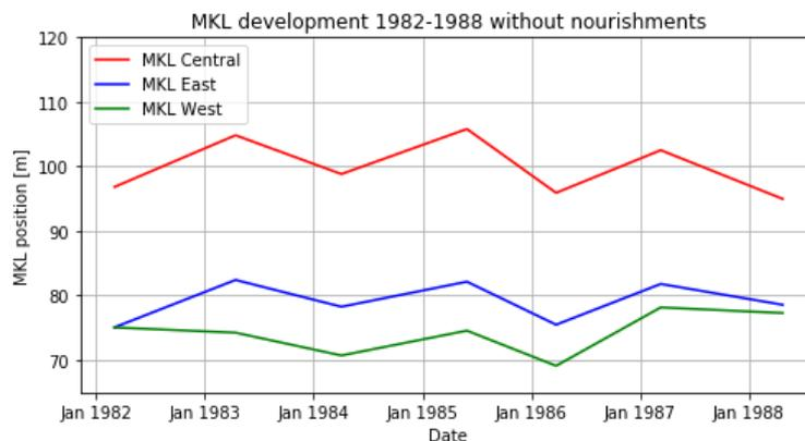
Figure 70: Average momentary coastline development in the period 1982-1988, before large scale sand nourishments were applied. The average MKL development of the central transects 1632-1448 is given in [red]. The adjacent coastlines, transects 1428-1306 to the east and 1694-1653 to the west are portrayed in [blue] and [green] respectively.
