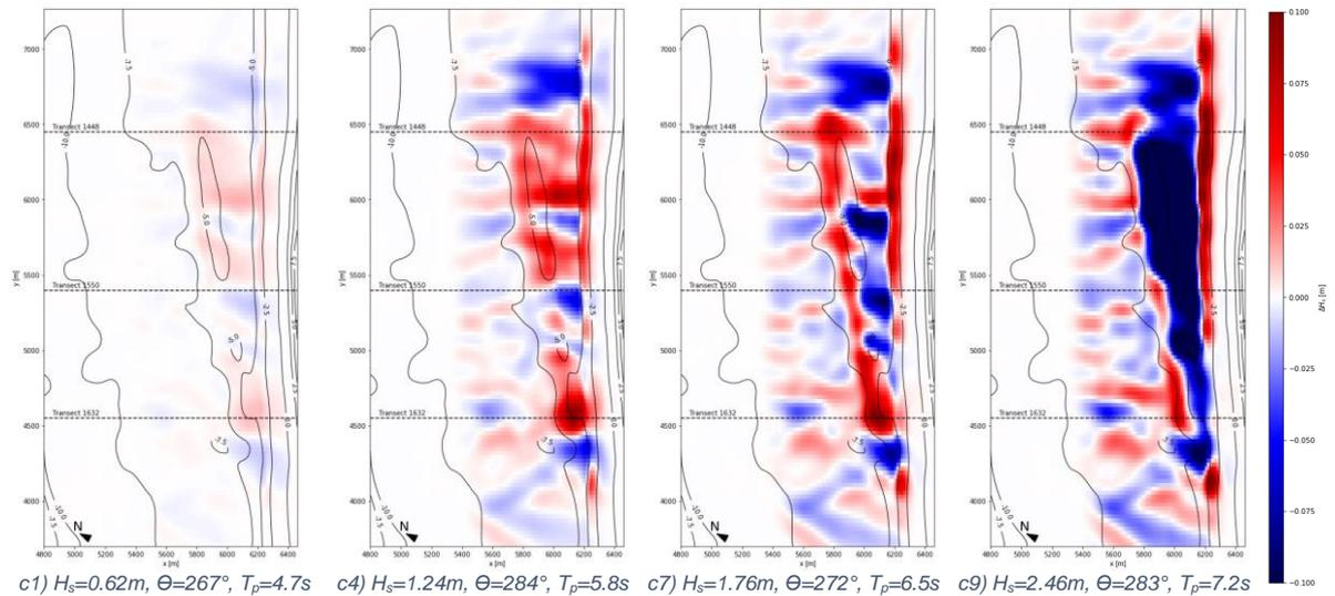
Figure 75: Difference in wave height for  $T_2-T_0$  for four obliquely incident wave classes to examine the effect of a shore parallel bar.
