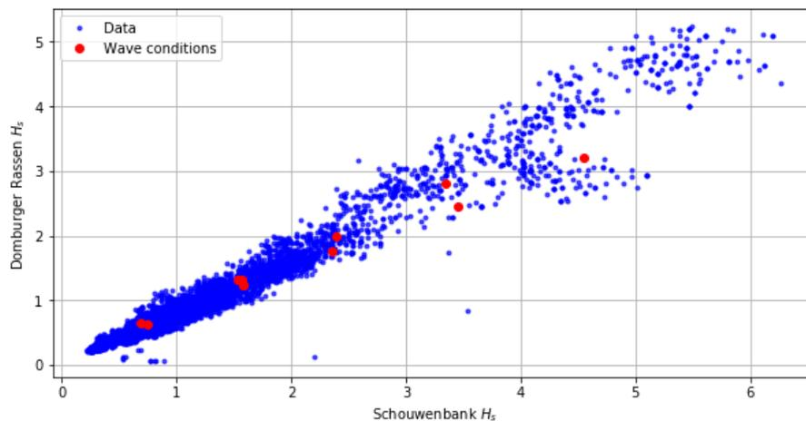
Figure 29: Significant wave height of the Schouwenbank 2 Wave buoy and the Domburger Rassen [Blue] compared to the transformed wave conditions from SWAN [Red].
