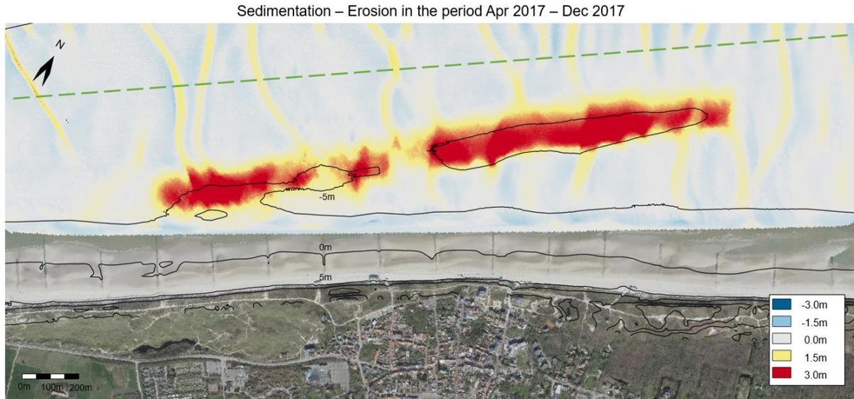
Figure 57: Sedimentation-erosion map between the in- and outsurvey, measured with multibeam, of the 2017 shoreface nourishment. The contour lines are based on the 2018 spring survey. The red area represents the nourished area. The dashed green transect shows the location of the cross-section of Figure 58.
