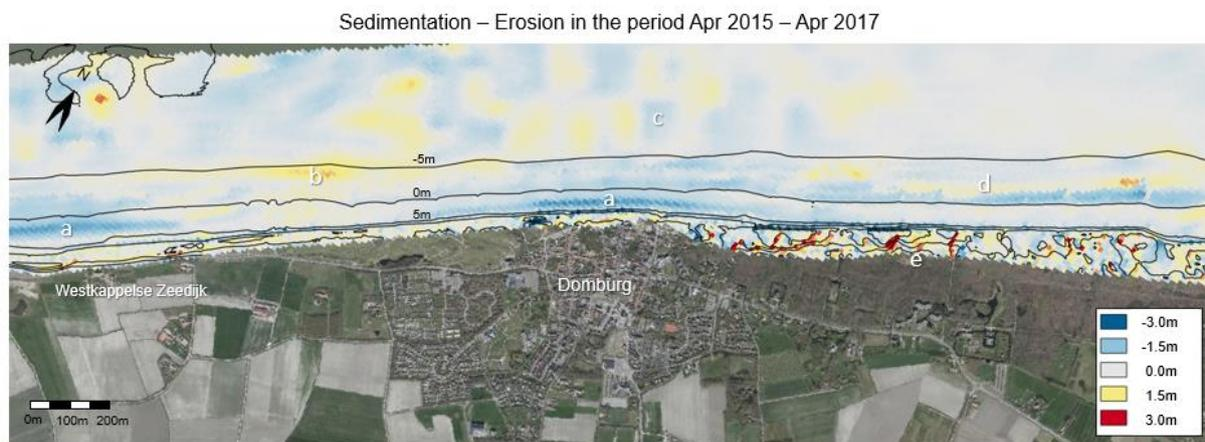
Figure 53: Sedimentation-erosion map between Apr 2015-Apr 2017, showing the morphological changes after a beach nourishment completed in Dec 2014. The contour lines are based on the Apr 2017 survey.
