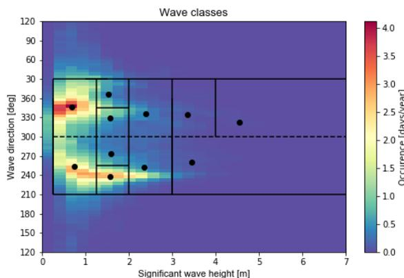
Figure 25: Wave climate at the Schouwenbank. The selected wave conditions, averaged per black square, are represented by black dots.
