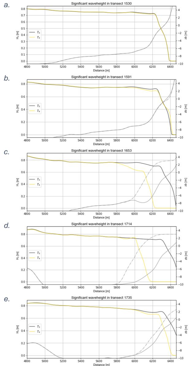
Figure 109: Year-averaged wave heights for  $T_0$  and  $T_4$  for transects a. 1530, b. 1591, c. 1653, d. 1694, e. 1735.
