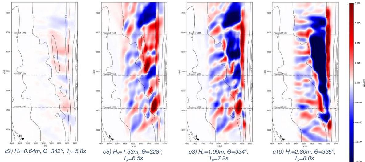
Figure 74: Difference in wave height for  $T_2-T_0$  for four near-normally incident wave classes to examine the effect of a shore parallel bar. The shore normal is at  $330^\circ$  and the depth contours are given with 2.5m intervals.
