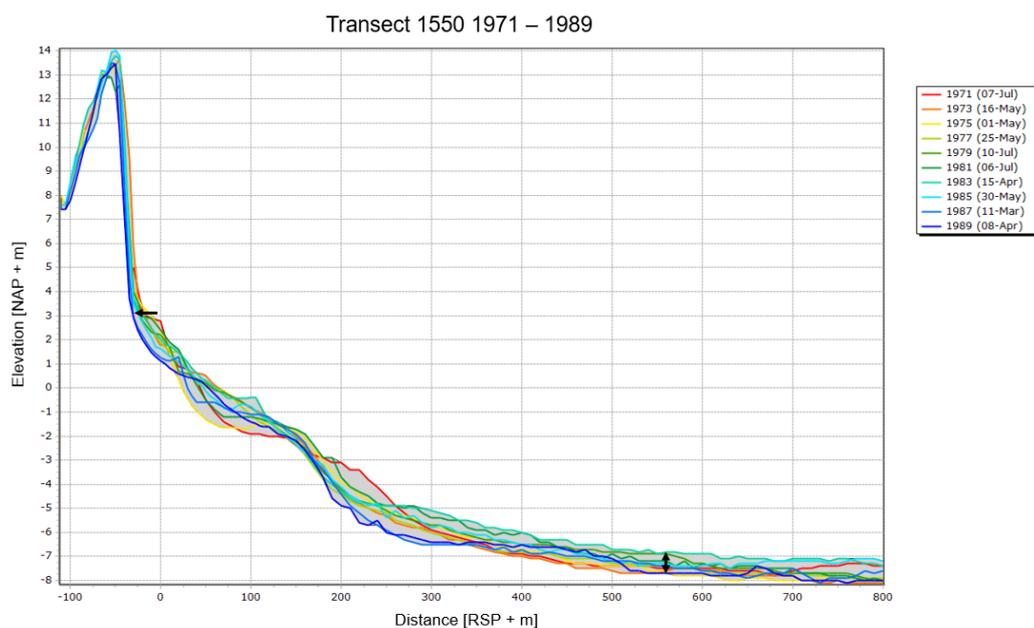
Figure 11: The cross-shore profiles at transect 1550 in the period 1971-1989, before large sand nourishments were applied. The arrows indicate the retreating dune face and the passage of transverse bars.
