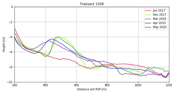
Figure 47: Cross-shore profiles of transect 1509, where the variability between 700m-1000m indicates the passage of transverse bars.
