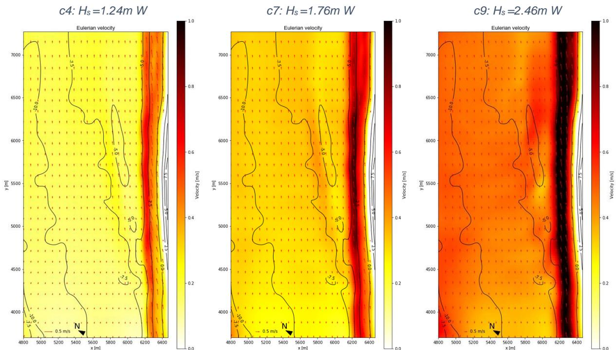
Figure 79: Magnitude of the currents under oblique ( $272-284^\circ$ ) wave conditions around a shoreface nourishment ( $T_2$ ).
