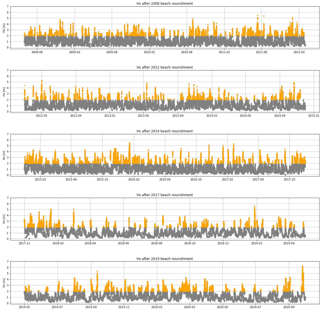
Figure 115: Significant wave height Schouwenbank. Wave height measurements above 2m have been indicated in orange to stress the high energy level of the waves.
