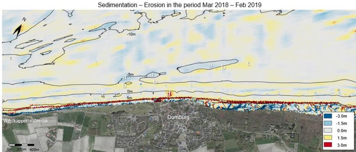
Figure 54: Sedimentation-erosion map between Mar 2018-Feb 2019, showing the morphological changes after a shoreface nourishment. The contour lines are based on the Mar 2018 survey.
