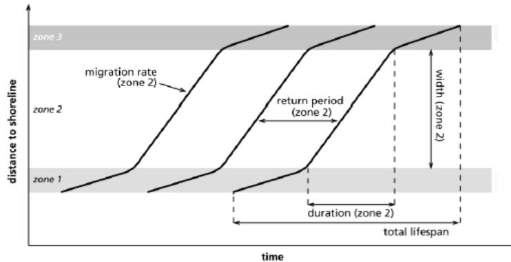
Figure 7: The cyclic pattern of multiple bars. In zone 1 the bar is initiated. When an older bar enters zone 3, the newly formed bar migrates from zone 1 to zone 2. It migrates offshore and grows larger until it reaches zone 3 where migration slows down and the bar decays. (From: Grunnet et al., 2003)
