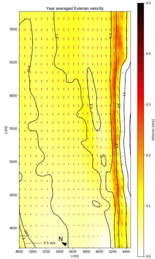
Figure 84: The year averaged Eulerian velocity for T<sub>3</sub>, with a combined beach and shoreface nourishment.
