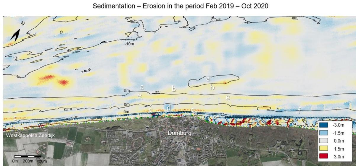
Figure 55: Sedimentation-erosion map between Feb 2019-Oct 2020, showing the morphological changes after a combined beach and shoreface nourishment. The contour lines are based on the Mar 2018 survey.
