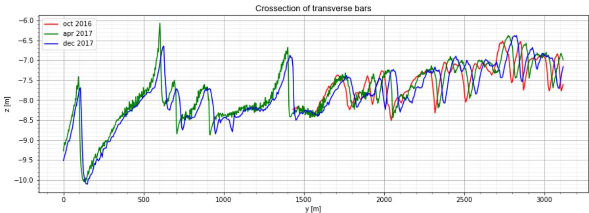
Figure 58: Cross-section of migrating transverse bars at the shoreface near Domburg, at the dashed green transect in Figure 57.
