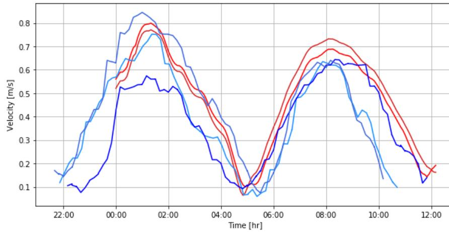
Figure 30: Comparison of measured current velocities and modelled current velocities. The measured current velocities are three random time instances from the Schouwenbank Stroomgat station [blue]. The [red] lines represent boundary conditions  $c_1$  and  $c_2$  near the offshore and west lateral model boundary.
