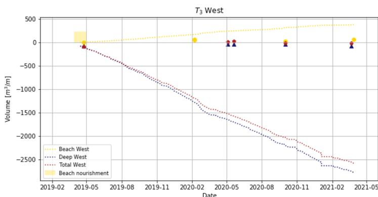
Figure 102: Comparison observed and modelled volume development west coastal zones for  $T_3$ .
