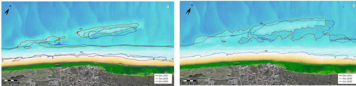
Figure 59: Migration of the shoreface bar in Dec 2017 - Oct 2020. a) The 5m contours. b) The 6m contours.
