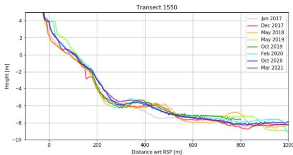
Figure 40: Transect 1550 shows no large shoreface bar but two small bodies at 450m and 750m after the 2017 nourishment.
