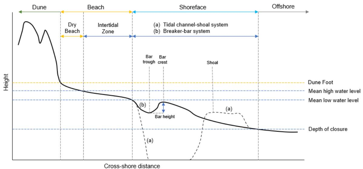
Figure 3: Definitions of coastal terms for a tidal channel-shoal system [dashed] and breaker-bar system [solid]. Adapted from: Hillmann (NLWKN).
