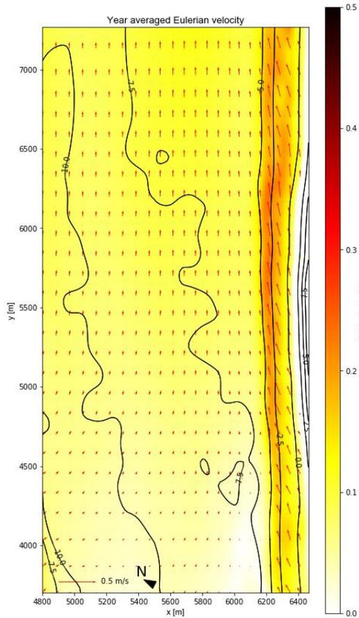
Figure 81: The year averaged Eulerian velocity for  $T_0$ , without a nourishment.
