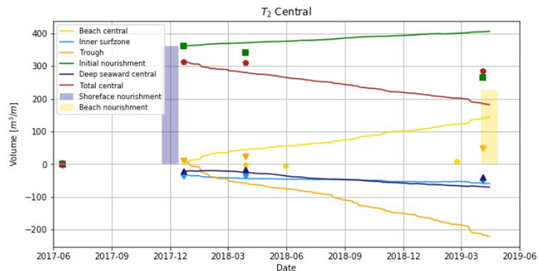
Figure 100: Comparison observed [points] and modelled [lines] volume development central coastal zones for  $T_2$ .
