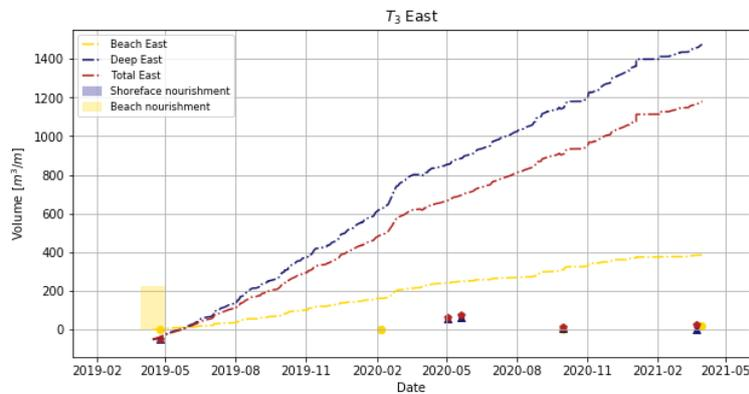
Figure 104: Comparison observed and modelled volume development east coastal zones for  $T_3$ .
