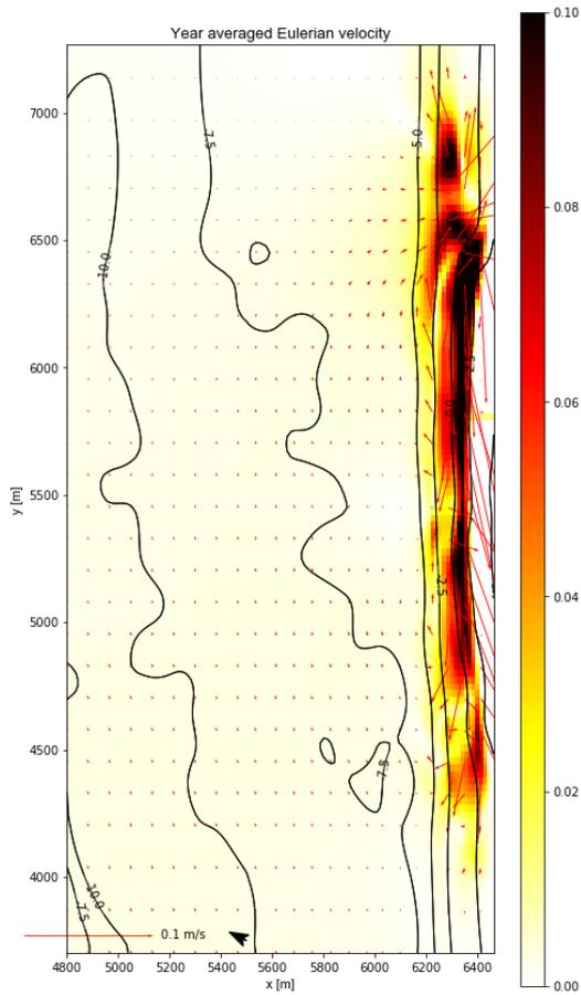
Figure 120: Year-averaged currents for  $T_1 - T_0$
