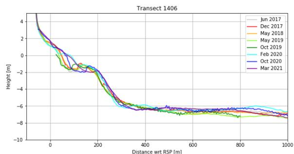
Figure 45: The second downstream transect shows extensive ridges and runnels but no emerging shoreface bar
