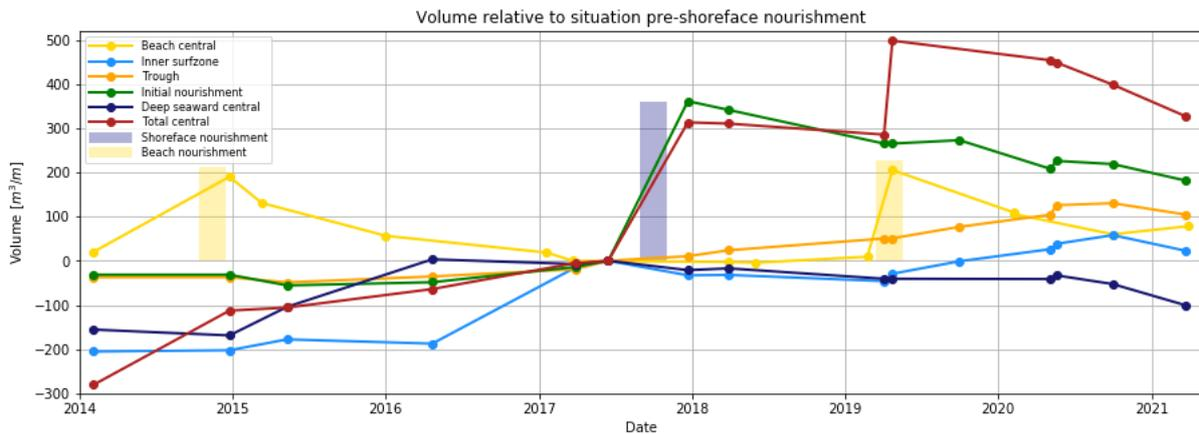
Figure 61: The relative volume change of coastal zones in the nourished transects 1632-1448, at Domburg for T<sub>1</sub>, T<sub>2</sub>, and T<sub>3</sub>.
