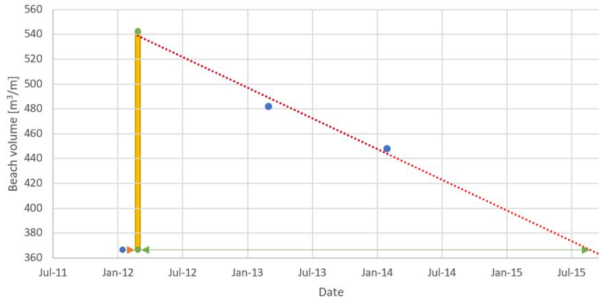
Figure 22: Example of linear fitting an erosion trend for the 2012 beach nourishment, where the volume was manually adjusted. The beach volume based on JARKUS measurements [Blue] was adjusted. The date was adjusted [Orange] and the nourished volume was added [Yellow] to create new data points [Green]. Then, a linear line [Red] was fitted through the datapoints from which the longevity [Green Arrow] was determined when the line intersects the pre-nourishment volume.
