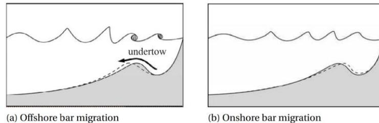
Figure 6: a) Offshore bar migration under breaking waves. b) Onshore bar migration under skewed waves (From: van den Ende, 2017)
