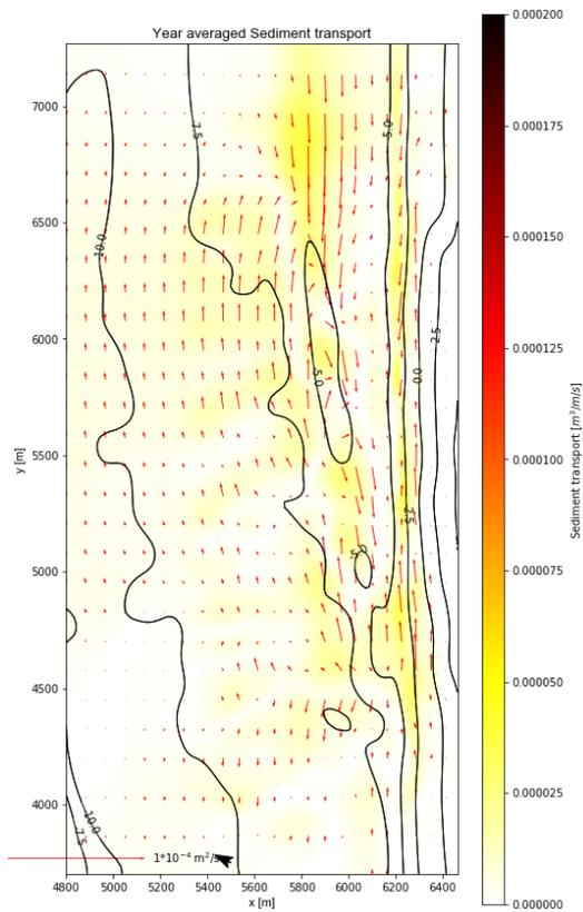
Figure 126: Year-averaged sediment transport for  $T_3 - T_1$
