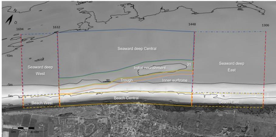
Figure 19: Top view of the coastal zones at Domburg.
