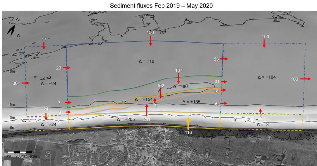
Figure 66: Sediment fluxes and volume changes near Domburg in Feb 2019 – May 2020 in  $10^3 \text{ m}^3$  estimated from measurement data. A beach nourishment was completed in May 2019 in the solid yellow polygon, while the 2017 shoreface nourishment is still present.
