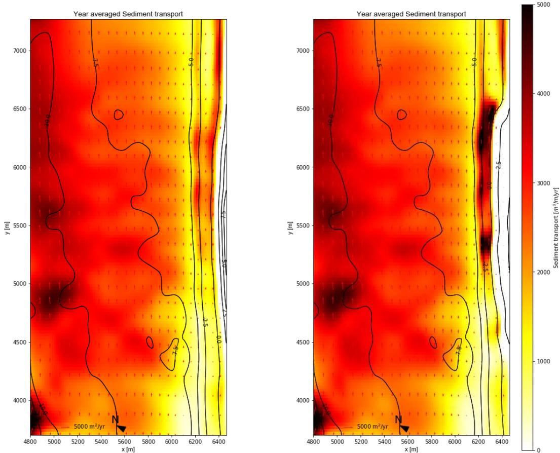
Figure 95: The year averaged sediment transport without a nourishment,  $T_0$ .
