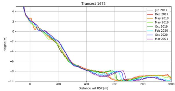
Figure 43: The second upstream transect portraying small variably ridges and runnels and the large variability on the shoreface at 600m.
