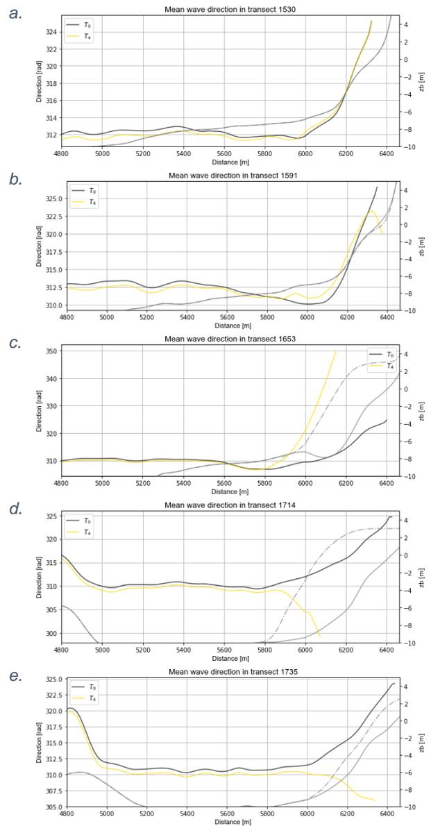
Figure 111: Year-averaged wave directions for  $T_0$  and  $T_4$  for transects a. 1530, b. 1591, c. 1653, d. 1694, e. 1735.
