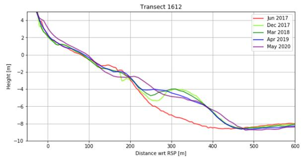
Figure 48: Cross-shore profiles of transect 1612, where the 2017 shoreface nourishment is evident between 250m - 450m and the 2019 beach nourishment at -50m - 150m.
