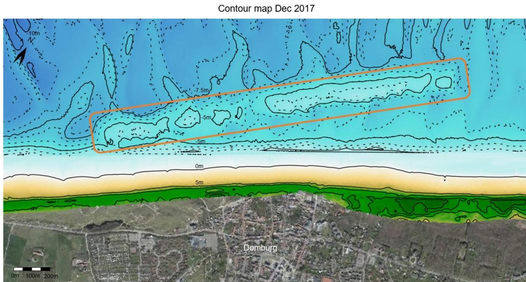
Figure 13: Contour map near Domburg, shortly after construction of the shoreface nourishment in Dec 2017 [Orange]. The subtidal contour intervals are 1m [dashed] and 2.5m [solid]. Besides the nourishment body, the transverse bars can be recognized seaward and landward of the nourishment.
