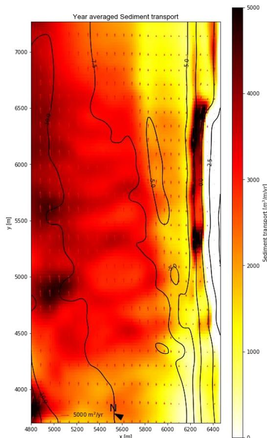
Figure 98: The year averaged sediment transport with a beach and shoreface nourishment,  $T_3$ .
