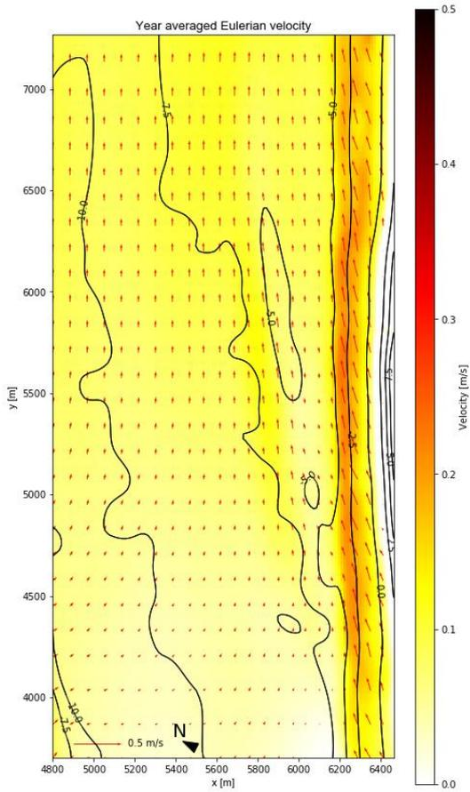
Figure 83: The year averaged Eulerian velocity for T<sub>2</sub>, with a shoreface nourishment.
