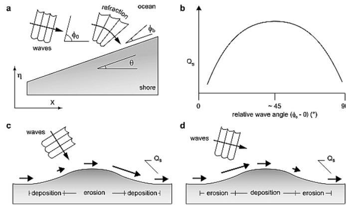
Figure 4: Response of a perturbation in the shoreline. a) Angles between incoming waves and the shoreline. b) Transport curve as a function of wave angle. c) For low-angle waves, the transport increases for higher relative angles. d) Response to high-angle waves for which the transport decreases for increasing relative angles. From: Ashton and Murray (2006).
