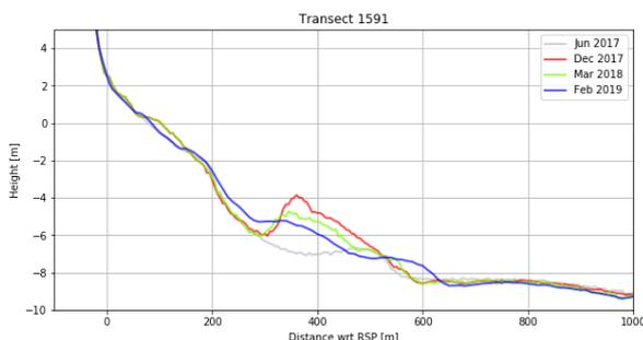
Figure 34: Cross-shore profiles of transect 1591, including the 2017 shoreface nourishment between 250-500m.
