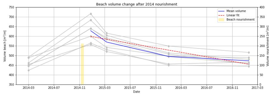
Figure 67: Beach volume change after the 2014 beach nourishment. An average erosion rate of  $-69.4\text{m}^3/\text{m}/\text{yr}$  and a lifetime of 3.1 years is estimated based on four surveys in the two years post-construction.
