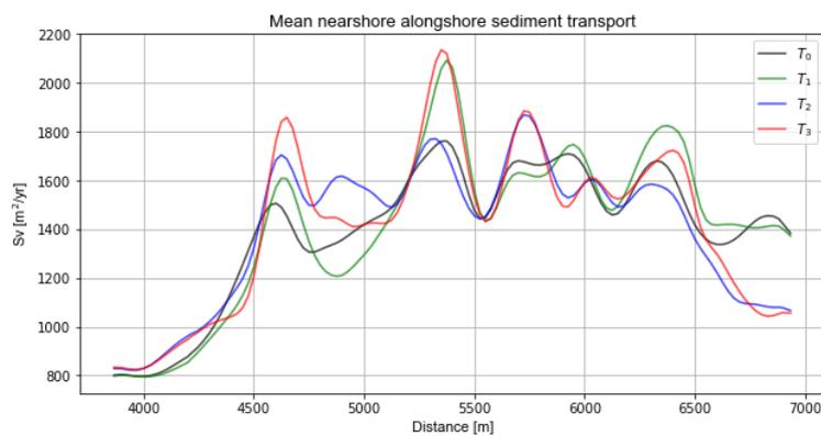
Figure 92: Mean alongshore sediment transport for wave condition c5:  $H_s=1.33\text{m}$ ,  $\Theta=328^\circ$ ,  $T_p=6.5\text{s}$  in the zone from the dune foot to 1000m offshore. Nourishments are placed between 4500-6500m.
