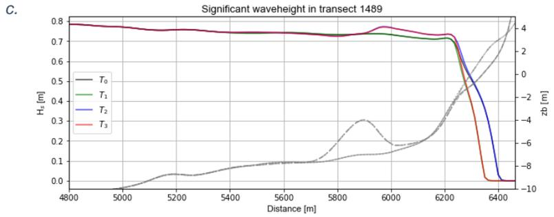
Figure 76: Annual cross-shore significant wave height for transects a) 1673, b) 1591, c) 1550, d) 1489, and e) 1406. On the secondary y-axis, the depth profiles are depicted with or without the beach and shoreface nourishments.
