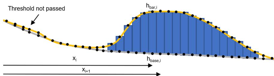
Figure 18: Visualisation of the midpoint Riemann sum to calculate a volume of a shoreface bar in a cross-shore profile. The volume is approximated by the volume of the slices between the base profile [grey] and the bar [yellow]. The XYZ data points [black] determine the slice's size. A threshold is applied to exclude small variations.
