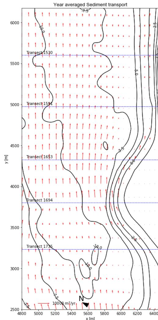
Figure 113: Year-averaged sediment transport for  $T_4$ .
