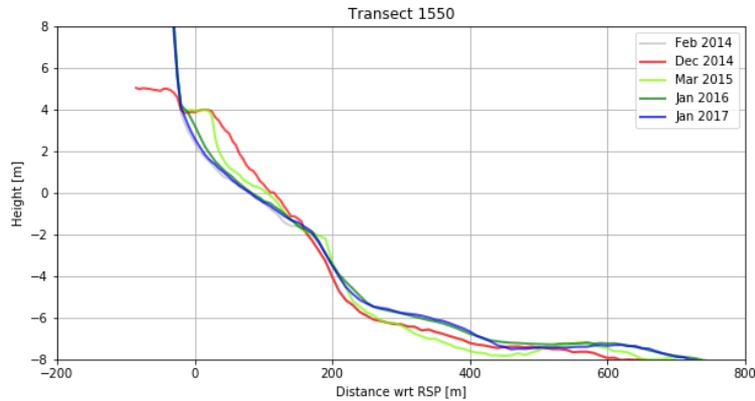
Figure 33: Cross-shore profiles of transect 1550, after the 2014 beach nourishment. The Dec 2014 survey between -100 - -50 was added manually for the beach volume calculation and does not represent reality.
