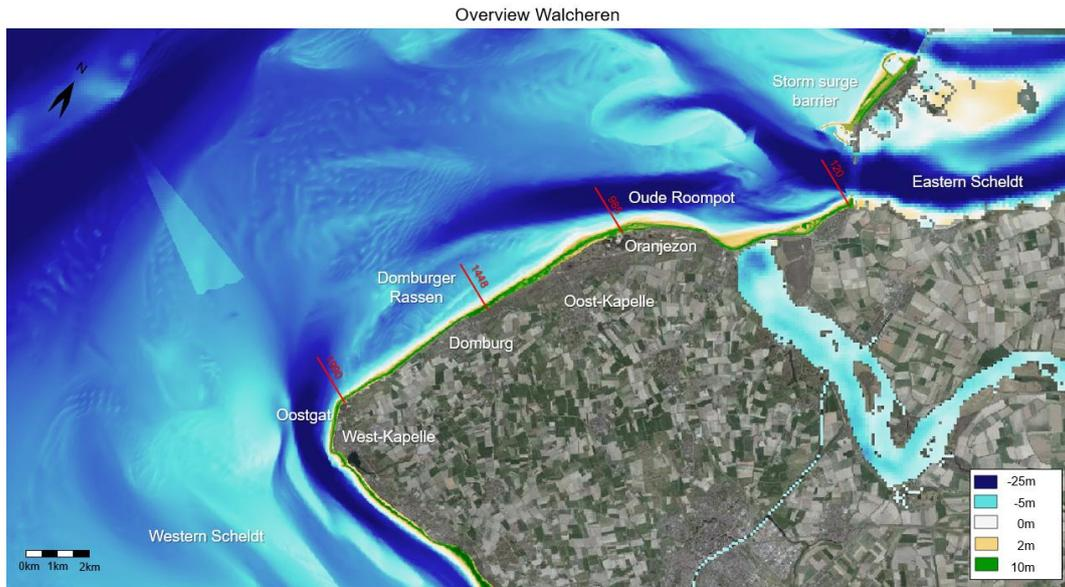
Figure 10: Overview of NW Walcheren. The villages of West-Kapelle, Domburg and Oost-Kapelle are indicated, as well as some distinct bathymetric features such as the tidal gully of the Oostgat and the Domburger Rassen. The locations of several transects are depicted [red] with the number increasing from the Eastern Scheldt storm surge barrier towards West-Kapelle. The transect number indicates the alongshore distance [dam].
