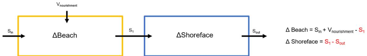
Figure 20: Example of a simple box model for a beach nourishment and the equations to find the unknown sediment fluxes [Red].
