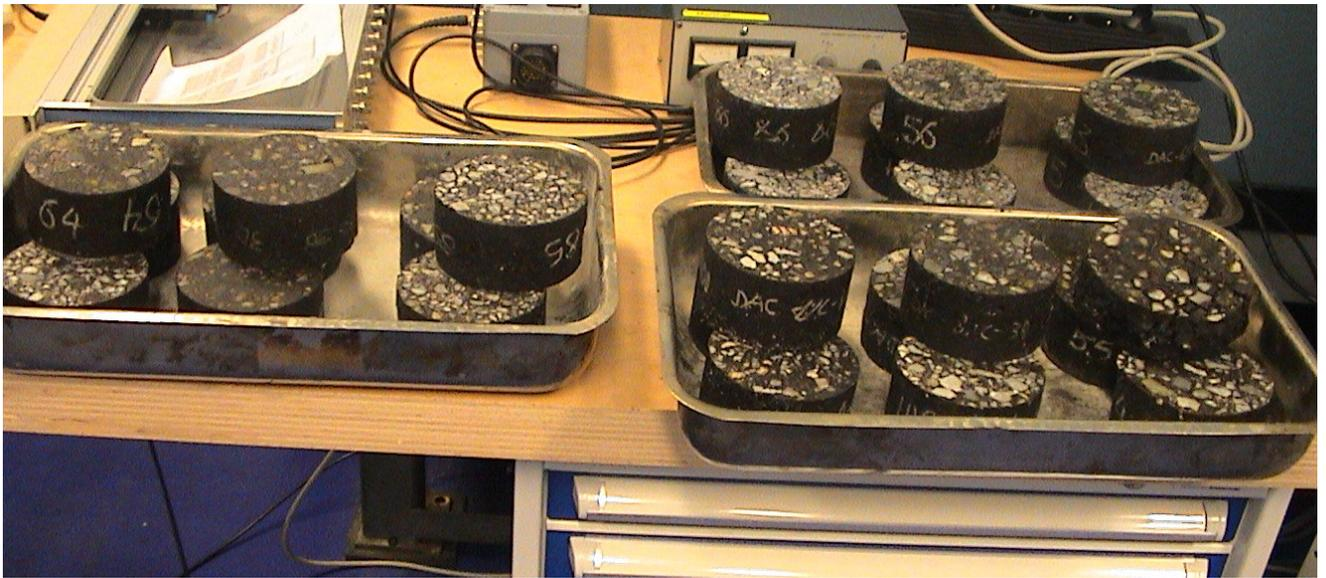
Figure 5 : Dynamic creep tested specimens @ 40, 50 and 60°C
