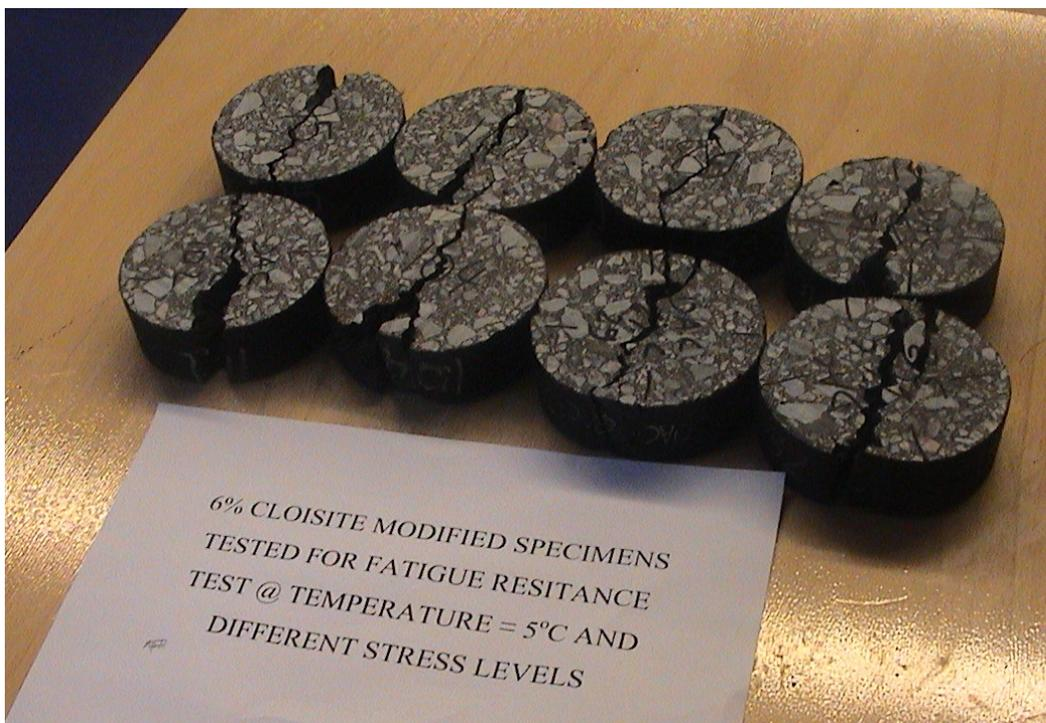
**Figure 4 : Fatigue resistance tested specimens @ 5°C**
