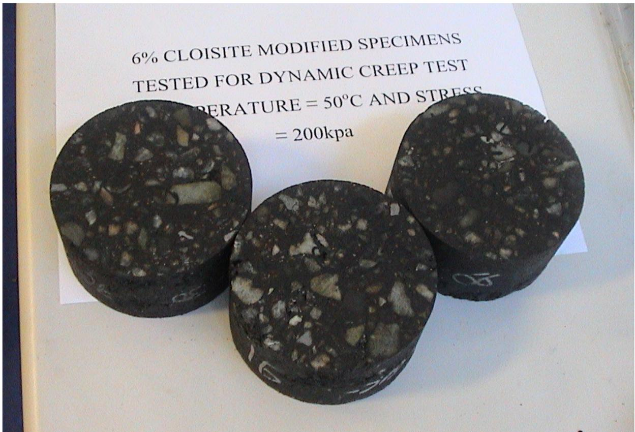
Figure 6 : Dynamic creep tested specimens @ 50°C and 200kpa (6% cloisite modified)
