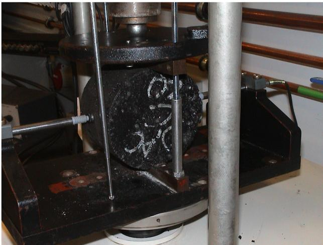
Figure 10: indirect tensile strength test
