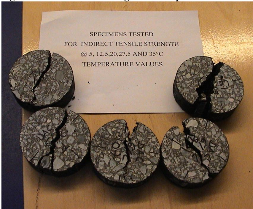
**Figure 2 : Indirect tensile strength tested specimens**
