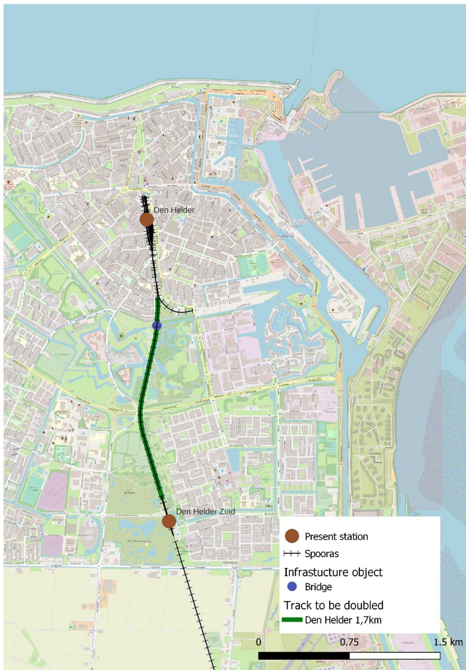
Figure 22: Track doubling Den Helder
