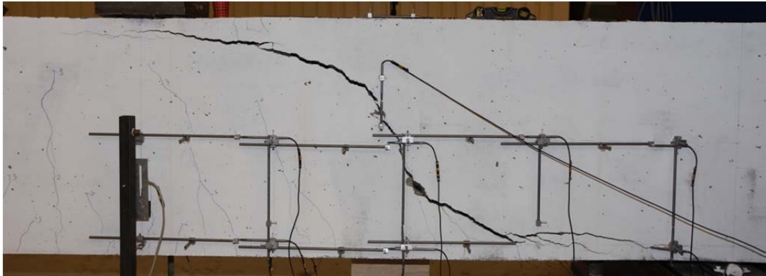
Fig. 5.102.2. Crack pattern after failure and LVDT layout at south side of beam
