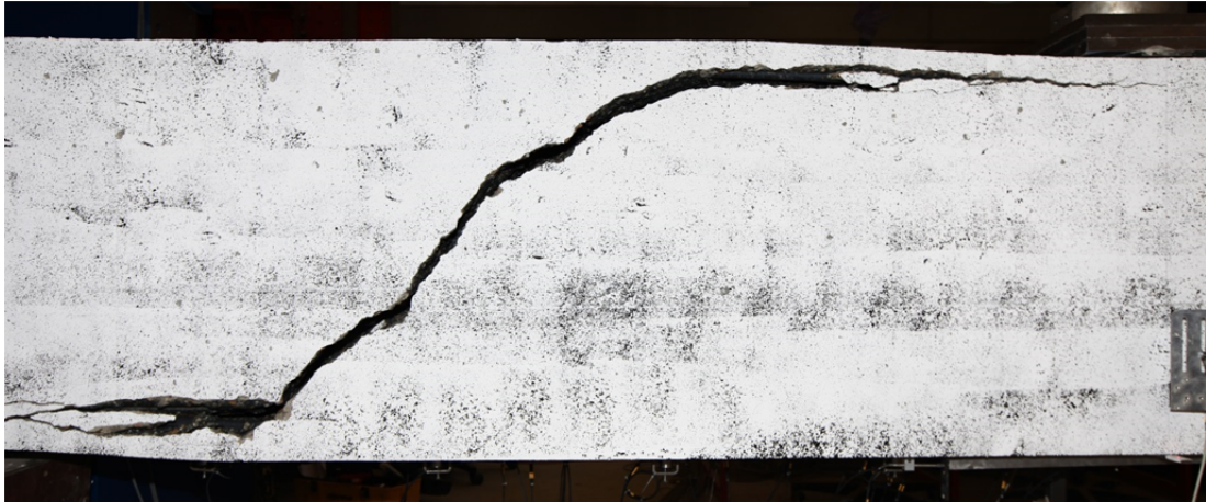
Fig. 5.93.1. Crack pattern after failure east side
