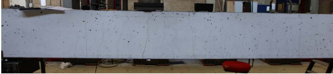
Fig. 5.82.1. Crack pattern after failure north side
