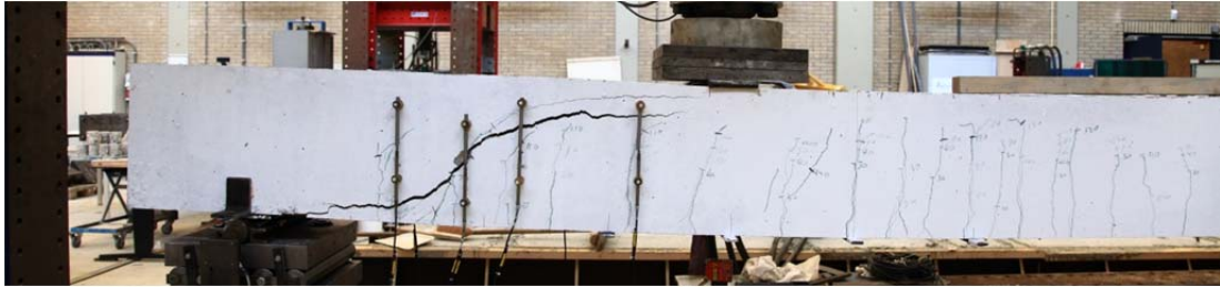
Fig. 5.3.1. Crack pattern after failure north side
