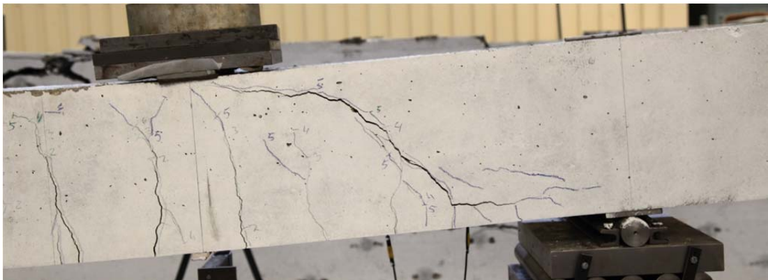
Fig. 5.32.2. Crack pattern after failure south side
