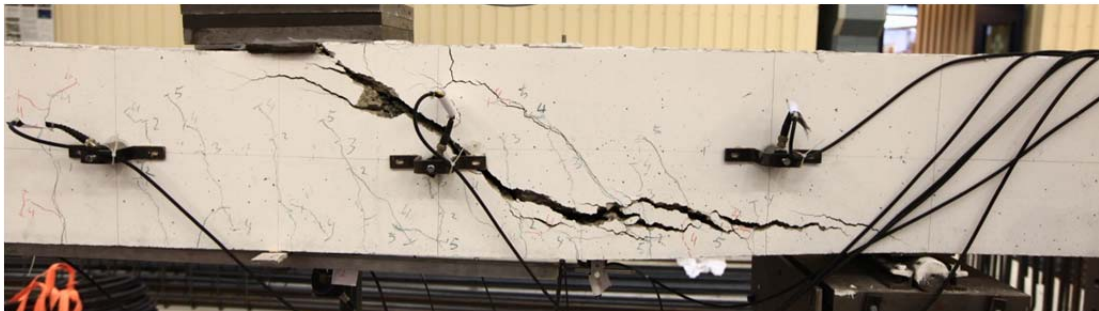
Fig. 5.55.2. Crack pattern after failure south side and sensors used for Acoustic Emission measurements
