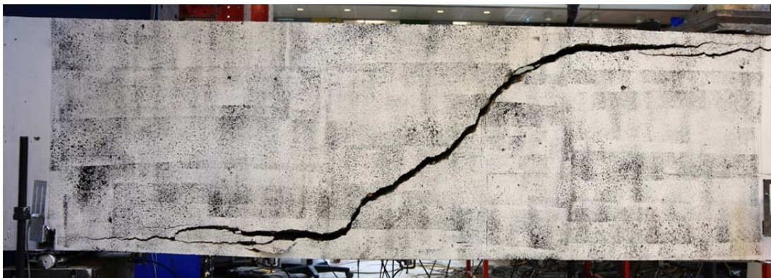
Fig. 5.94.1. Crack pattern after failure east side
