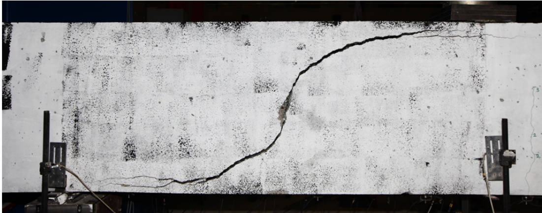
Fig. 5.101.1. Crack pattern after failure east side
