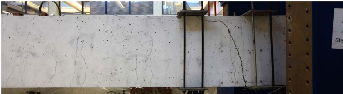
Fig. 5.86.3. Shear failure at A-side
