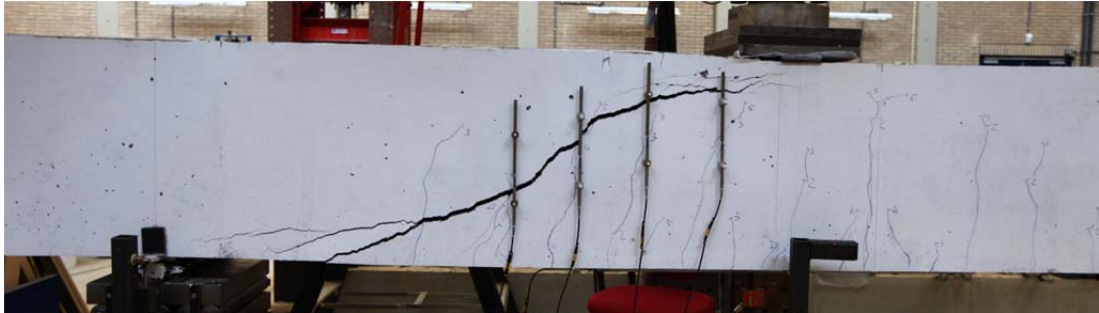
Fig. 5.44.1. Crack pattern after failure north side
