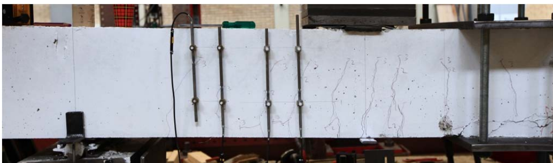
Fig. 5.69.1. Crack pattern after failure north side
