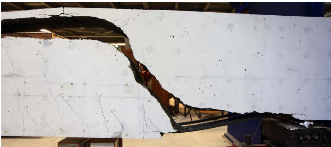
Fig. 5.107.2. Crack pattern after failure and part of LVDT layout at west side of beam
