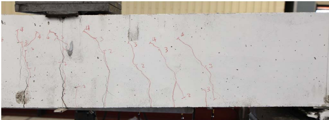
Fig. 5.67.2. Crack pattern after failure south side
