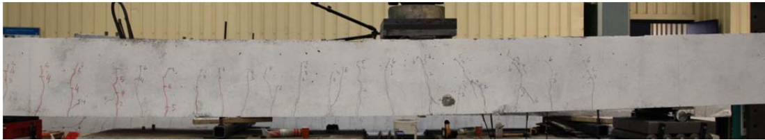
Fig. 5.20.2. Crack pattern after failure south side
