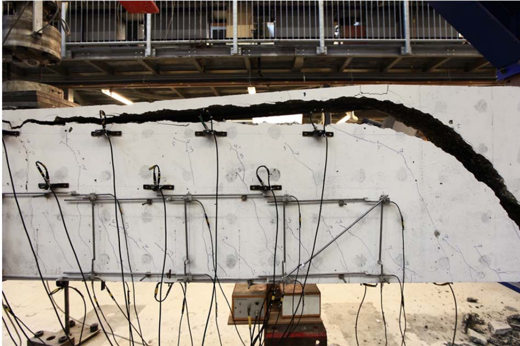
Fig. 3.2.4. Acoustic emission sensors and the LVDT grid for the deformation field.
