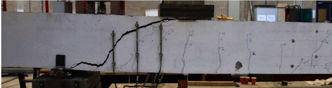
Fig. 5.37.1. Crack pattern after failure north side
