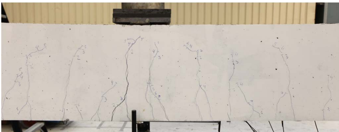
Fig. 5.50.2. Crack pattern after failure south side
