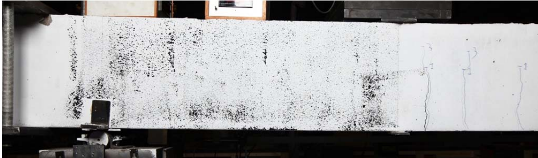
Fig. 5.71.1. Crack pattern after failure north side
