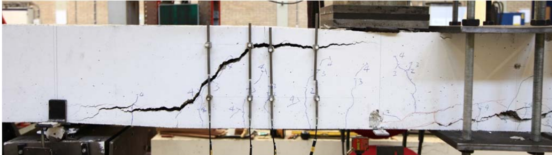
Fig. 5.56.1. Crack pattern after failure north side
