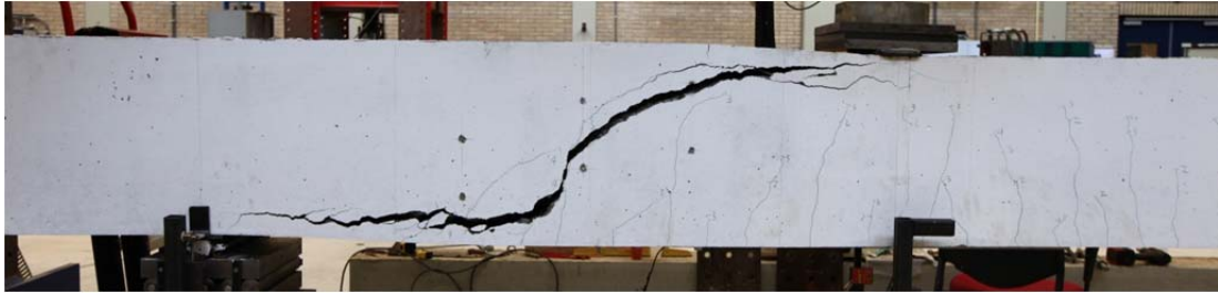
Fig. 5.49.1. Crack pattern after failure north side
