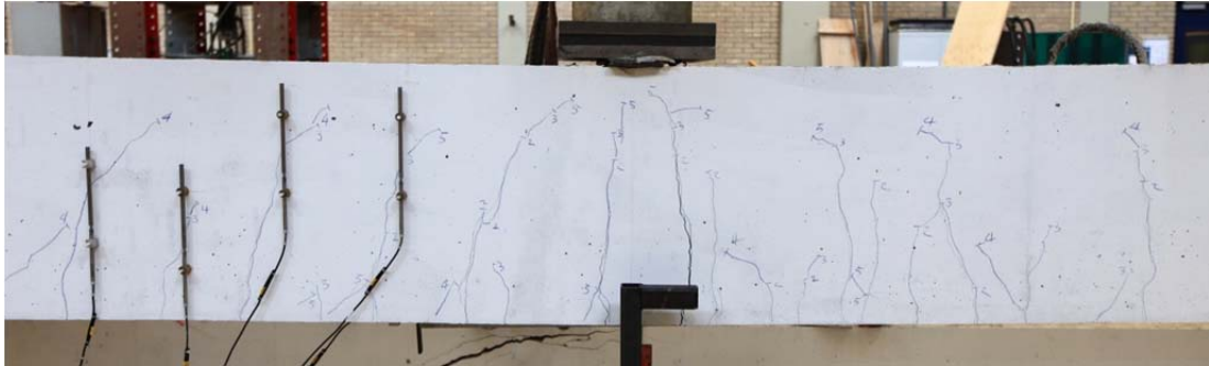
Fig. 5.50.1. Crack pattern after failure north side
