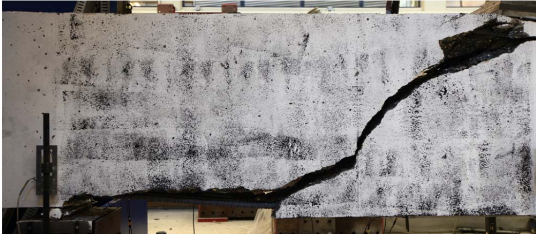
Fig. 5.100.1. Crack pattern after failure north side
