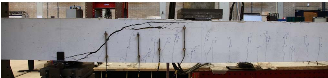
Fig. 5.6.1. Crack pattern after failure north side
