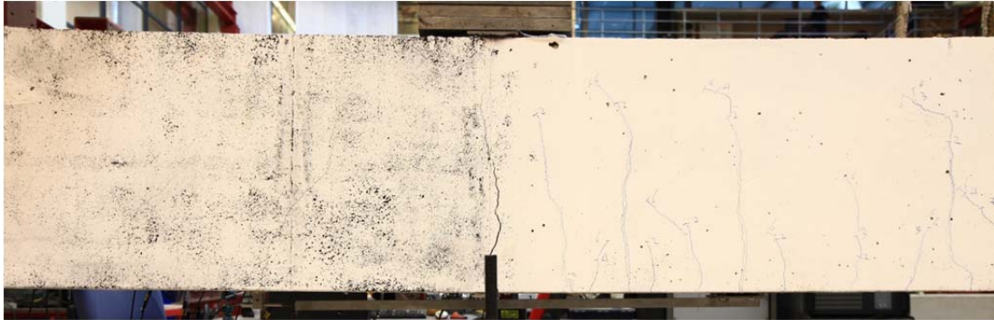
Fig. 5.97.1. Crack pattern after failure north side
