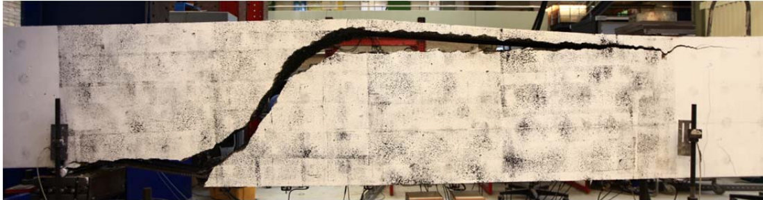
Fig. 5.106.1. Crack pattern after failure at east side of beam
