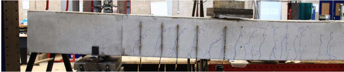
Fig. 5.13.1. Crack pattern after failure north side
