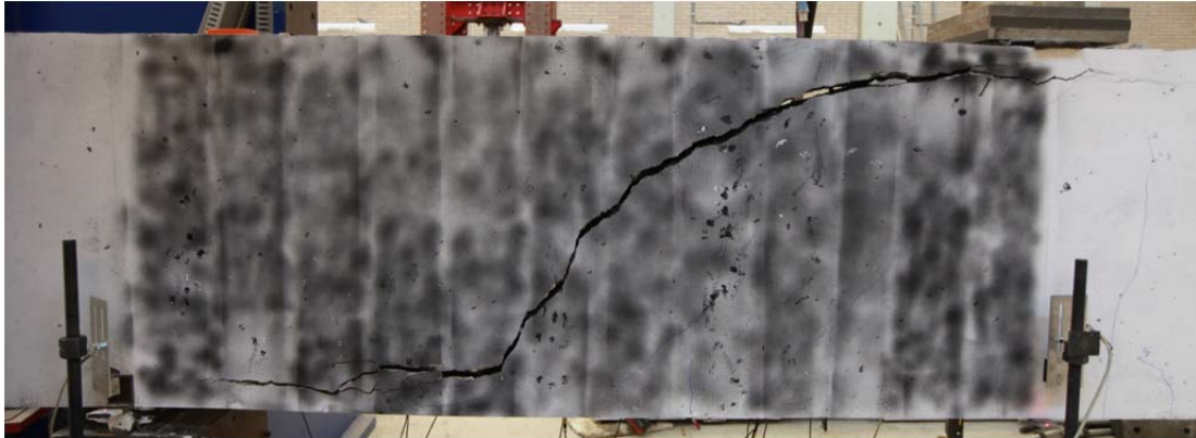
Fig. 5.87.1. Crack pattern after failure at north side of beam
