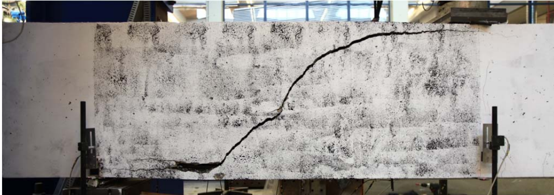
Fig. 5.89.1. Crack pattern after failure north side
