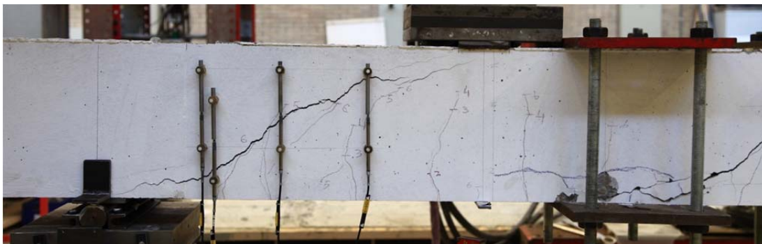
Fig. 5.7.1. Crack pattern after failure north side
