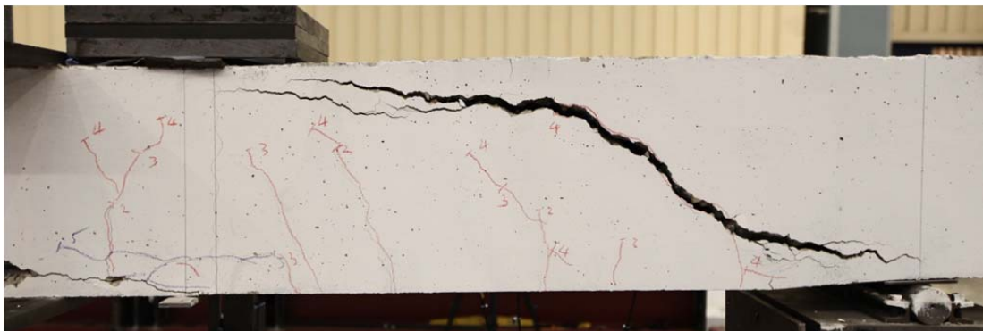
Fig. 5.60.2. Crack pattern after failure south side
