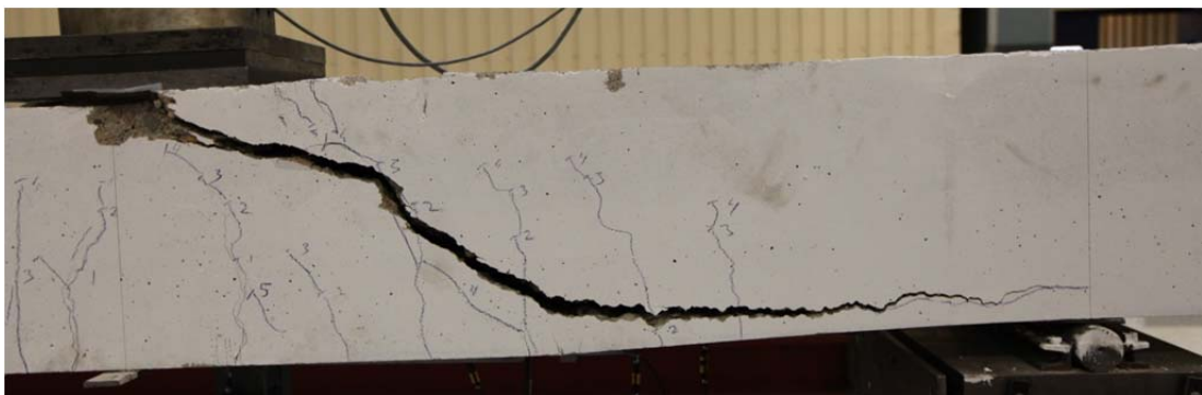
Fig. 5.61.2. Crack pattern after failure south side
