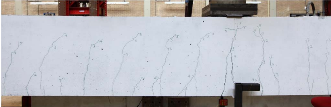
Fig. 5.40.1. Crack pattern after failure north side
