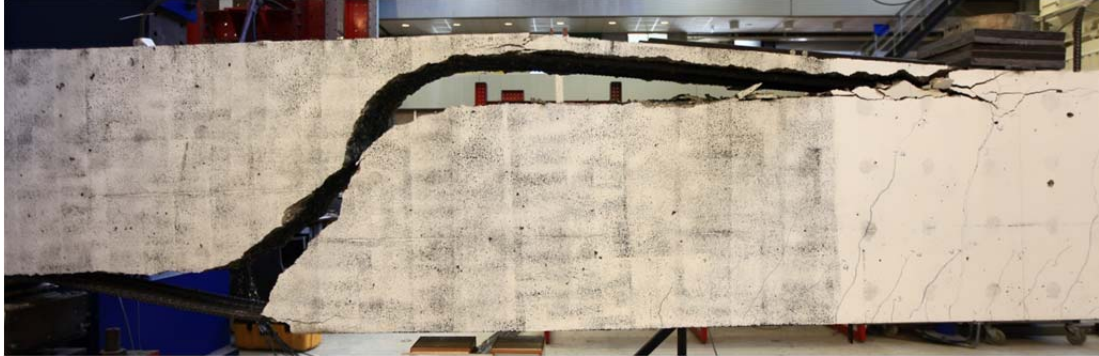
Fig. 5.107.1. Crack pattern after failure at east side of beam
