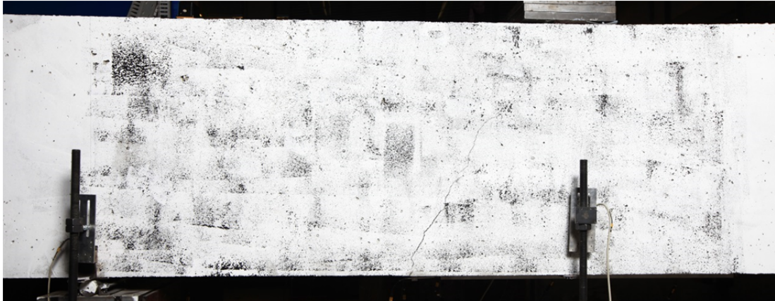
Fig. 5.86.1. Crack pattern after failure north side
