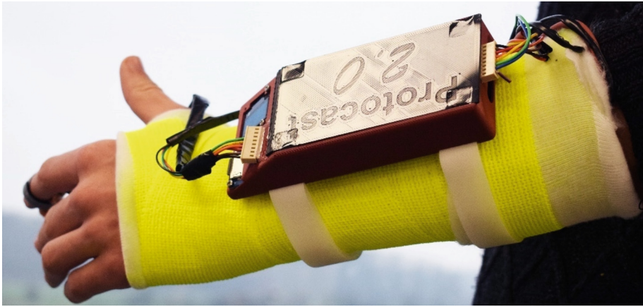
Fig. 8. Prototype of the SMC installed on the left lower arm.
