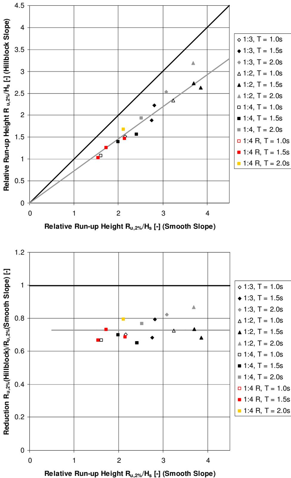
Figure 4-11: Wave run-up reduction on Hillblock slope as compared to smooth slope (irregular wave tests)
