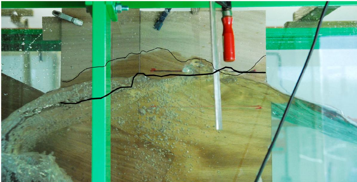
**Figure 4-2: Breaking wave at the toe of the smooth slope and water surface envelope at the toe of smooth slope (thin line) and Hillblock slope (thick line)**
