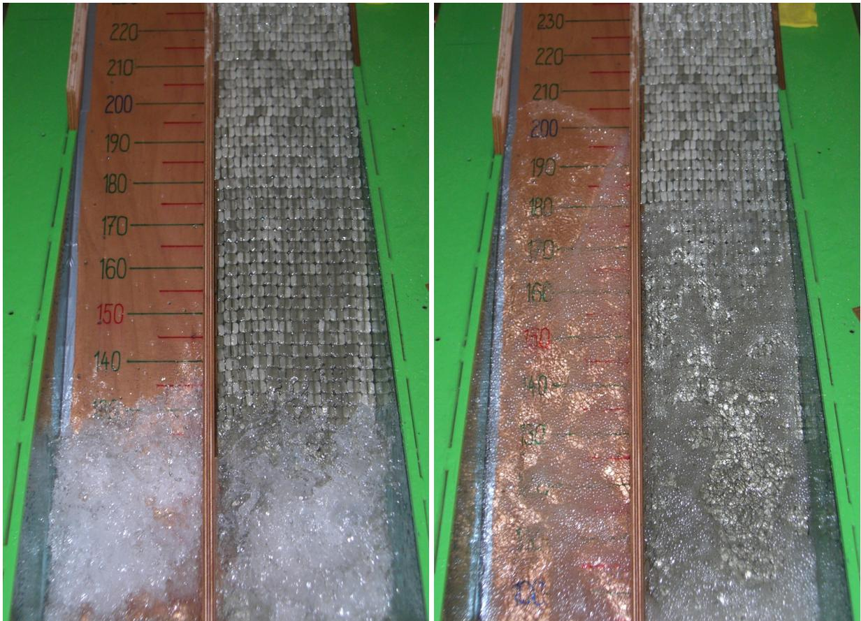
Figure 4-4: Wave breaking (left) and wave run-up (right) on 1:3 slope
