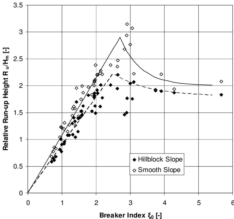
**Figure 4-6: Relative run-up height vs. breaker index (regular wave tests)**
