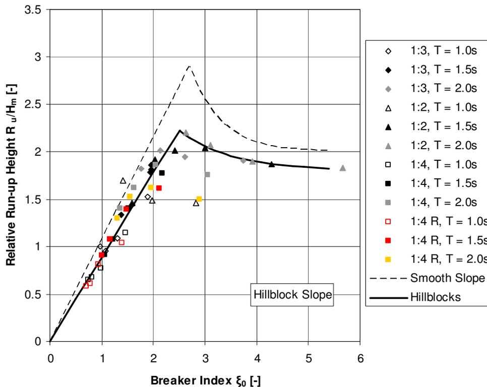
Figure 4-5: Relative run-up height on reference slope (top) and Hillblock slope (bottom) vs. breaker index (regular wave tests)
