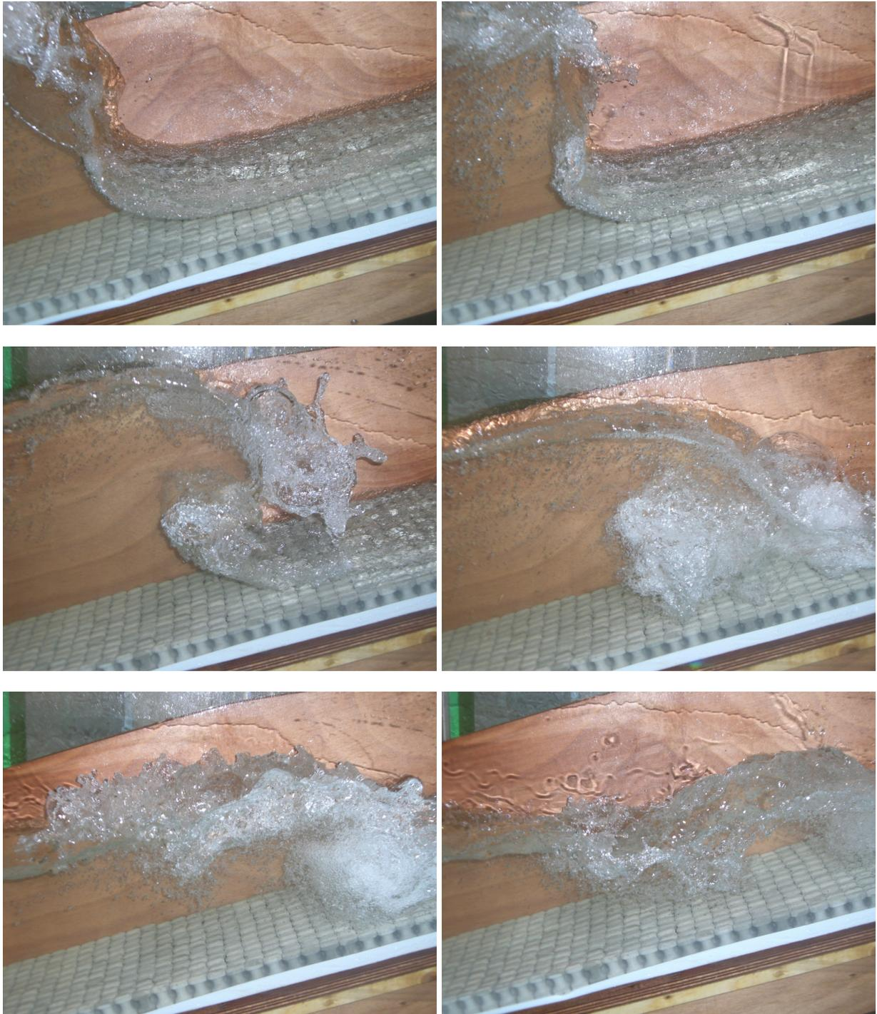
**Figure 4-3: Breaking wave on Hillblock slope (1:3)**
