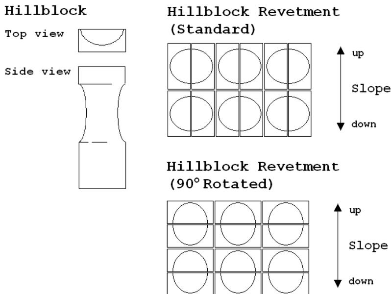
Figure 2-5: Hillblock geometry and placement pattern (sketch, not to scale)
