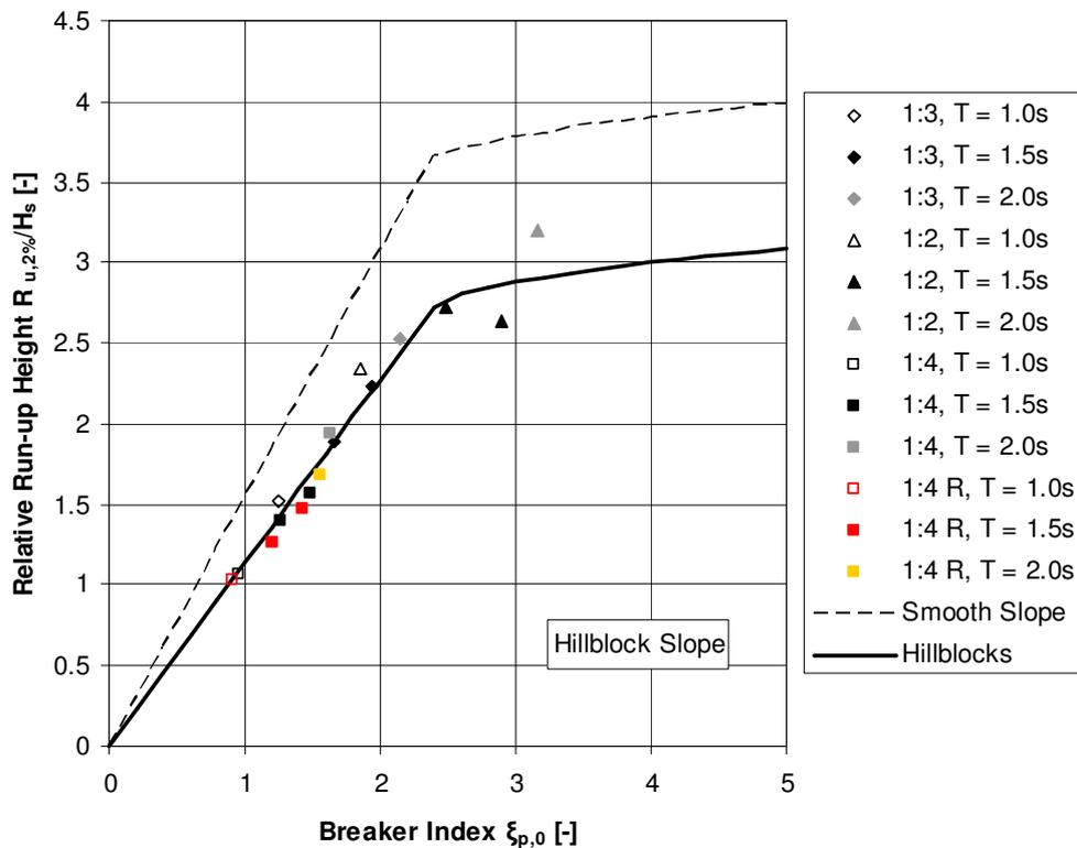
Figure 4-9: Relative run-up height on reference slope (top) and Hillblock slope (bottom) vs. breaker index (irregular wave tests)
