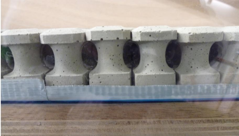
**Figure 2-3: Detail of Hillblock revetment**
