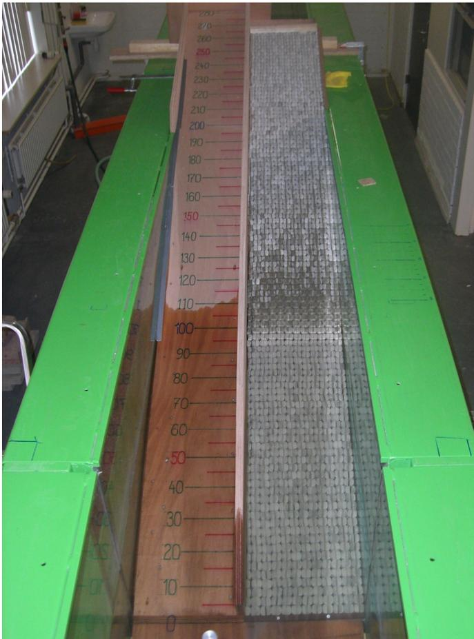
**Figure 2-4: Dike slope (1:3) with Hillblock revetment and reference slope (front view)**
