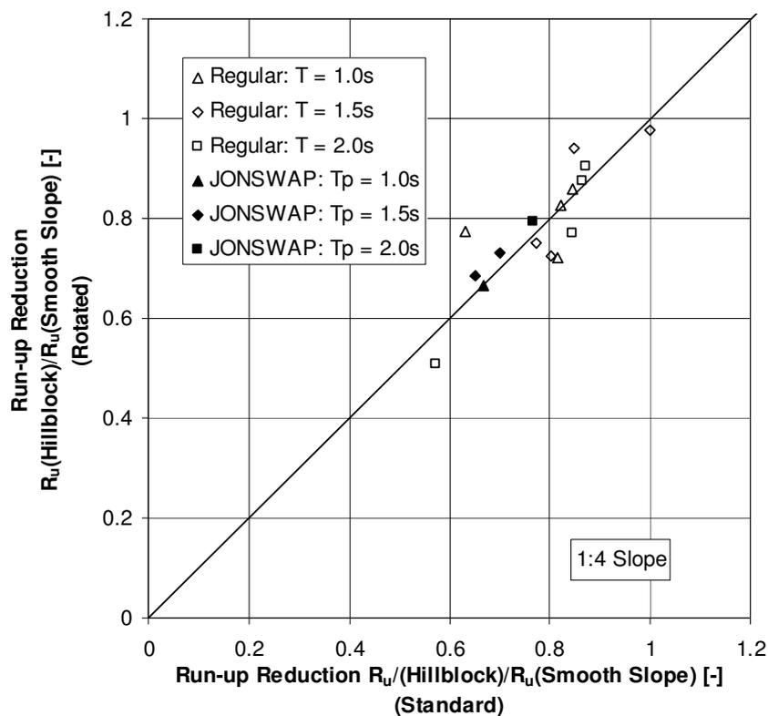
Figure 4-13: Run-up reduction on Hillblock slope with modified placement pattern as compared to standard placement pattern (regular and irregular wave tests)
