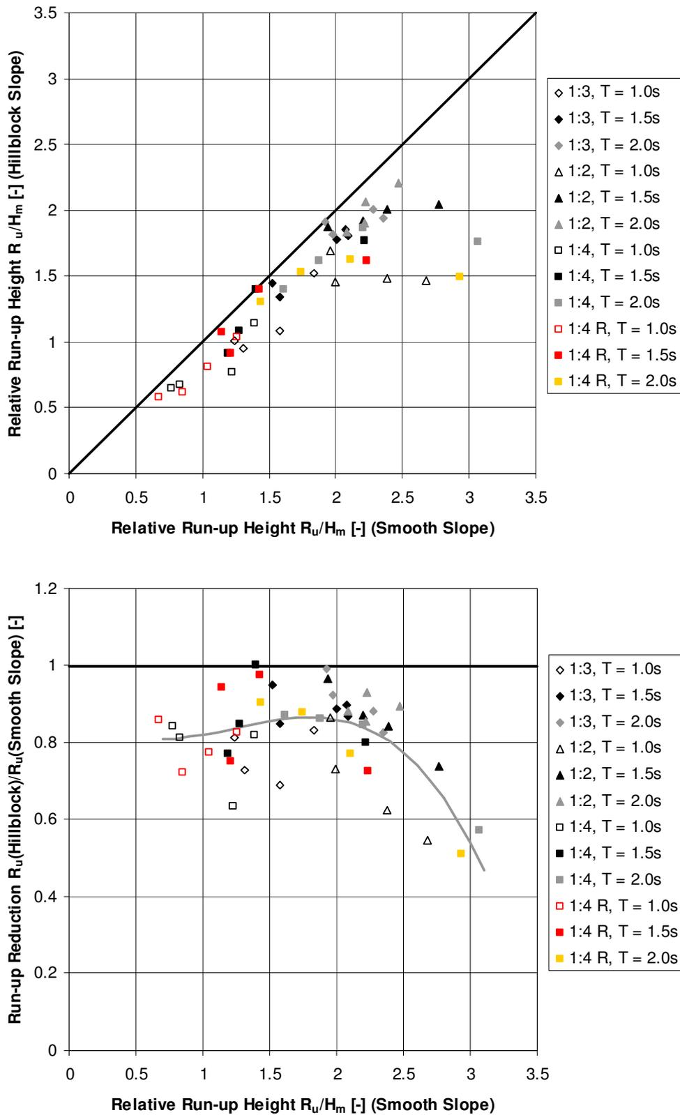
Figure 4-7: Wave run-up reduction on Hillblock slope as compared to smooth slope (regular wave tests)
