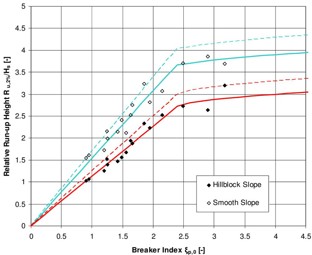
Figure 4-15: Relative run-up heights on various types of dike slopes according to literature (top) and measured run-up heights on Hillblock slope and reference slope (bottom)
