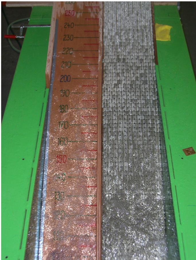
**Figure 4-8:** Asymmetrical wave run-up on 1:3 reference slope (to 215 mark) and on Hillblock slope (to 170 mark)
