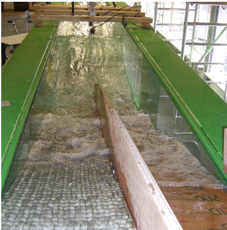
**Figure 4-1: Wave run-up on Hillblock slope and reference slope (1:3 slope)**
