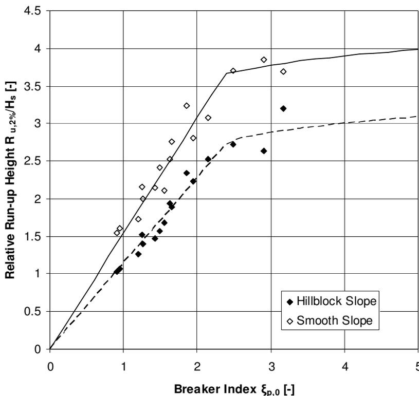
**Figure 4-10: Relative run-up height vs. breaker index (irregular wave tests)**
