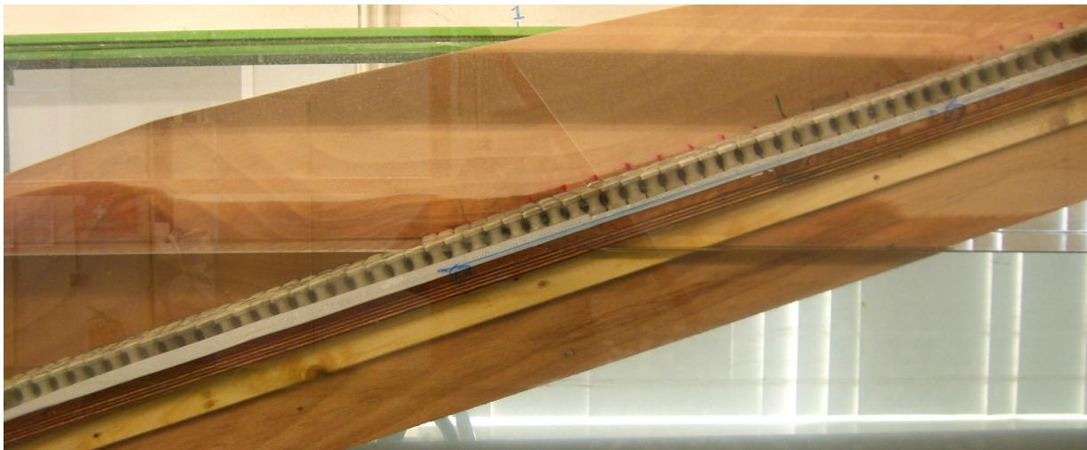
**Figure 2-2: Side view of Hillblock revetment (1:3 slope)**
