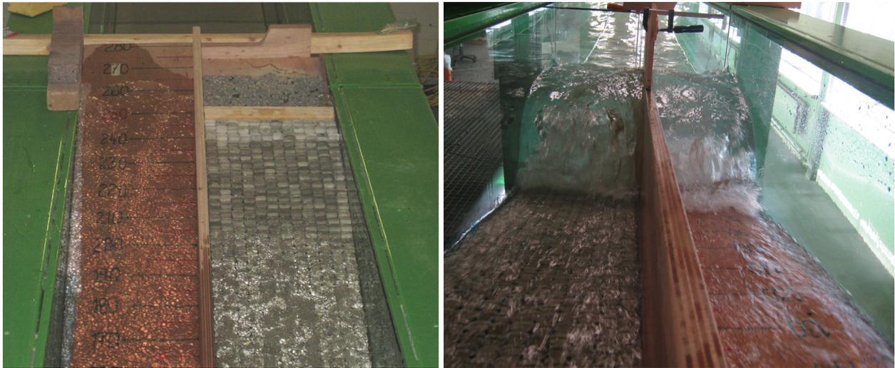
**Figure 4-14: Exceptional high wave run-up (left) and wave breaking (right) on 1:4 slope with modified Hillblock placement pattern**
