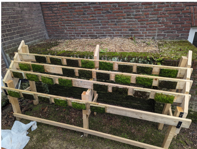
Fig. 3. Outdoor incubation setup with moss-covered concrete samples immediately after removing the light-blocking mesh cloth (following 3 months of outdoor incubation).
