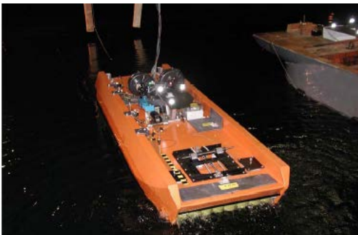
Fig. 5. DTMB model 5687 used for NSWCCD testing of ONR generic T-Craft.
