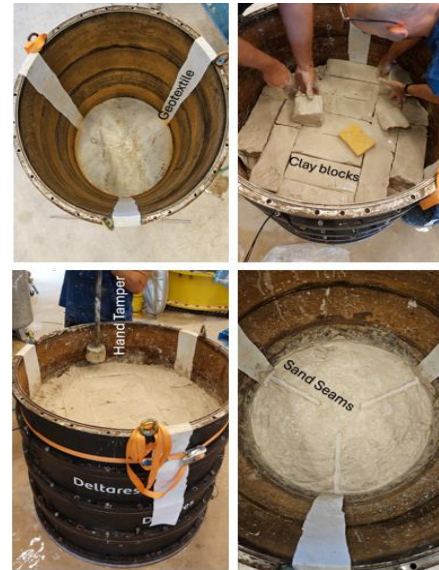
Figure 4. Top left – geotextiles used for vertical drainage, top right – assembly of clay blocks prior to hand tamping (bottom left), bottom right- introduction of sand seams for accelerated drainage.
