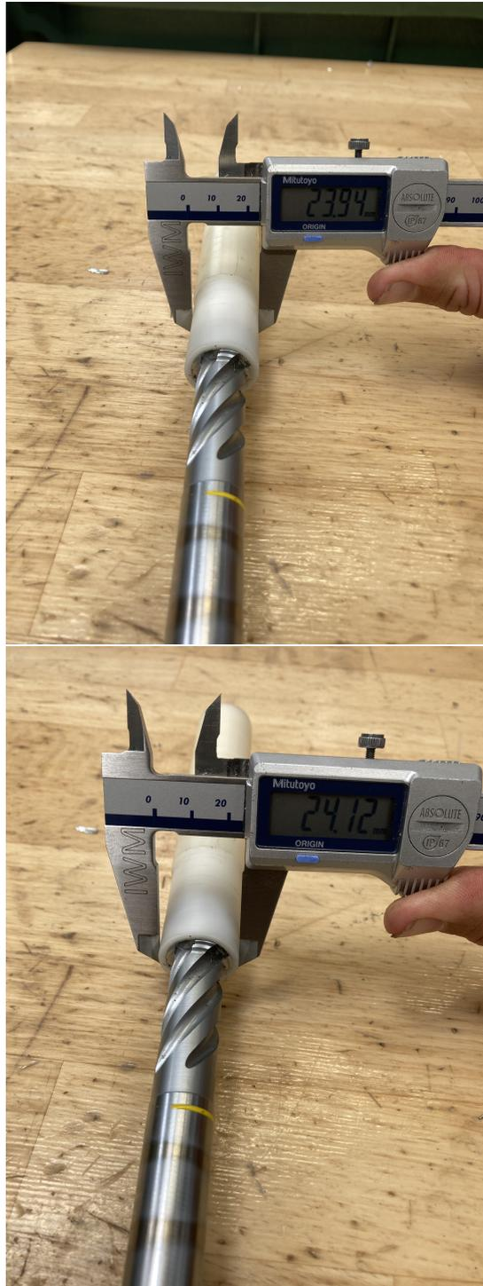
Figure B.2: Difference in outer diameter with thread cutting tool inside part.
