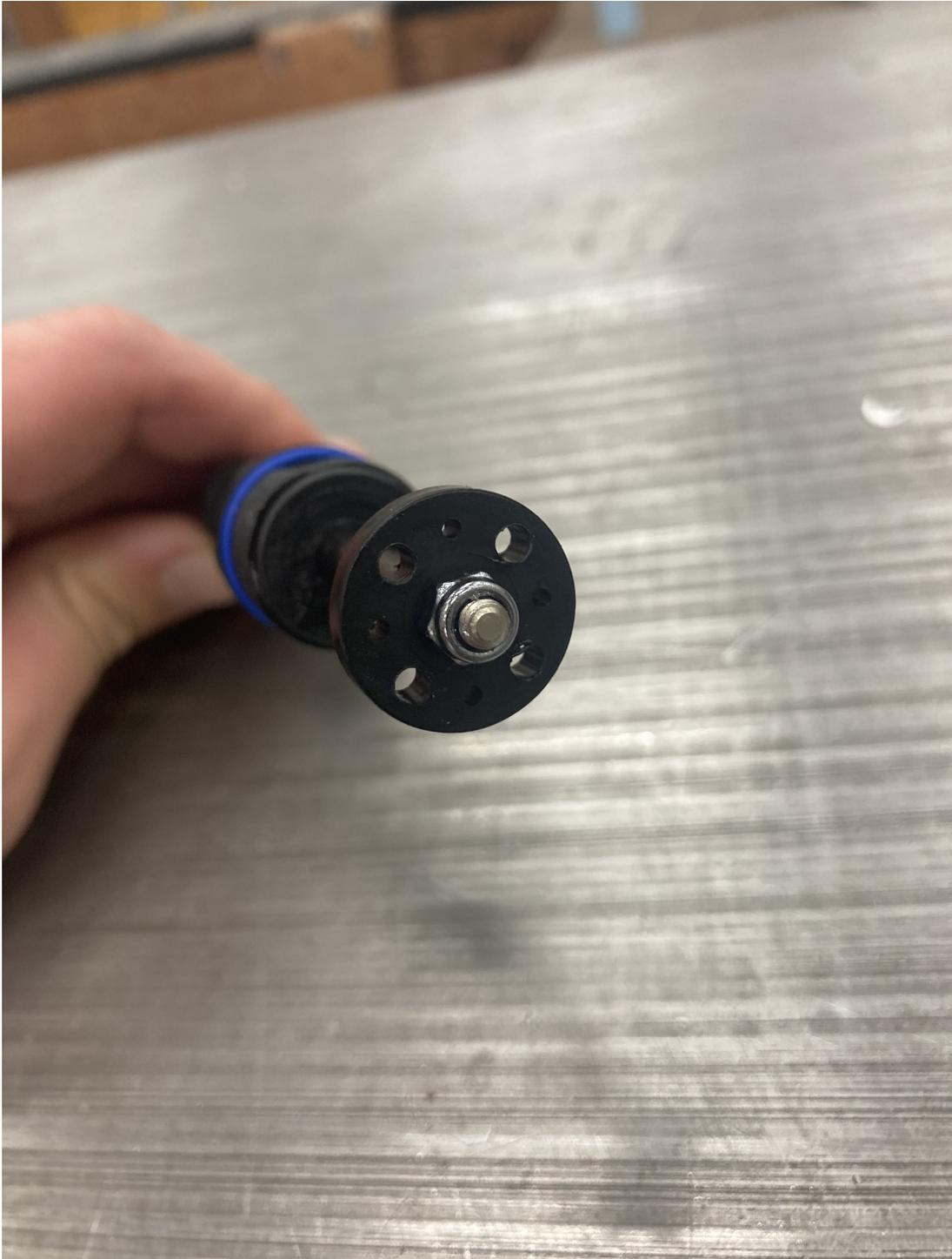
Figure B.4: Four holes reamed and the other 4 still in their original shape in the cylinder of the shock absorber
