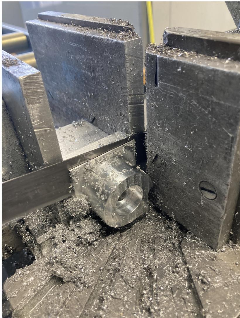
Figure B.7: Cutting of hinge part
