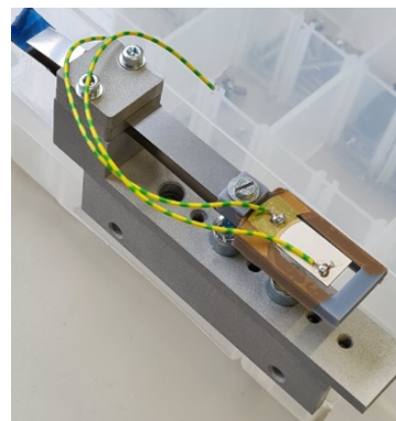
Figure H.5: a) 3D model of the proposed frequency up-converter. b) Picture of manufactured frequency up-converter.
