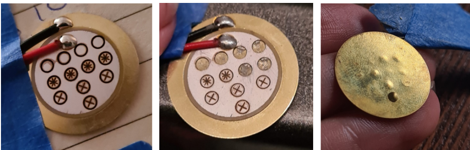
Figure 3.6: Depiction of the the different patterns that were laser cut, the induced cracking and the resulting damage of the brass.
