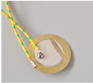
Figure 3.7: Ceramic removed in a single pass.
