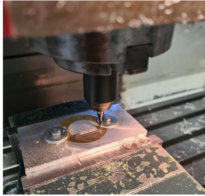
Figure 3.2: Milling of a piezoelectric audiobuzzer element
