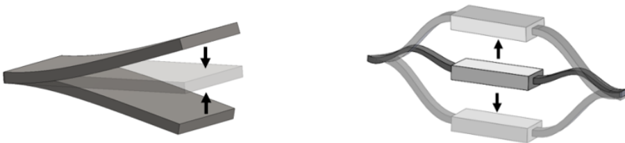
Figure 4.2: Visualization of the restoring force acting on the cantilever (on the left) and the out of plane force as a result of buckled flexures (on the right).
