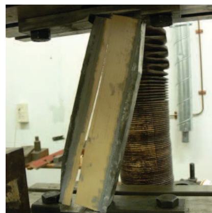
Figure 12: Spruce specimen: Failure of 0% in the glueline.
