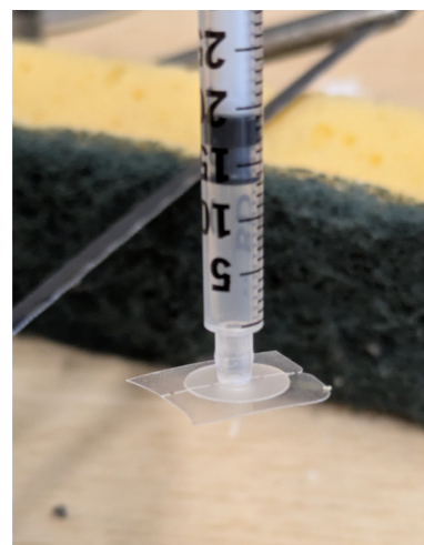
Figure 3.38 : Testing power of vacuum seal with pimple patch
