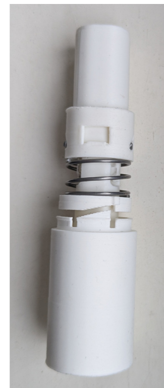
Figure 4.14 : Applicator with first ratchet mechanism
