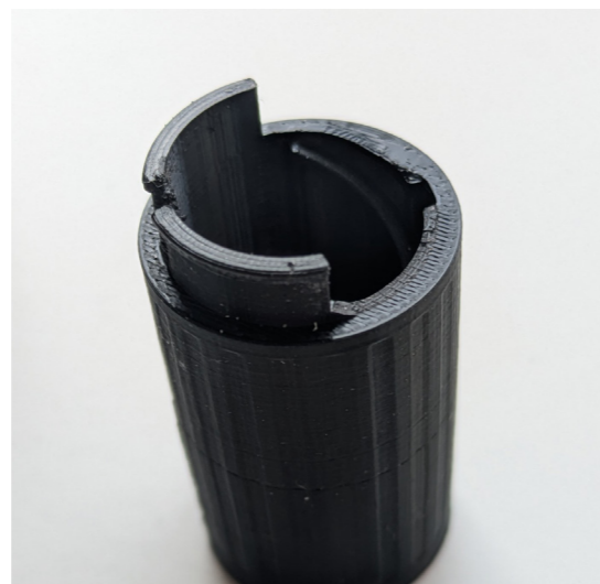
Figure 4.43 : PET G print whit broken fits
