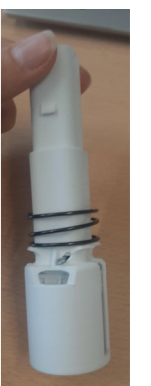
Figure 3.30 : Internal components of uPATCH PLUS applicator
