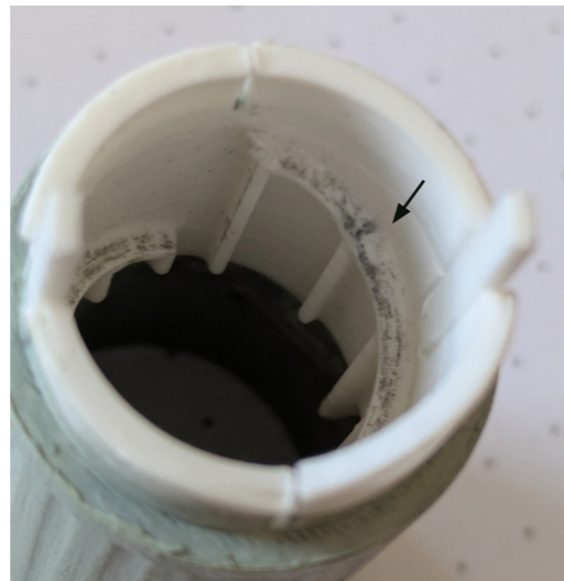
Figure 4.42 : Rotary cylinder with an damaged elevation groove
