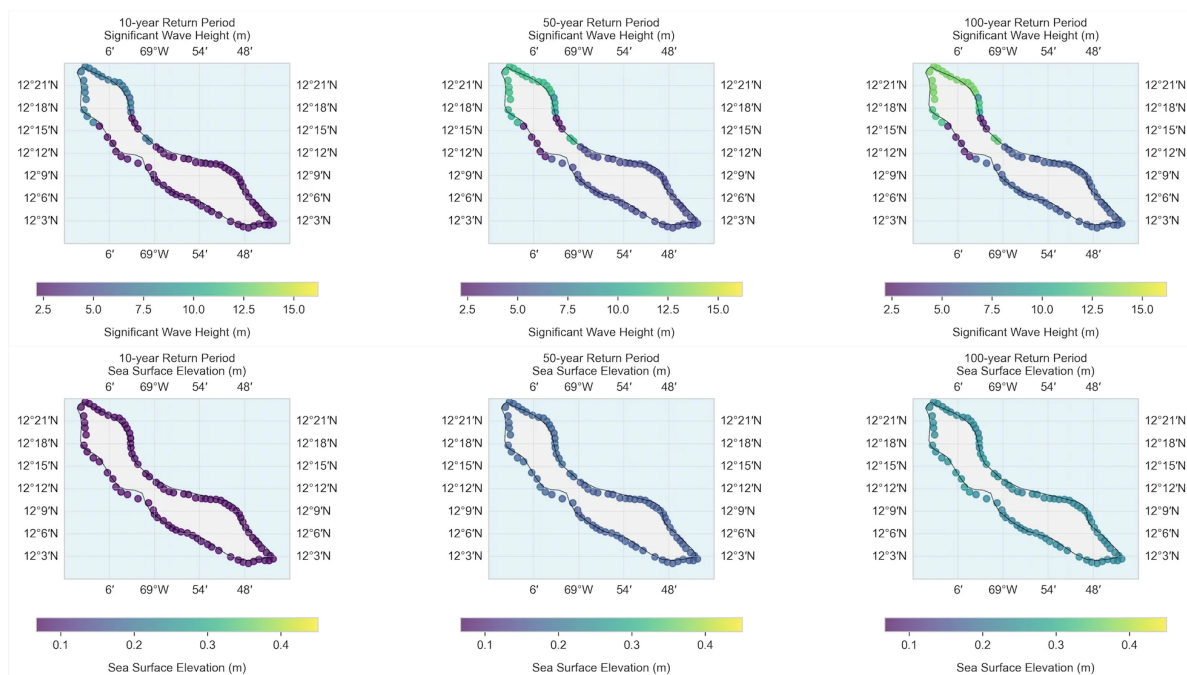
Figure 3.2: Hs and SSE levels for tropical cyclone events in the Curaçao region. The spatial maps show 10, 50, and 100-year return periods derived from 1000 synthetic tropical cyclones representing present-day climate conditions. Source: Analysis based on [89].
