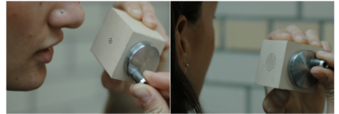
Figure 2.4 - Energy Memento Prototype, Crank-Sound Box. Turning the crank on one face records sound using energy collected from cranking; turning the crank the opposite direction plays the recorded sounds through the speaker on the opposing face (Pierce, 2010).
