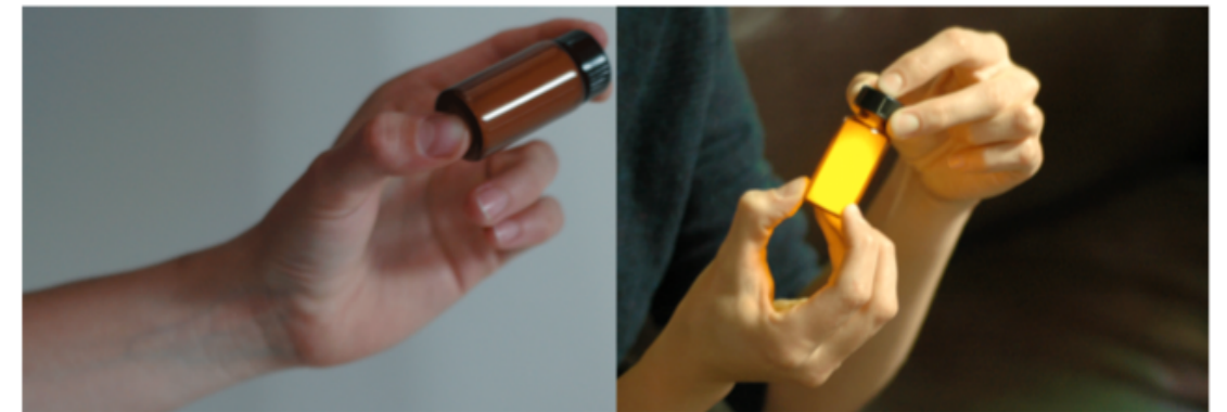
Figure 2.6 - Energy Memento Prototype, Shake-Light Bottle. Shaking the bottle collects energy; removing the cap activates the light energy (Pierce, 2010).
