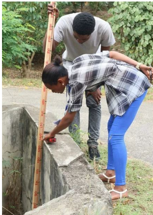
Figure 3.6: Mapping of a culvert on 12 September 2017, using measuring stick, tape measure and smartphone. http://ramanihuria.org/art-drainage-mapping-dar-es-salaam/ .
