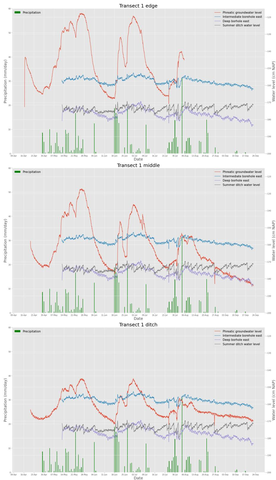
Figure C.4: Pressure monitor data for the boreholes along Transect 1 as well as the deep borehole pressure monitor data between the 16<sup>th</sup> of April and the 23<sup>rd</sup> of September.
