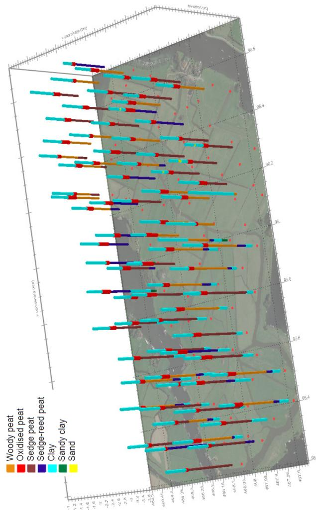
Figure A.1: Borehole subsurface composition data [DINOLOket, 2021].
