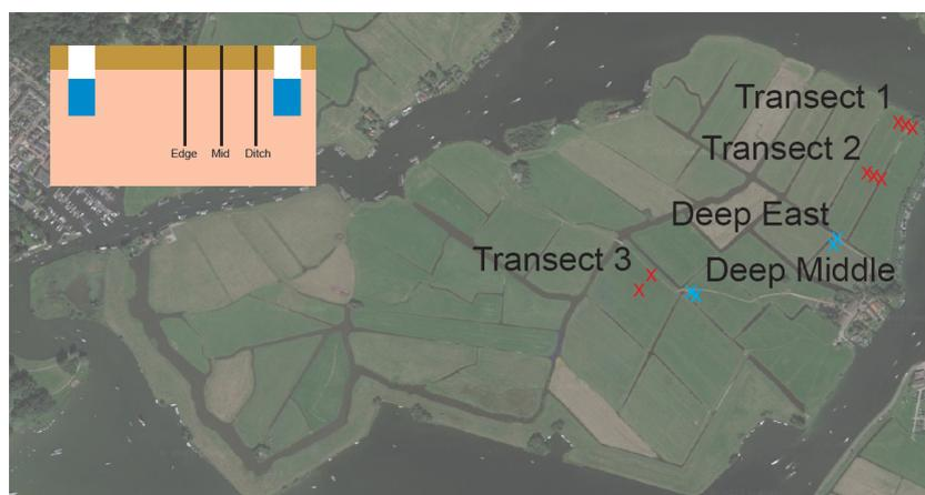
Figure 4.3: Locations of the installed boreholes. Red X are the shallow boreholes and the blue X are the intermediate and deep boreholes.
