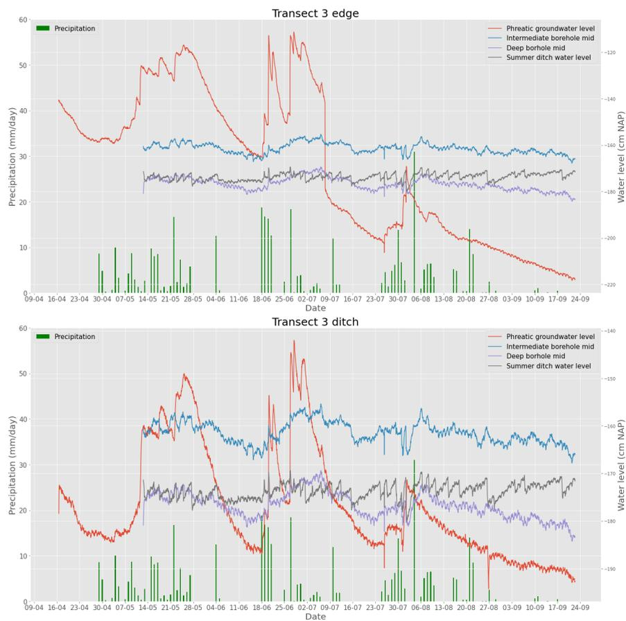
Figure C.6: Pressure monitor data for the boreholes along Transect 3 as well as the deep borehole pressure monitor data between the 16<sup>th</sup> of April and the 23<sup>rd</sup> of September.
