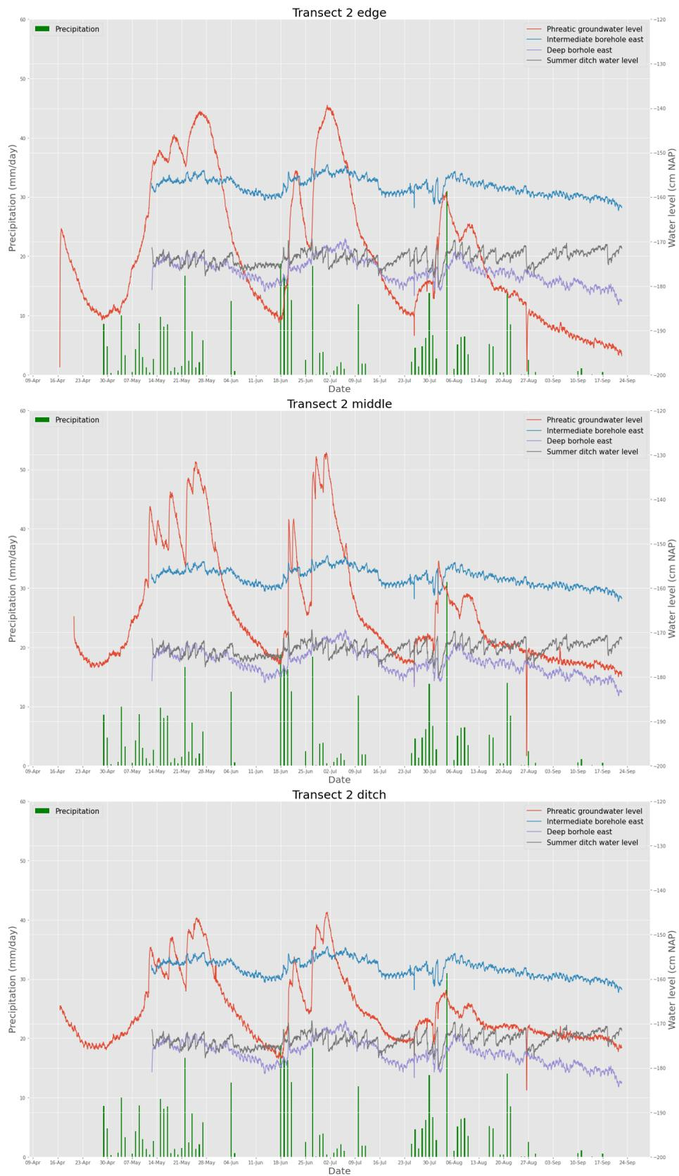
Figure C.5: Pressure monitor data for the boreholes along Transect 2 as well as the deep borehole pressure monitor data between the 16<sup>th</sup> of April and the 23<sup>rd</sup> of September.
