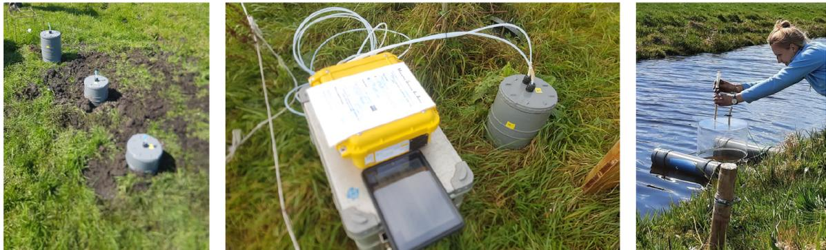
Figure 6.2: From left to right: the three flux chambers placed in different subsurface layers, the MGGGA connected to one of the flux chambers and the floating flux chamber.
