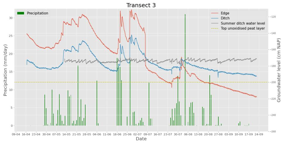
Figure C.3: Pressure monitor data for the boreholes along Transect 3 between the 16<sup>th</sup> of April and the 23<sup>rd</sup> of September.
