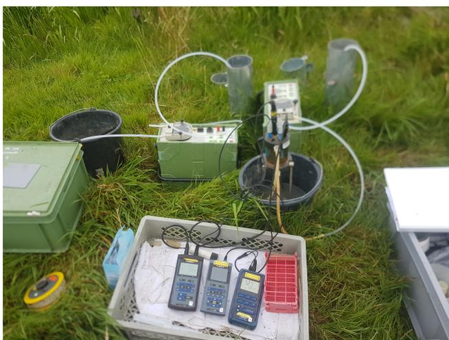
Figure 5.1: Groundwater sampling setup in two deep boreholes. The pump can be seen as well as the three multimeters used to measure pH, EC, temperature, redox potential and DO.
