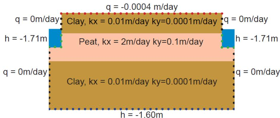
Figure 4.4: Pressure head and specific discharge boundary conditions used in the FlexPDE model as well as the used hydraulic conductivities.
