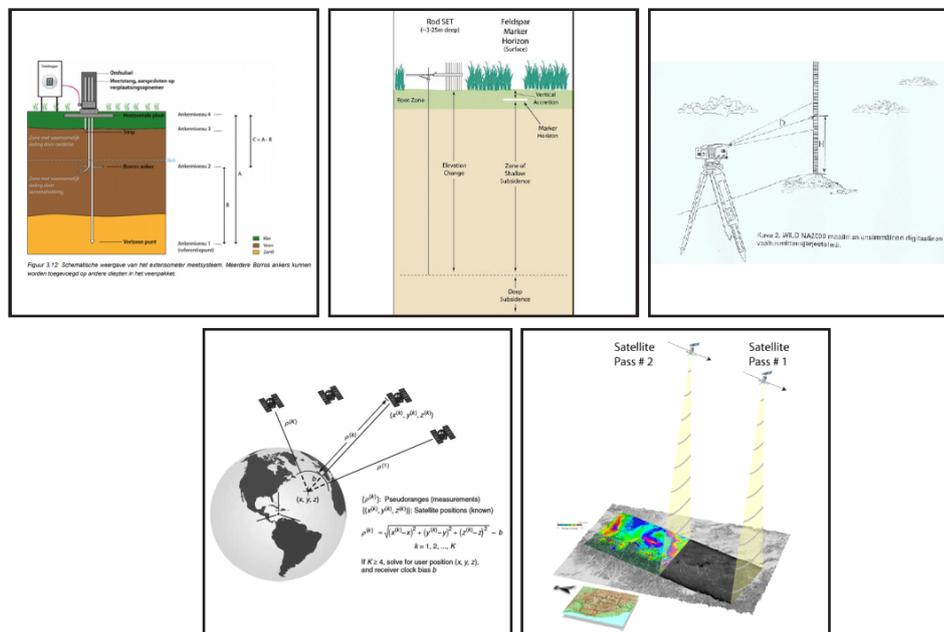
Figure 3.1: Surface elevation measuring techniques (L to R, T to B): extensometer [Asselen et al., 2020], SET [Lynch et al., 2015], Digital leveller [Takalo and Rouhiainen, 2004], GNSS [Fokker et al., 2018] and InSAR [Helz, 2005].
