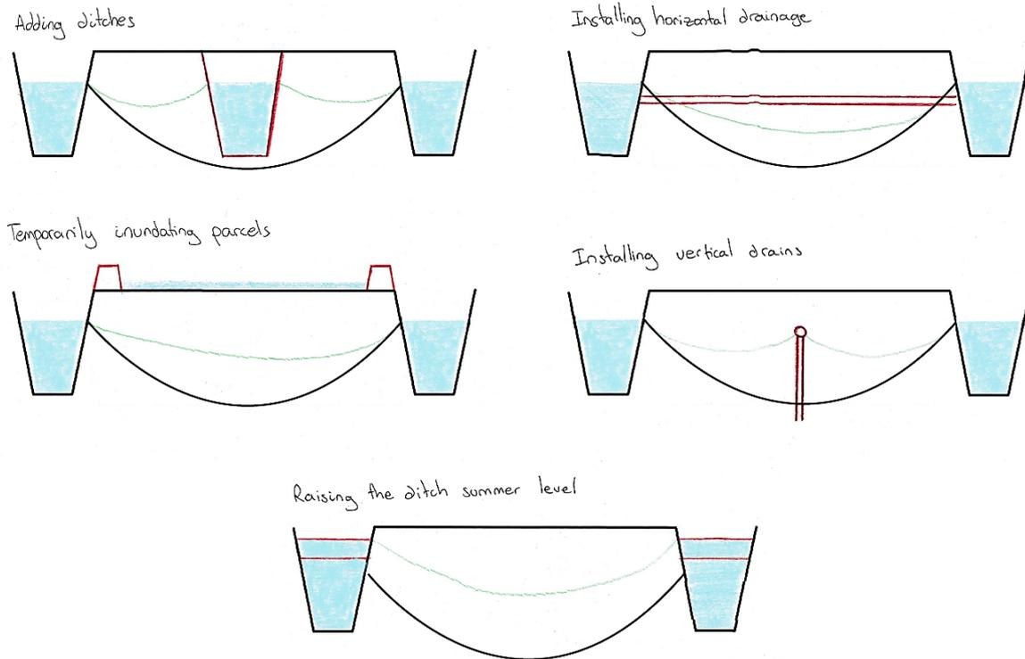
Figure 8.1: Sketch of water management measures examined in this study. The application of the measures are shown in red, and the expected impact on the groundwater levels are shown in green.
