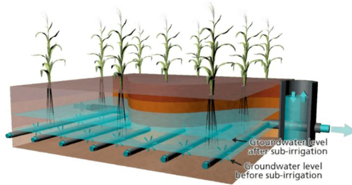
Figure 8.7: Vertical drains illustration. In this study, the vertical drain is connected to the first aquifer from which water is transported up and then across the parcel through a horizontal drain placed in the middle of the parcel, parallel to the ditches [Narain-Ford et al., 2020].
