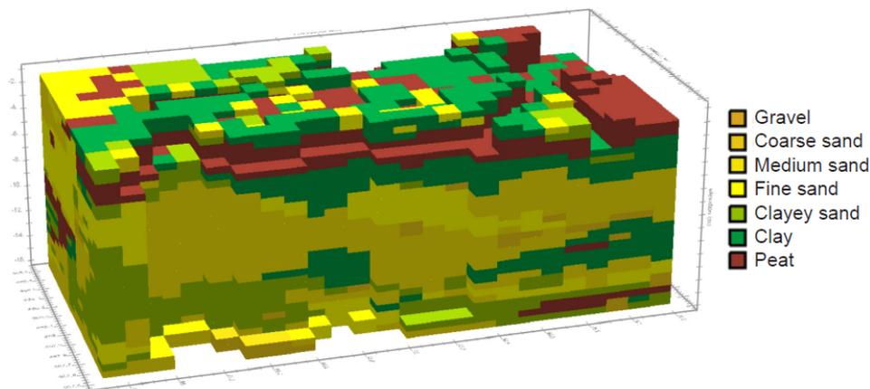
Figure B.2: Subsurface composition gathered from GeoTop data
