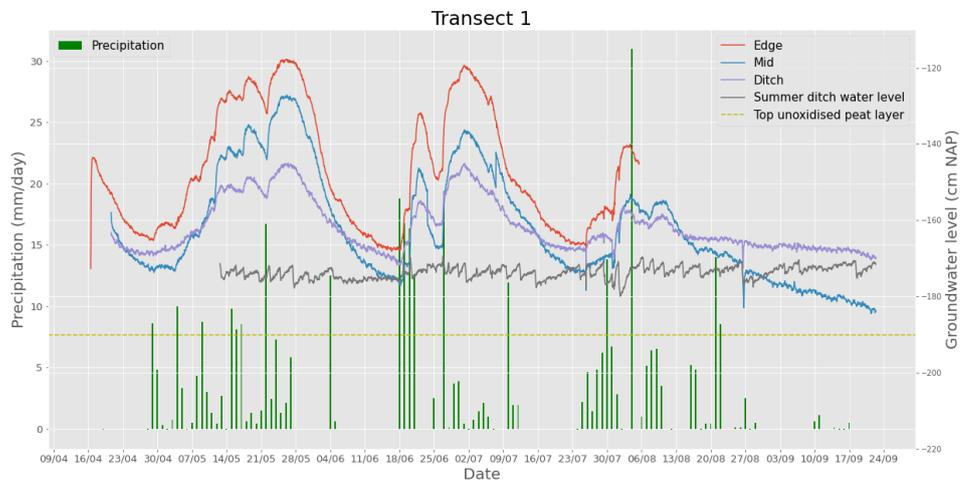
Figure C.1: Pressure monitor data for the boreholes along Transect 1 between the 16<sup>th</sup> of April and the 23<sup>rd</sup> of September.
