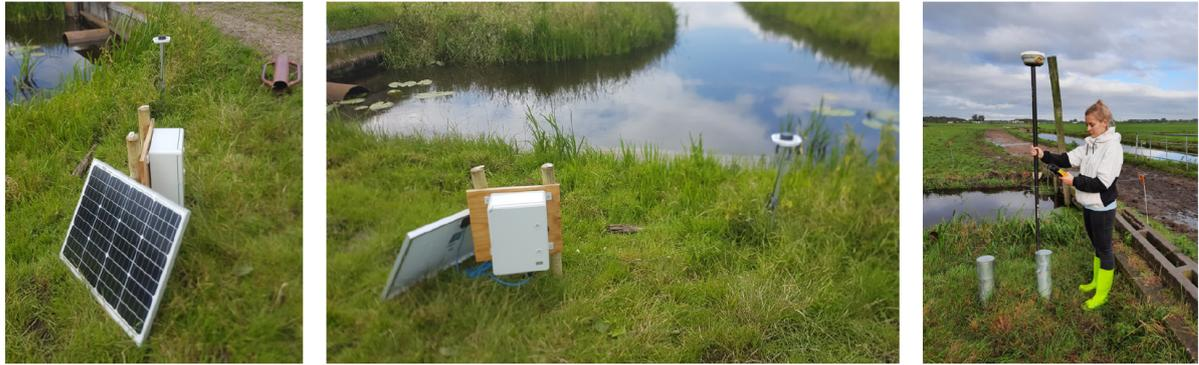
Figure 7.1: Left and center: GNSS station used to measure land surface displacements. The GNSS receiver can be seen on the top of the pole, inserted 30 cm into the ground. In the cabinet, the logger and batteries are stored and the solar panel recharges the batteries. Right: Manual GNSS measurements with the Trimble R8.
