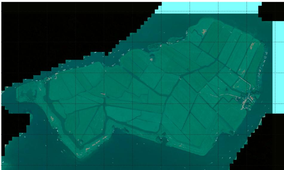
Figure B.3: Model boundary, the blue highlighted region was taken into account for this model. The boezem and the island were set to 1 (active cells) and the black surroundings were set to 0 (inactive cells).
