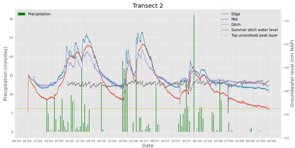
Figure C.2: Pressure monitor data for the boreholes along Transect 2 between the 16<sup>th</sup> of April and the 23<sup>rd</sup> of September.
