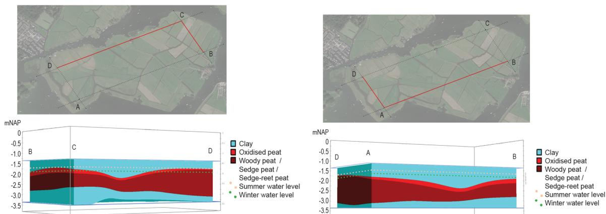
Figure 2.3: Subsurface composition from borehole interpolation of the north eastern part of the polder.
