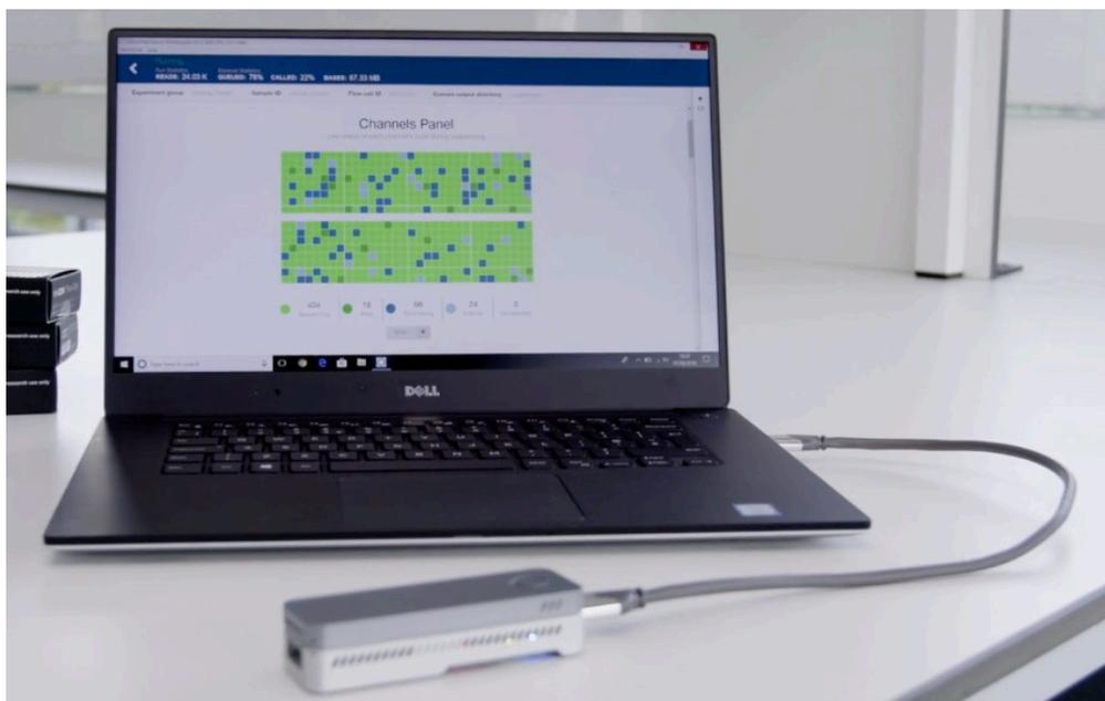
**Figure 1.4 A MinION™ sequencing device plugged in a laptop**
