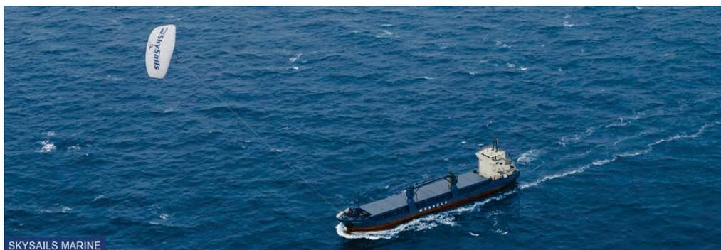
**Figure A.6:** A cargo ship propelled by a kite from the company SkySails.
