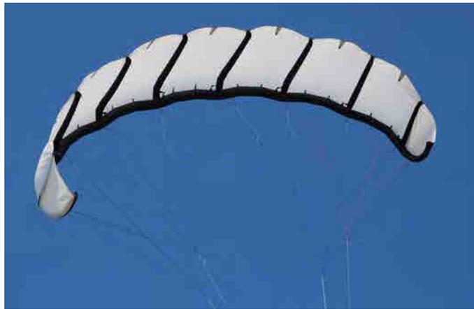
**Figure B.6:** The Genetrix 25m<sup>2</sup> contains a bulging LE to preserve a more constant profile over the wing.
