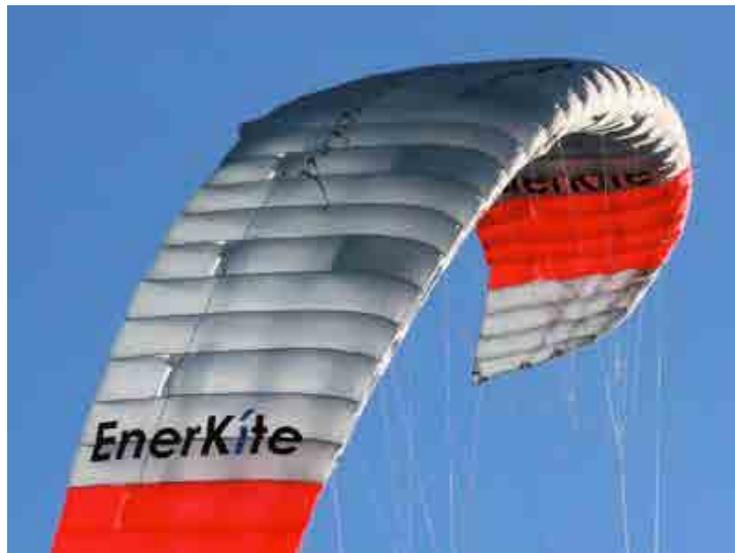
**Figure A.9:** The 21m<sup>2</sup> high performance foil kite used by EnerKite (EnerKite, 2012).
