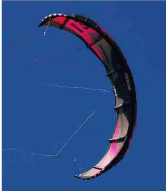
**Figure B.5:** An additional kite was acquired to verify whether a lower camber factor and higher aspect ratio positively influenced performance. This kite is a  $14m^2$  Genetrix Hydra.
