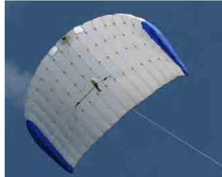
**Figure A.11:** The foil kite used by SkySails Power with two large air inlets near the center (SkySails, 2012b).
