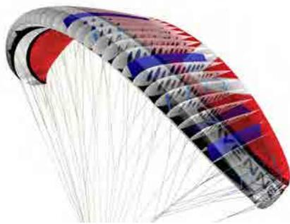
**Figure A.1:** See through impression of the construction of a ram air wing (Skywalk, 2008).
