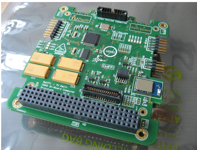
Figure 2.14: Example of a CubeSat on-board computer (TU Delft) with PC/104 connector.
