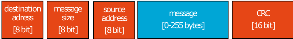
Figure 3.22: Proposed packet definition for RS-485.
