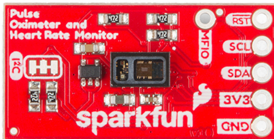
Figure 3-13: Pulse Oximeter and Heart Rate Monitor (MAX30101) from Maxim Integrated™: breakout board from SparkFun™(left) and system diagram (right) [11]
