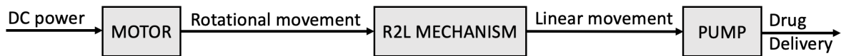
Figure 6-1: A rough overview of the mechanical components of the novel drug delivery pump
