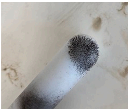
Fig. 12. Material of the black layer on a magnet, showing that the material consists of powders with magnetic properties.
