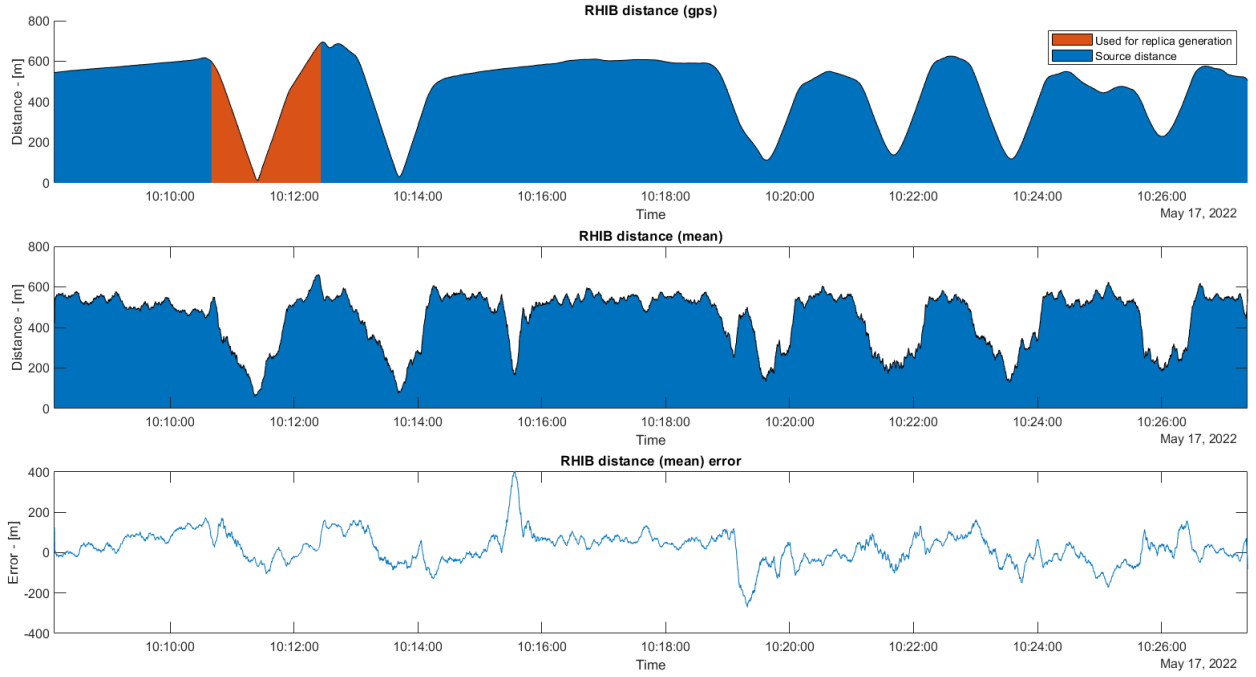
(b) Minimisation ranging - single-pass - moving average filter
