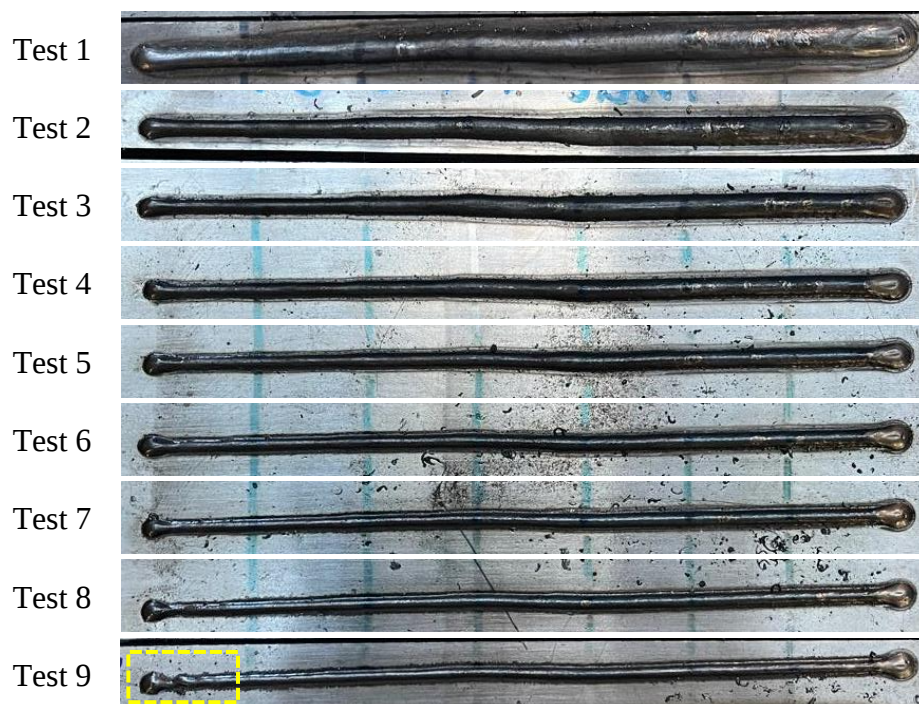
Figure 4.2 Bead appearance from ramping test in SAWP mode
