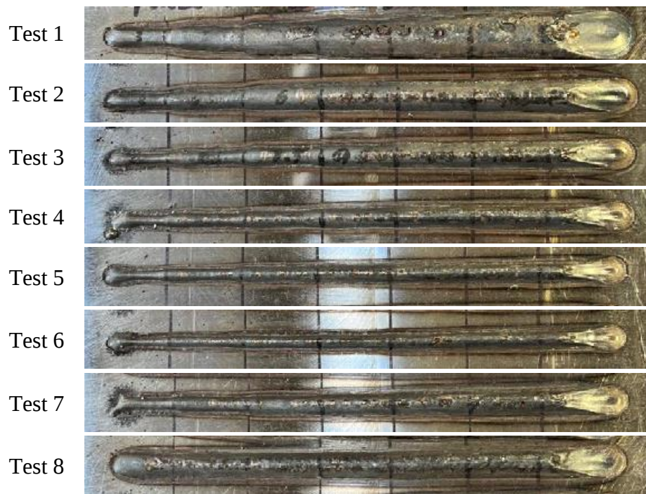
Figure 4.1 Bead appearance from ramping test in pulsed mode
