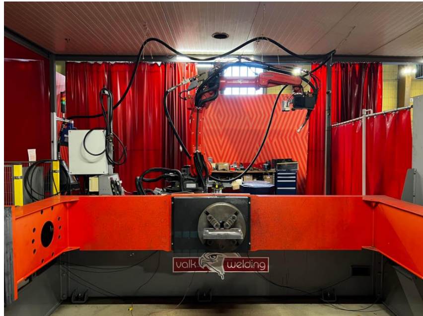
Figure 3.2 Panasonic TM 2000 WGIII robot setup for printing experiment
