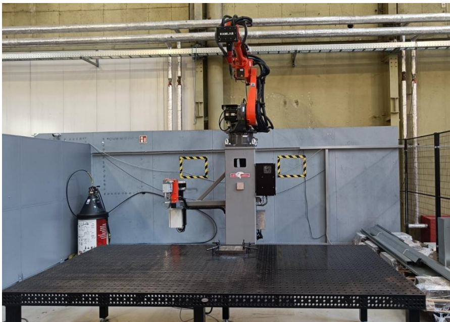
Figure 3.1 Panasonic WGHIII-E-HH020L robot setup for printing experiments
