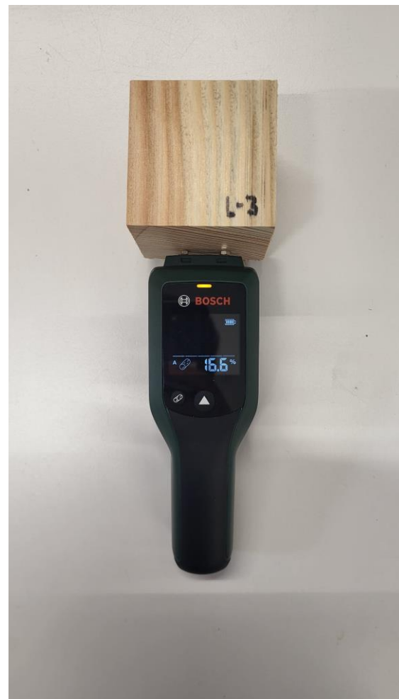
Figure 34 Moisture sensor monitoring process of Larch wood piece on initial experimentation estage.
