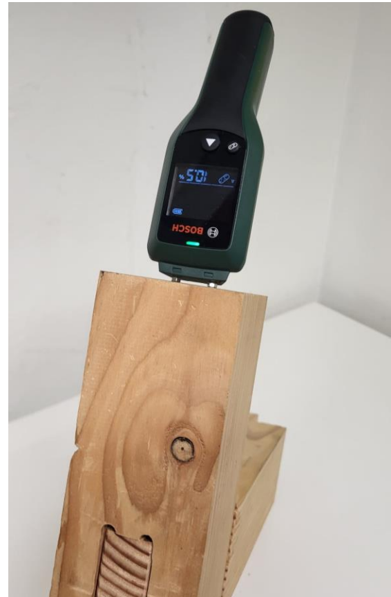
Figure 118 Cross- Half Lap Moisture Content
