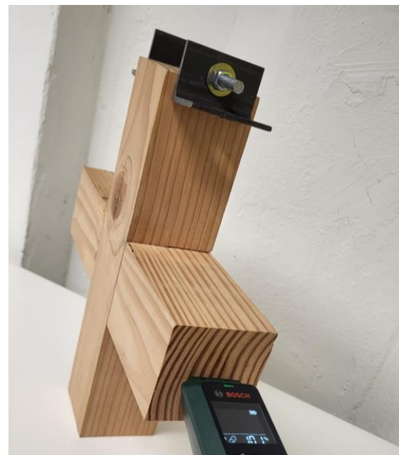
Figure 118 Cross- Half Lap Moisture Content
