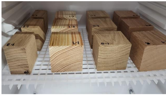
Figure 36 samples placement in fridge chamber ( Elm, Larch, Oak, Meranti )
