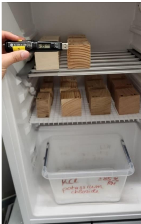
Figure 38 Moisture sensor, and experiment set up
