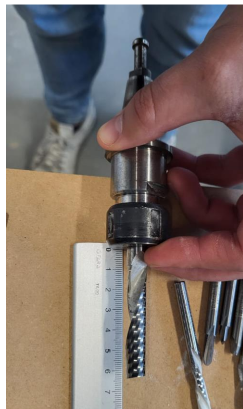
Figure 63 mill and holder collector dimensions
