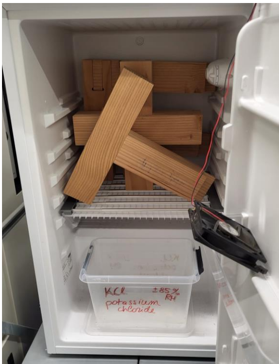
Figure 116 Moisture Induce Wood Connections Testing Set Up
