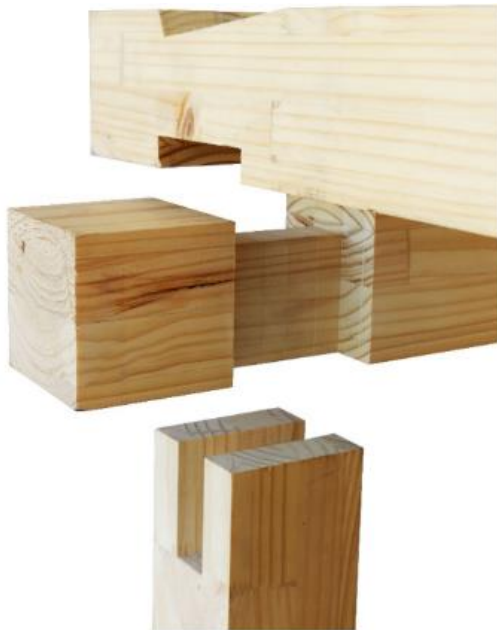
Figure 56 - knot compose of T-bridle jointed post and top plate with notched tie beam, and oblique mortise. Source: (Bohme et al., 2017)
