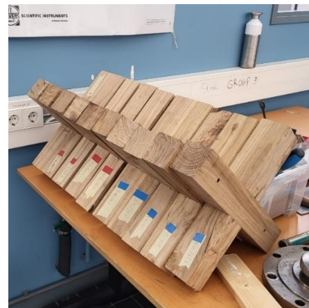
Figure 126 Cross Half Lap specimens for Tensile Test
