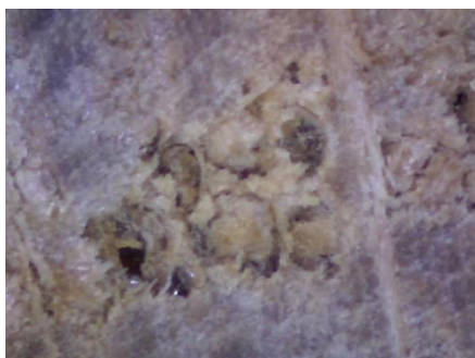
Oak O-5 Tangential and Radial structure x 200
