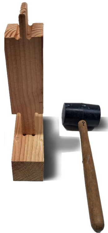
Figure 81 Assembly method - Mortise and Tenon
