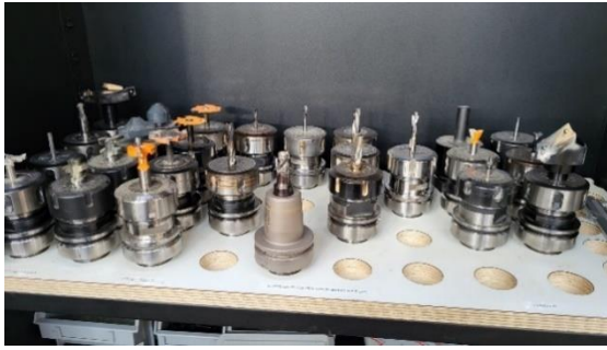
Figure 61 Mills use in TNM production process.
