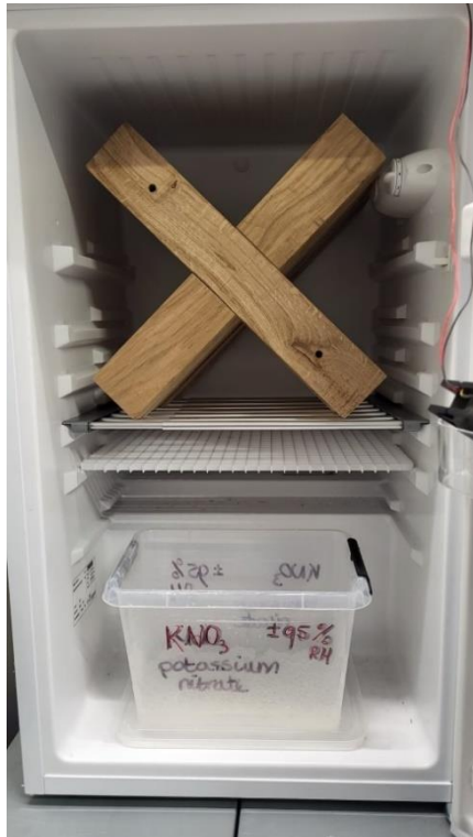
Figure 125 Climate chamber Cross- Half Lap
