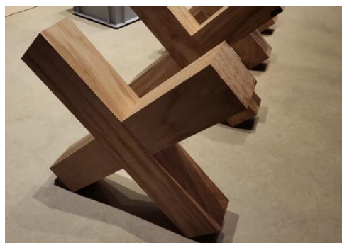
Figure 104 Cross- Half Lap Prototype, Koln, Germany
