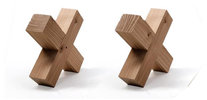
Figure 89 Cross-Half-lap joint, parallel and perpendicular to the grain
