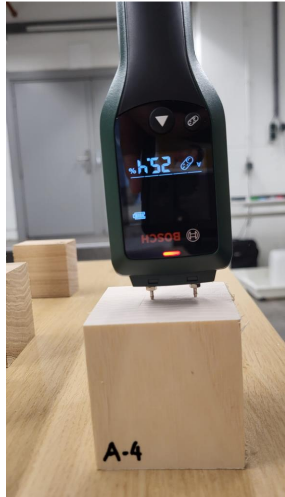
Figure 35 Ash moisture sensore value beginig of experiment
