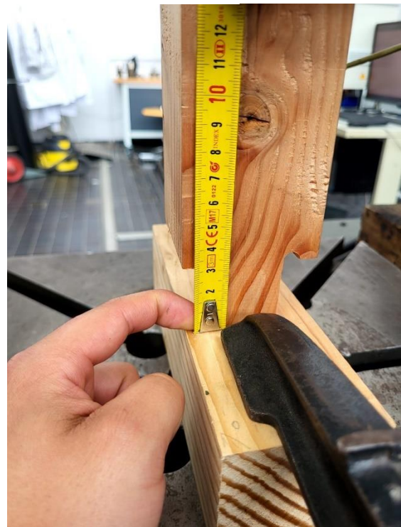
Figure 122 Mortise and tenon maximum displacement
