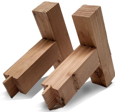
Figure 82 Mortise and tenon prototype - Douglas Pine
