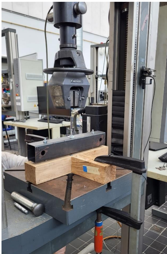
Figure 127 Tensile test of Cross Half Lap Joints
