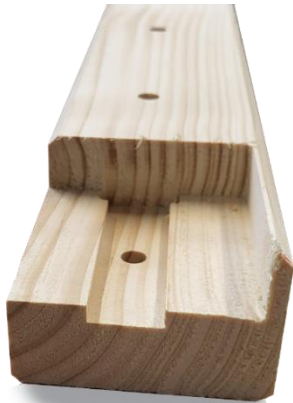
Figure 72 First CNC Sample of the research - starting point mistake.
