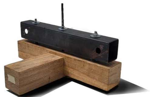
Figure 128 Cross - Half Lap Set Up pin connection
