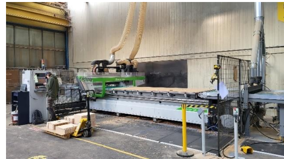
Figure 60 CNC Machine for big formats 1220 mm x 3000mm The New Makers
