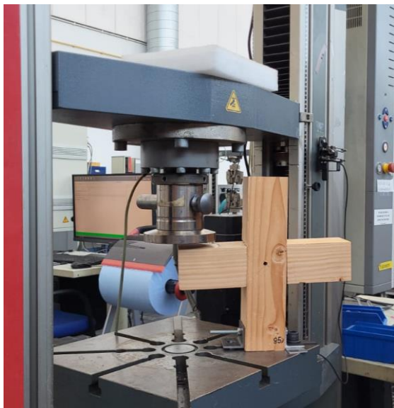
Figure 123 Cross -Half Lap joint Under Compression
