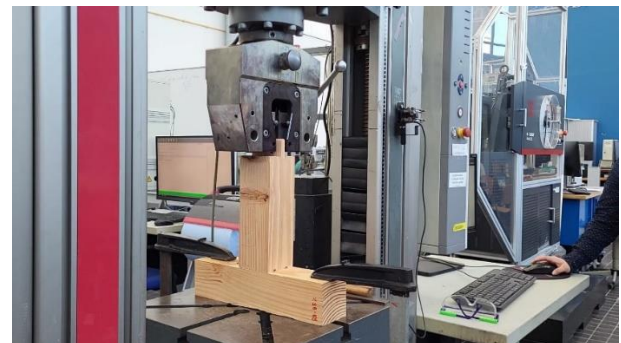
Figure 120 Tension Test capacity of Mortise and Tenon Joints
