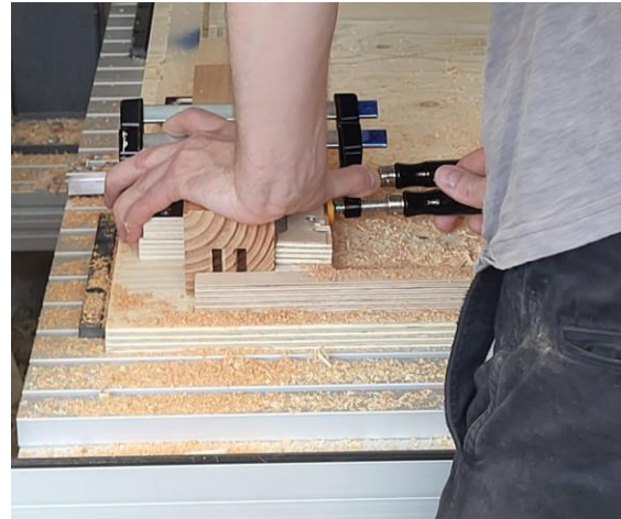
Figure 78 First material mold anchorage system
