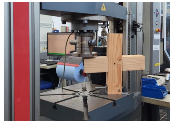
Figure 148 Compression test Laboratory of Mechanics-3ME faculty TU Delft University
