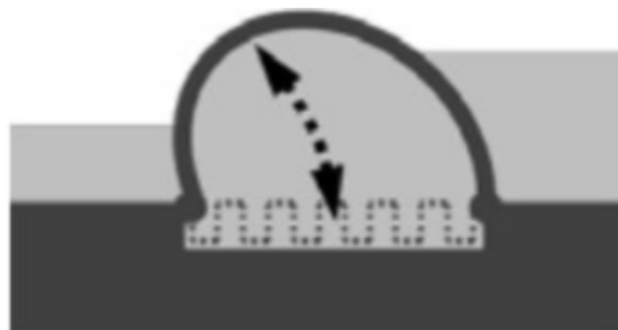
Figure L.3: Cross-section of an inflatable gate (Mooyaart & Jonkman, 2017).
