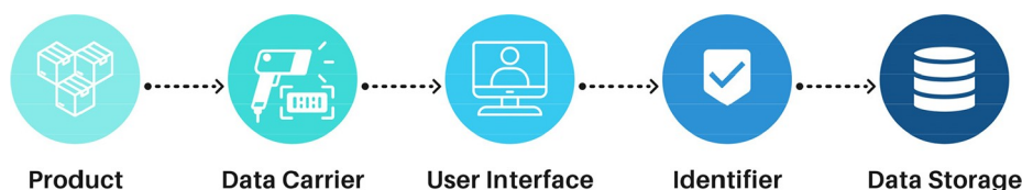
Figure 1. Proposed track and trace technology stack connecting the physical construction product to its digital representation
