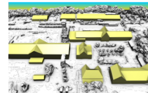
Figure 1. Given a MVS mesh, our approach provides simple, topological valid building models that can be used in the context of urban scene reconstruction.
