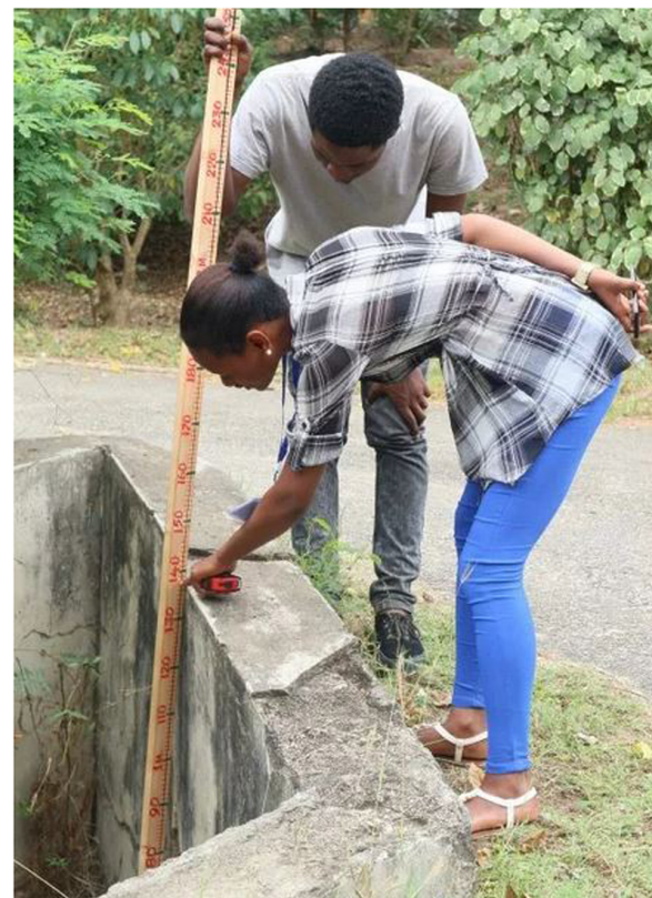
FIGURE 3 | Ramani Huria drainage mappers, recording drainage features with a wooden ruler and smartphone. Written informed consent was obtained from the participants for the publication of any potentially identifiable images or data included in this article. Photo Chris Morgan/World Bank.
