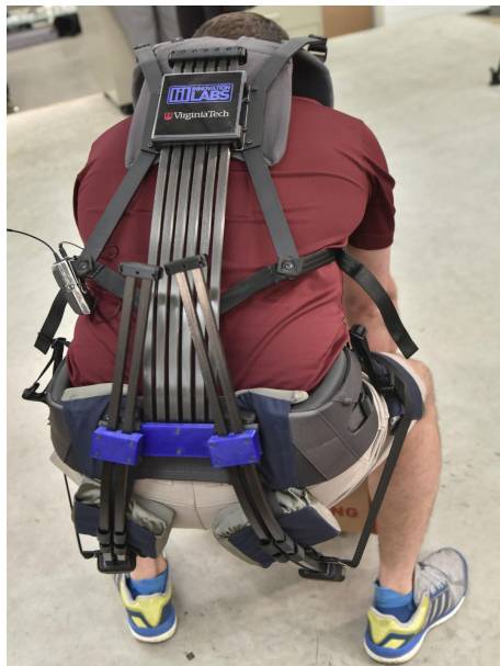
Figure 3.2: Virginia Tech Lowe's Exoskeleton in lifting configuration [14].
