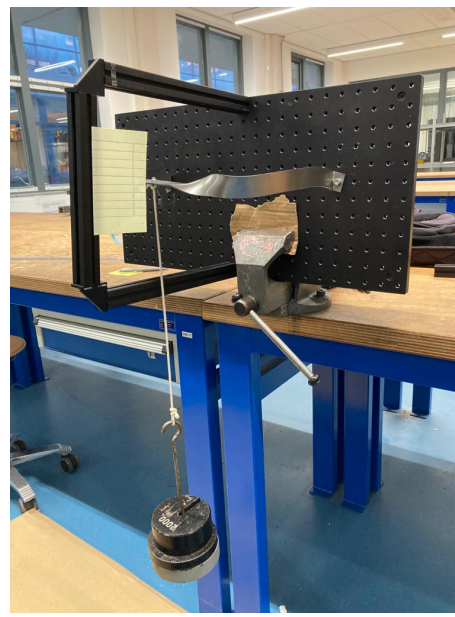
Figure A.20: Setup forward bending experiment
