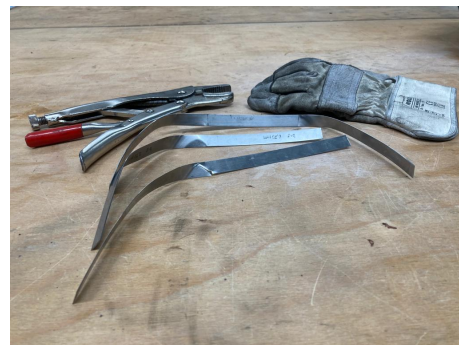
Figure A.18: Twisting spring steel strip of thickness 0.5mm, 0.75mm and 1.0mm. The results show that the strip with 0.5mm thickness broke after a twist was applied. The used pliers and glove for this experiment are also shown.
