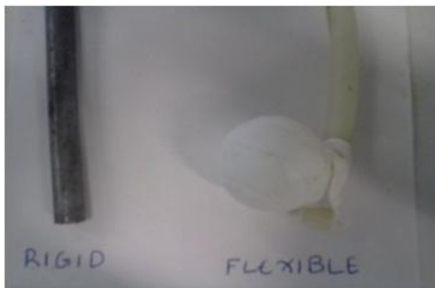
Figure 10 Improvised floating decanter
