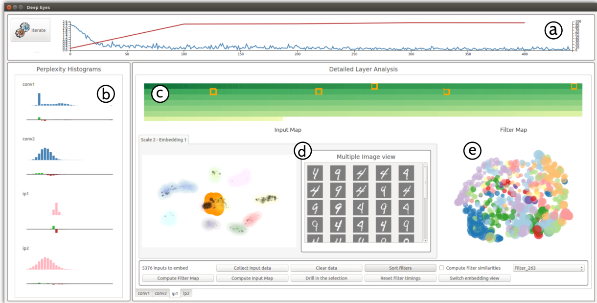
Fig. 1. DeepEyes is a Progressive Visual Analytics system for the analysis of deep neural networks during training. The overview on the training is given by the commonly used loss- and accuracy-curves (a) and the Perplexity Histograms (b) a novel visualization that allows the detection of stable layers. A detailed analysis per layer is performed in three tightly linked visualizations. Degenerated filters are detected in the Activation Heatmap (c), and filter activations are visualized on the Input Map (d). Finally, in the Filter Map (e), relationships among the filters in a layer are visualized.
