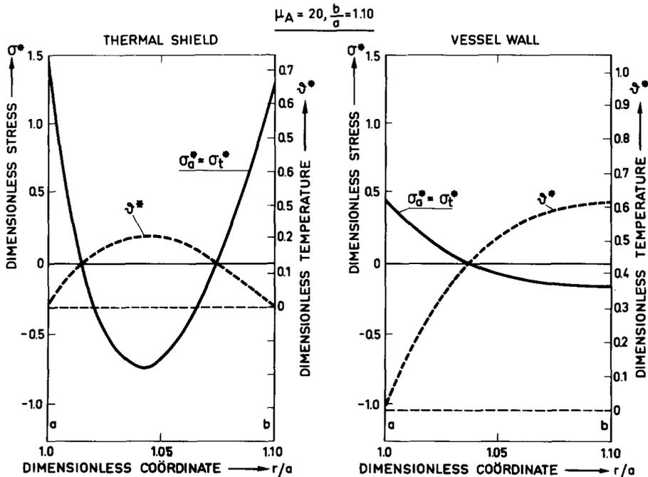
Fig. 10. Temperature and stress distribution in vessel wall and thermal shield due to  $\gamma$ -heating, ref. [B.29].
