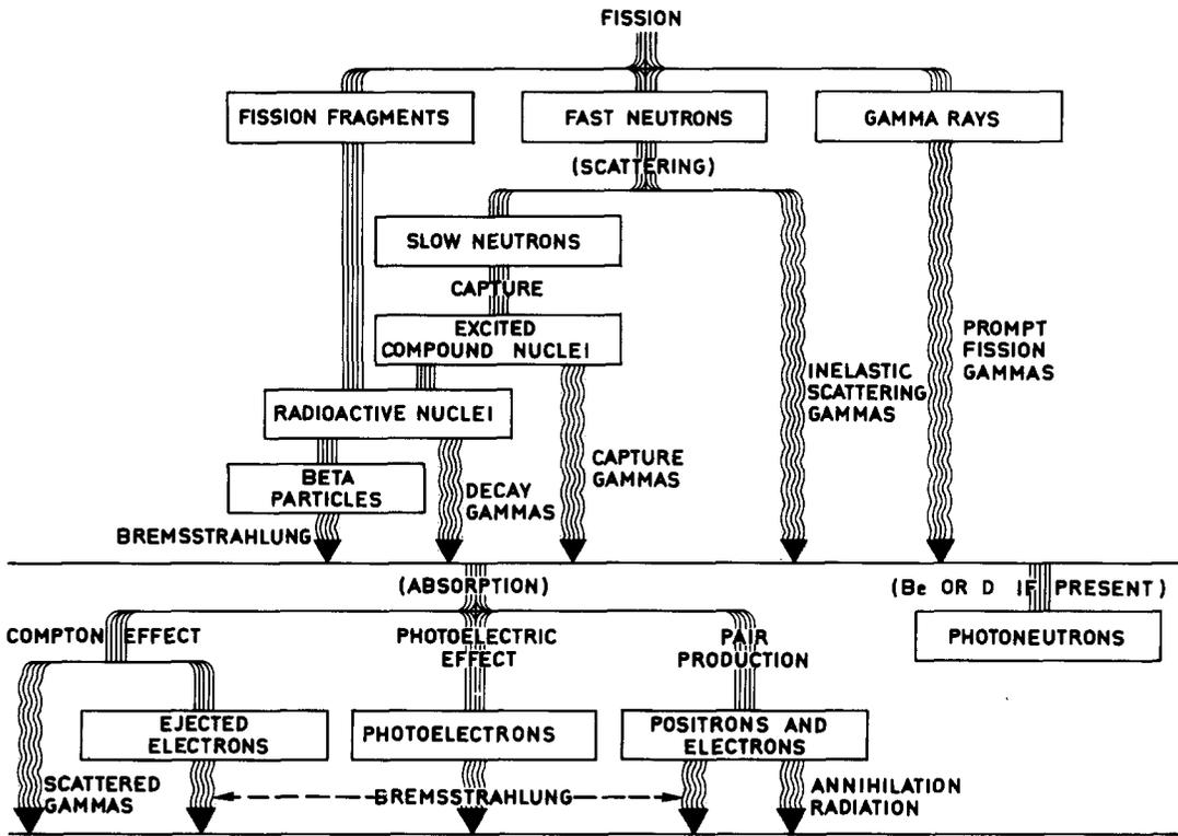
Fig. 9. Types of radiation from a nuclear reactor core, Ref. [B.27].
