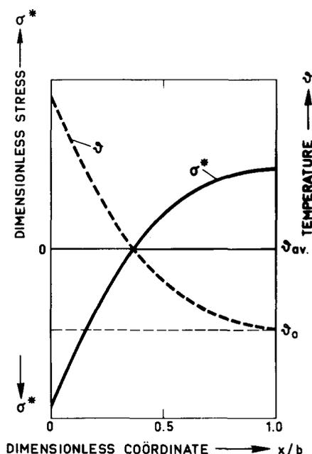
Fig. 7. Wall temperature stress distribution for quasi-steady state heating.
