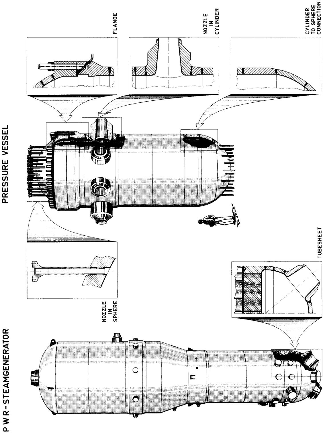
Fig. 4. Schematization of p.v. components into basic elements.
