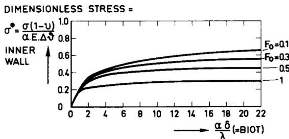
Fig. 8. Maximum stress for transient heating, ref. [B.25].
