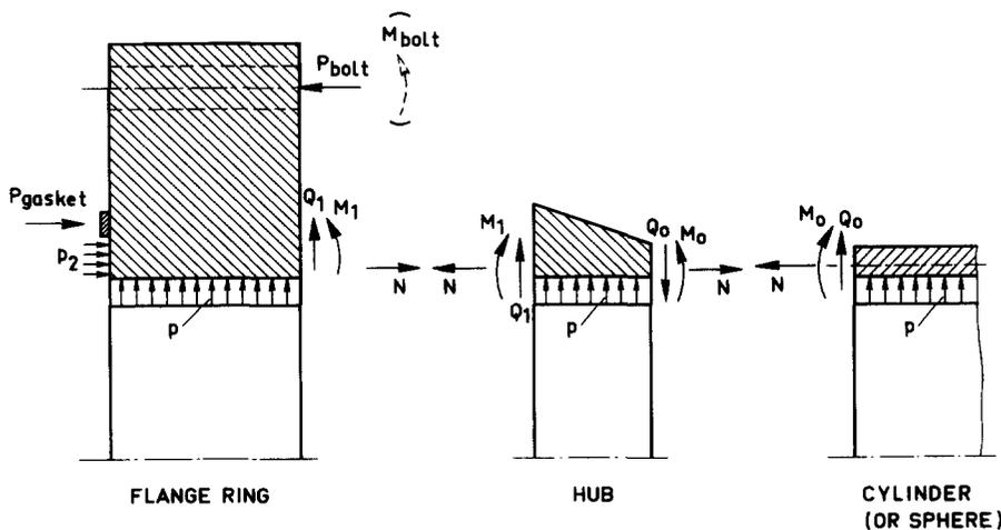
Fig. 11. Schematization of flange.
