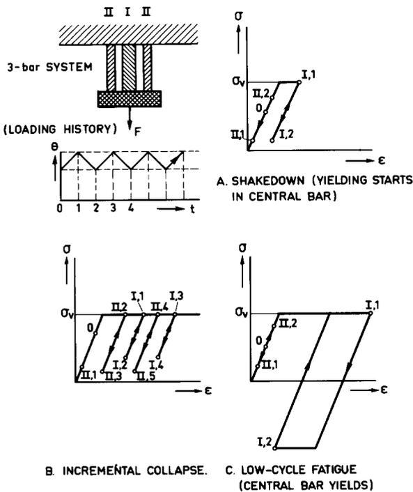
Fig. 1. Failure under alternating load, ref. [A.5].
