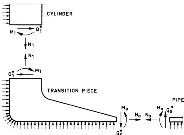
Fig. 12. Schematization of nozzle.
