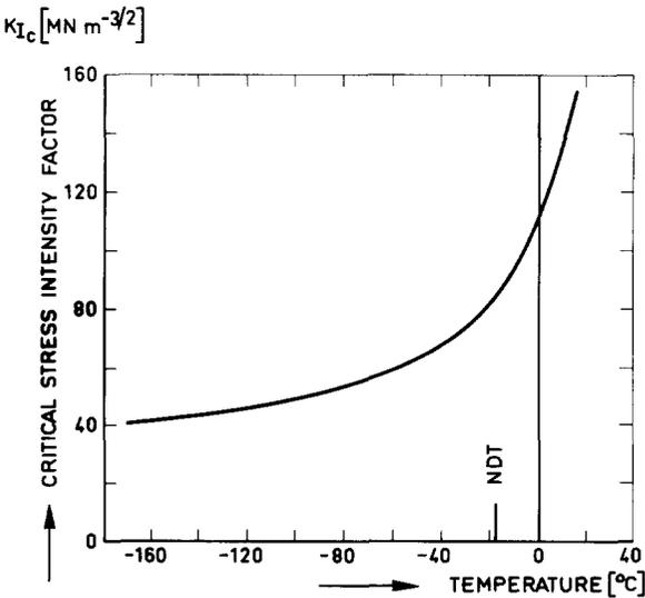
Fig. 2. Fracture:  $K_{Ic}$  as  $f(\theta)$  (ref. as for fig. 3).
