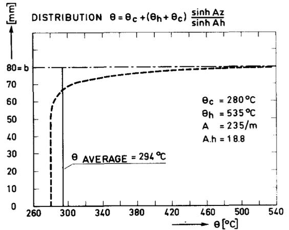
Fig. 15. Temperature distribution in tubesheet.
