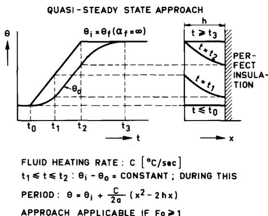
Fig. 6. Fluid temperature ramp change: quasi-steady state approach.
