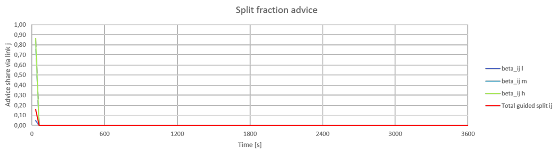
Figure 5.8: Split fraction advice towards link j when optimising accident risk with a compliance rate of 0.4 in the school route case
