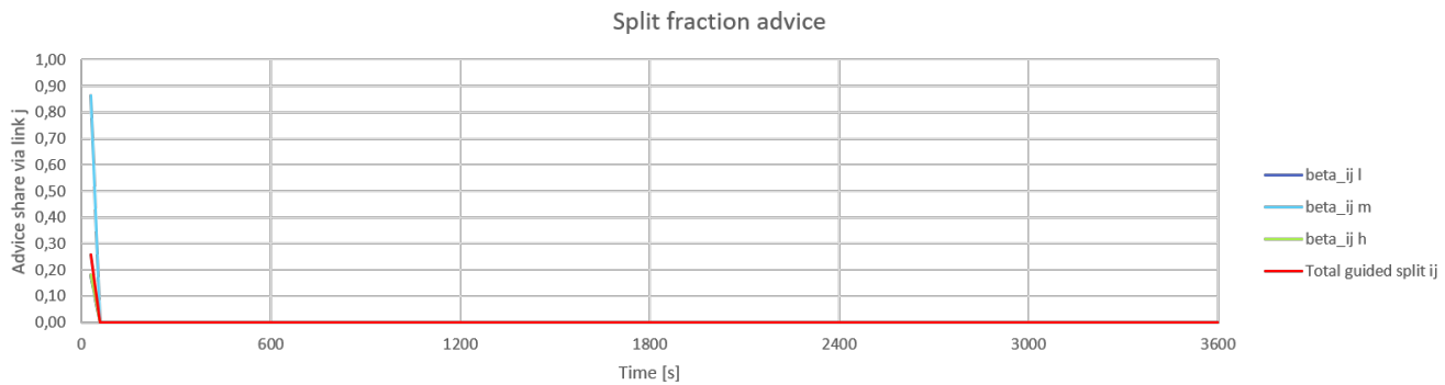
Figure D.17: Split fraction advice towards link j when optimising air quality with a compliance rate of 1, with schoolchildren given a double weight
