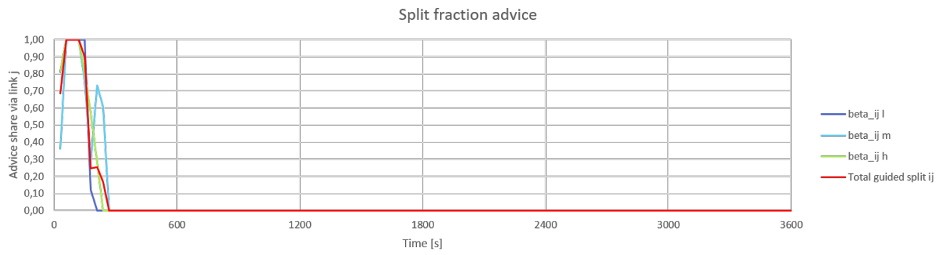
Figure D.36: Split fraction advice towards link j when optimising noise with a compliance rate of 0.1
