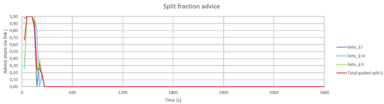
Figure D.28: Split fraction advice towards link j when optimising travel time with a compliance rate of 0.1
