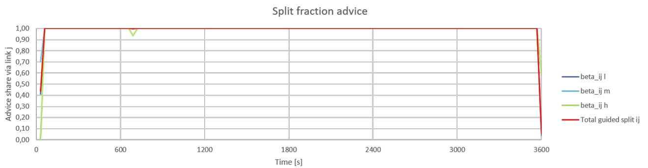
Figure D.1: Split fraction advice towards link j when optimising travel time with a compliance rate of 1
