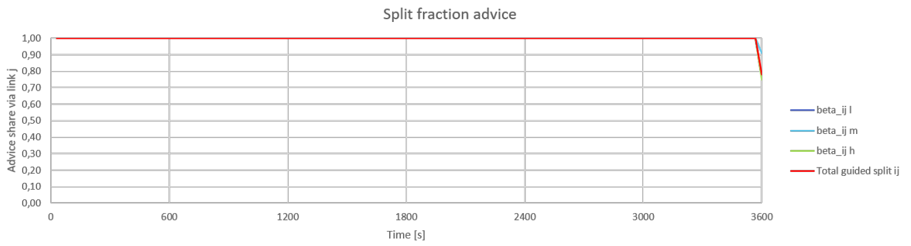
Figure D.12: Split fraction advice towards link j when optimising noise with a compliance rate of 0.1
