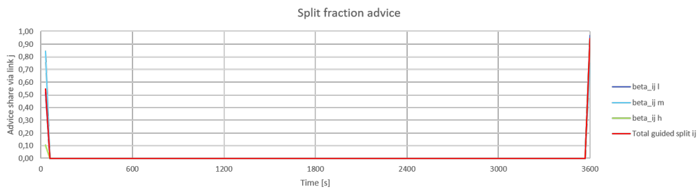
Figure 5.6: Split fraction advice towards link j when optimising noise with a compliance rate of 0.4 in the school route case
