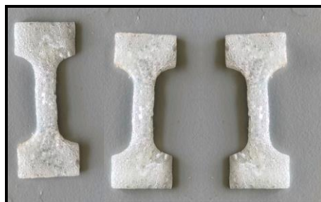
Figure 42: Sample: Tensile testing of recovered resin
