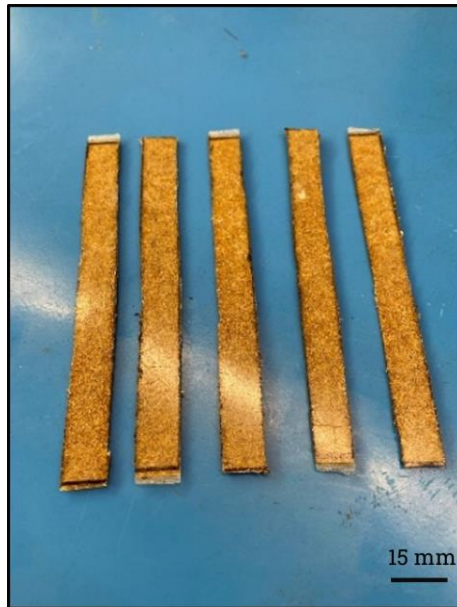
Figure 31: Samples- Tensile testing of composite
