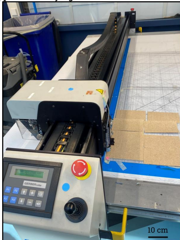
Figure 19: Gerber Cutting Machine cutting bamboo fiber mat
