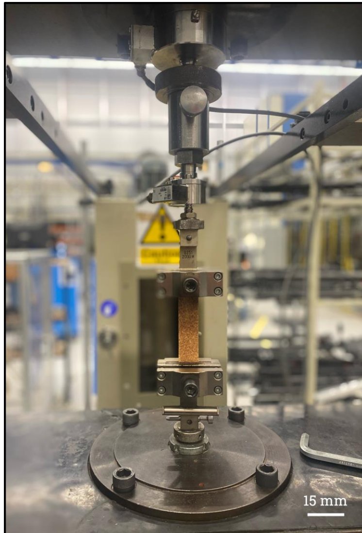
Figure 30: : Test setup- Tensile testing of composite
