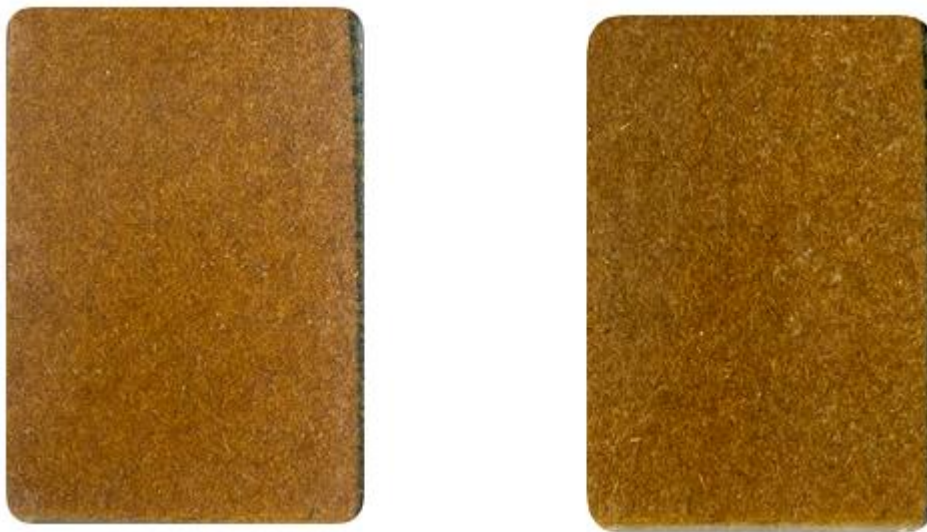
Figure 46: Composite samples- before water absorption test; after water absorption test
