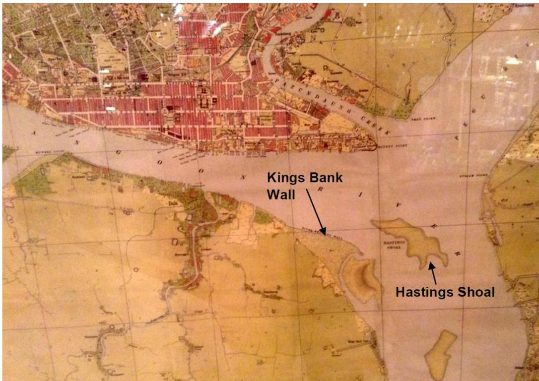
Figure 2.17: Yangon Estuary 1930 at the estuary split. Construction of the Kings Bank Wall. The goal of the wall was to erode the Hastings Shoal.
