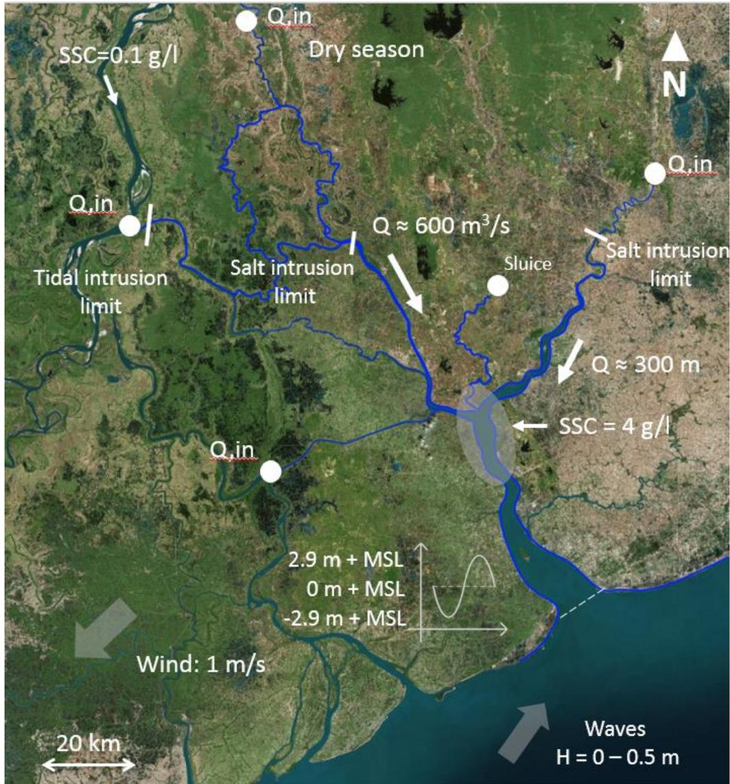
Figure 2.21: Stage 1 conceptual model, dry season.  $Q_{in}$  is the symbol for the locations where water enters the system.  $Q$  is the average discharge.  $SSC$  is the measured suspended sediment concentration within the oval.  $H$  is the wave height.
