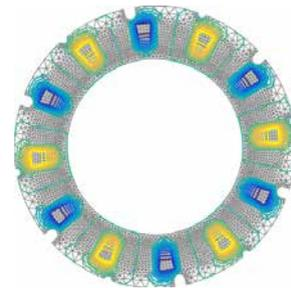
The 2<sup>nd</sup> MTA of the stator for the ACB method
