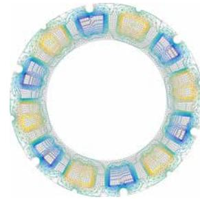
The 13<sup>th</sup> fixed interface mode of the stator for the ACB method
