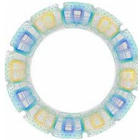
The 12<sup>th</sup> fixed interface mode of the stator for the ACB method
