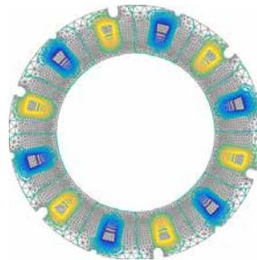
The 1<sup>st</sup> MTA of the stator for the ACB method
