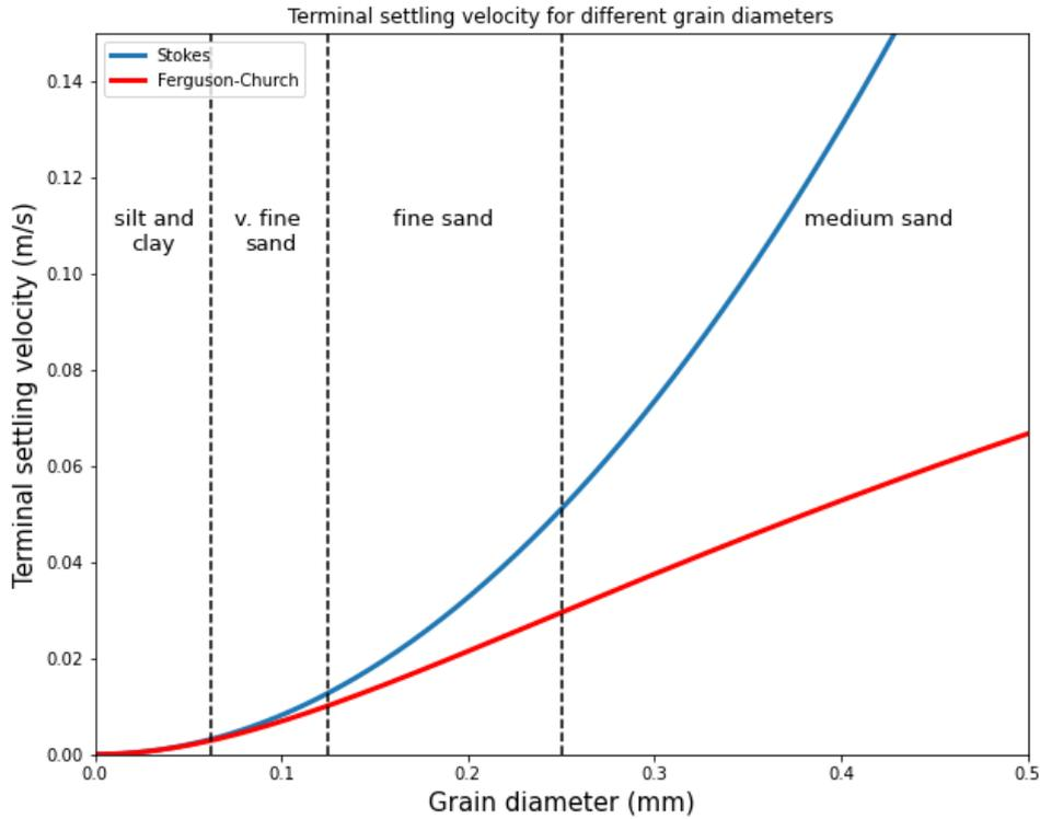
Figure 3.1: Settling velocity depending on grain size and calculation method
