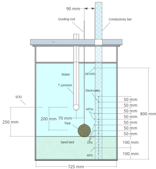
Figure 5.1: Experimental set-up with the location of the measurement devices (after Yang (2020))
