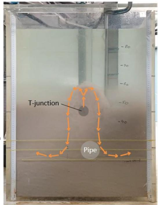
Figure 5.2: Upward discharge from T-junction during the experiments of Eikhout (2020)
