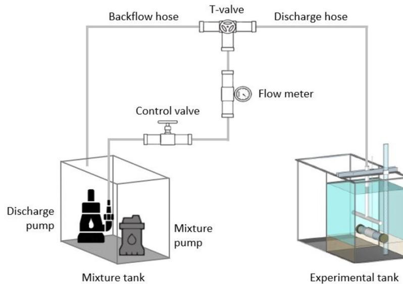
Figure 4.5: Laboratory set-up (after Eikhout (2021))
