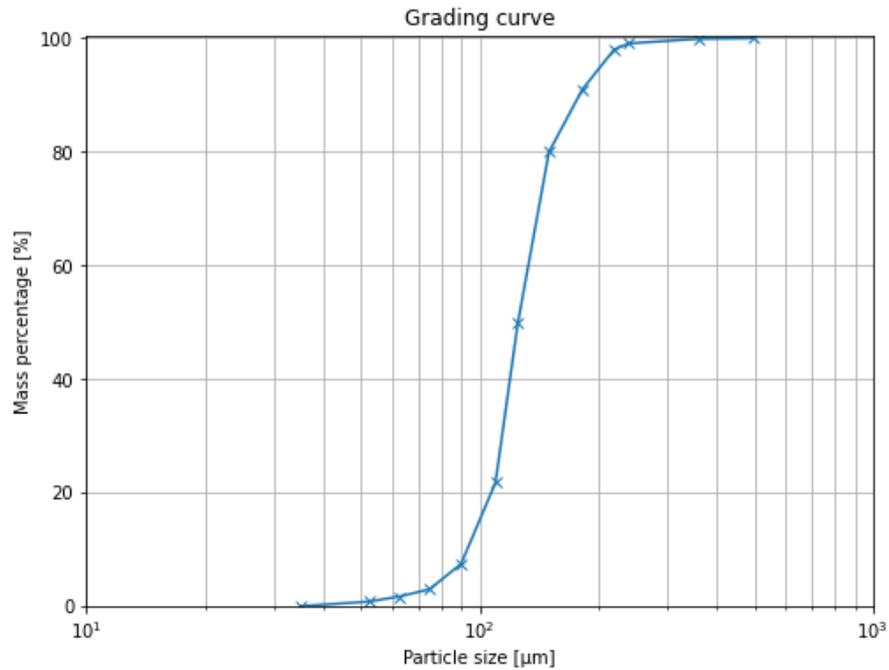
Figure 5.8: Grainsize distribution Geba Weiss sand used for experimental modelling (after Yang (2020))
