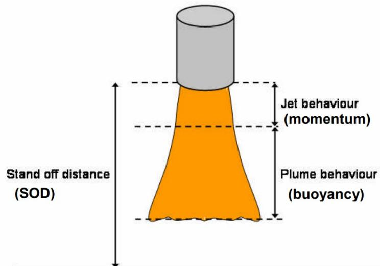
Figure 2.3: Graphical illustration of the jet characteristics (after de Nijs et al., 2009)
