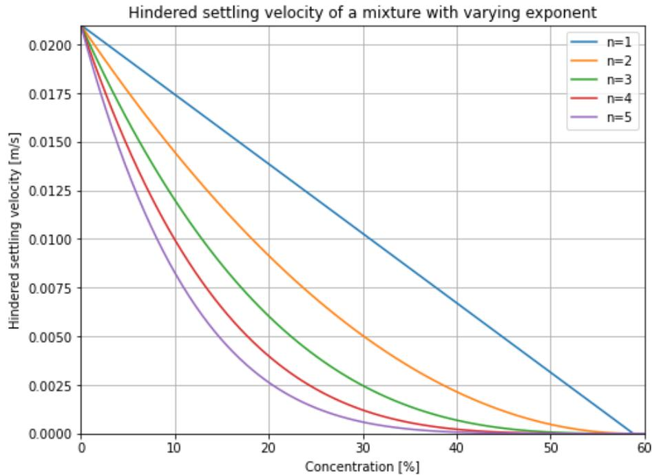
Figure 3.4: Settling velocity of a suspension with different concentrations.
