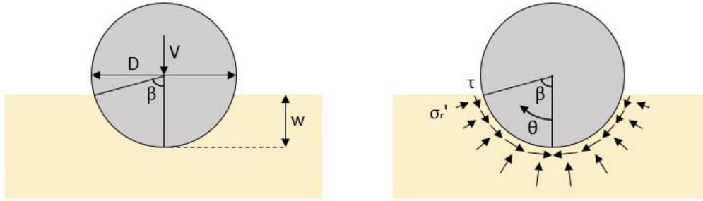
Figure 2.5: Schematisation of the pipe-soil contact stresses (after Eikhout, 2021)
