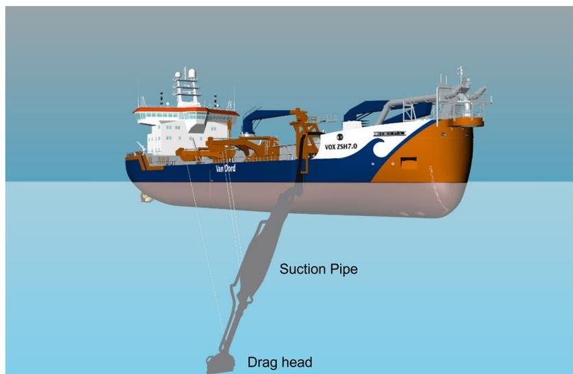
Figure 2.1: TSHD from Van Oord and its primary components
