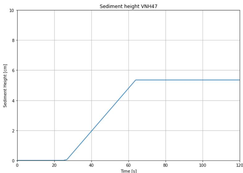
Figure 5.16: Height new formed sand layer over time (Test VNH47)
