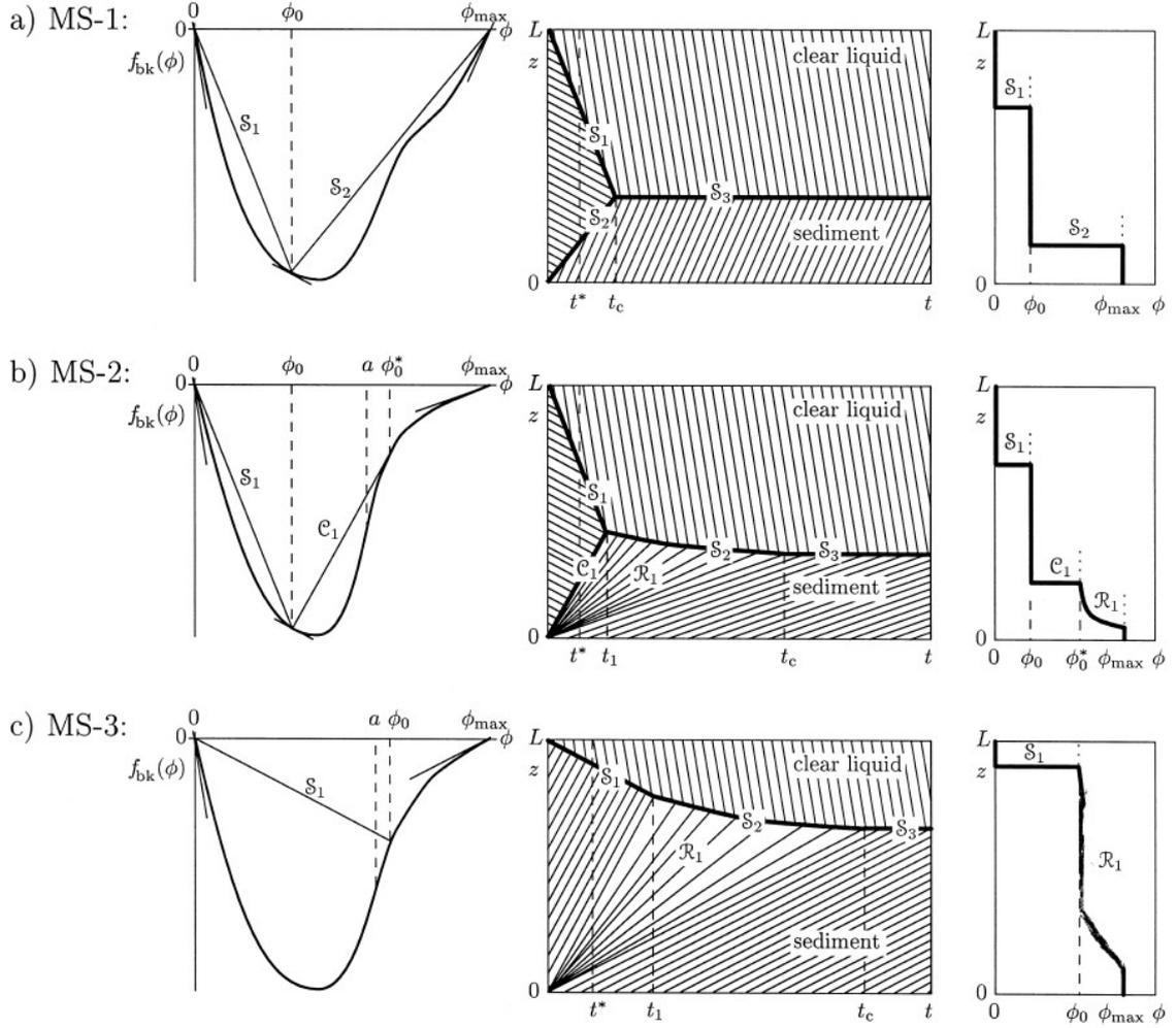
Figure 3.2: Modes of sedimentation MS-1 to MS-3. From the left to the right, the flux plot, the settling plot showing characteristics and shock lines, and a representative concentration profile at a certain time (after Bürger and Tory, 2000).
