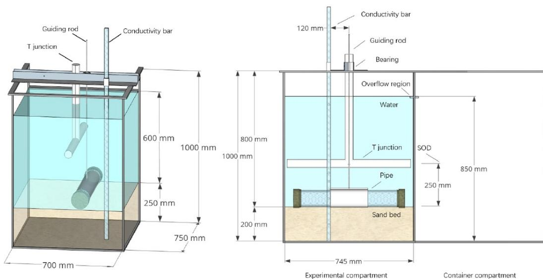
Figure 4.6: Set-up experimental tank (after Yang (2020))
