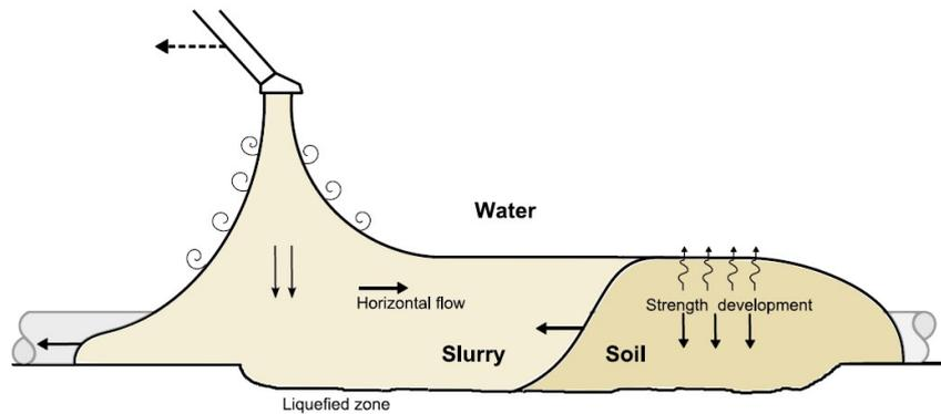
Figure 2.2: Schematic illustration of the backfilling along the pipe. The vessel in this illustration is moving from right to left (after Biemans, 2012)
