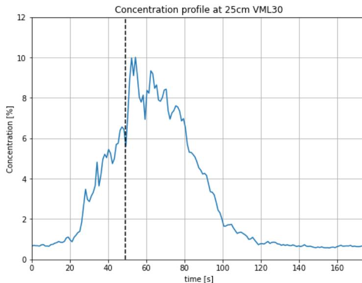
Figure 5.3: Concentration profile at height of the centre of T-junction test VML30
