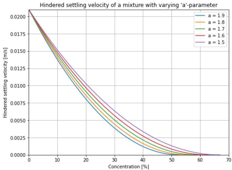
Figure 3.5: Settling velocity depending  $\alpha$ - parameter. Analysis based on the formula:  $v(c) = 0.021 * (1 - \alpha * c)^2$
