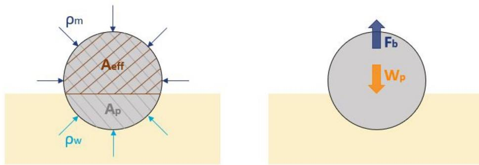
Figure 2.4: Schematic drawing of a one-dimensional section of the pipeline, which is partially embedded and fully surrounded by the sand-water mixture above the sedimentation front (after Eikhout, 2021)
