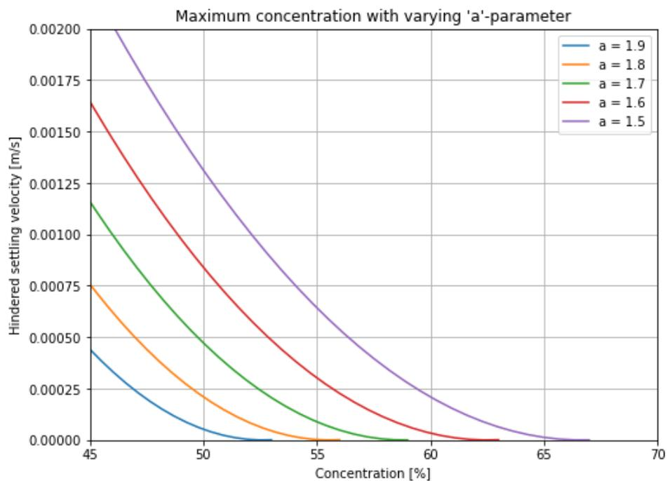
Figure 3.6: Maximum concentration varying with the  $\alpha$ -parameter. Analysis based on the formula:  $v(c) = 0.021 * (1 - \alpha * c)^2$
