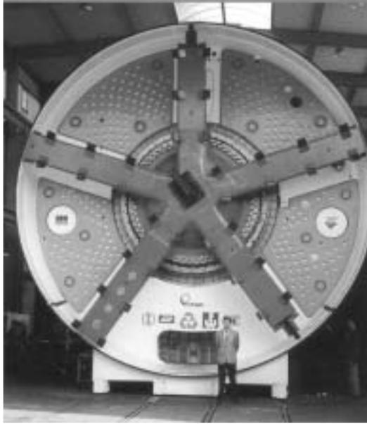
Figure 2.55: Front view of Second Heinenoord TBM
