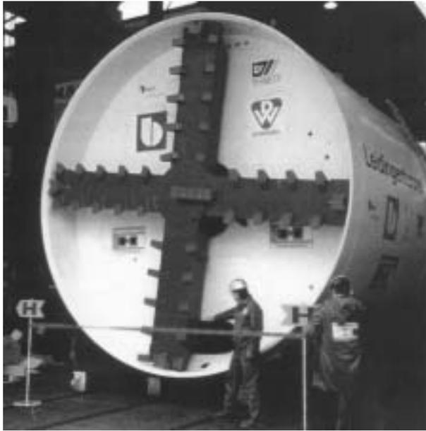
Figure 2.66: Botlek Utility Tunnel TBM
