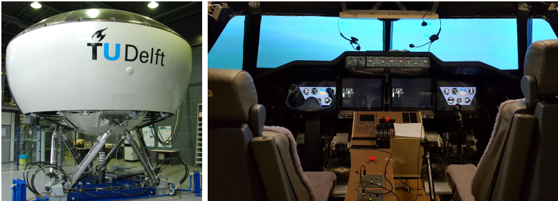
Figure 6.14: SIMONA Research Simulator. The basic instrument panel and the outside view are visible, the navigation display has been placed on the screen to the left of the right-hand instrument panel.
